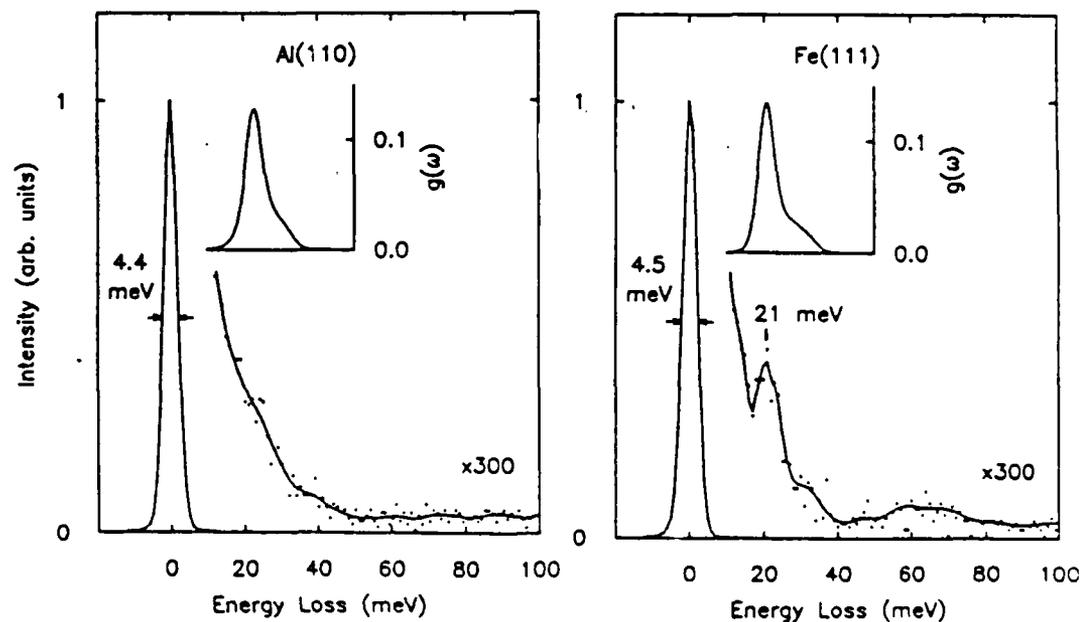
**Fig. 4** Electron energy loss spectrum of (a) the Al(110) surface and (b) the Fe(111) surface. The spectra were recorded at 300 K in the specular direction. The inset shows the dipole projected to account for the instrumental resolution. The force constants were obtained from a Born-von Karman analysis of the measured longitudinal bulk phonon dispersions. A small amount of oxygen contamination, less than 1%, is observed for Fe(111) around 60 meV.
