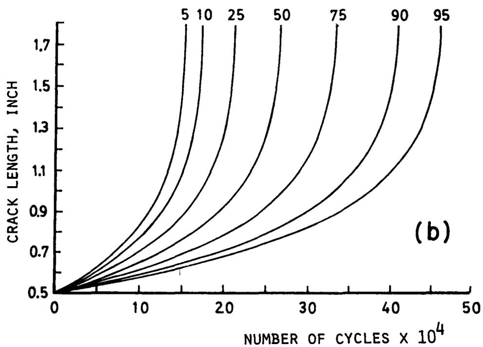
Figure 7: Experimental Constant-Probability Crack Growth Curves for a) Test Condition I and b) Test Condition II (Ref.(16))
