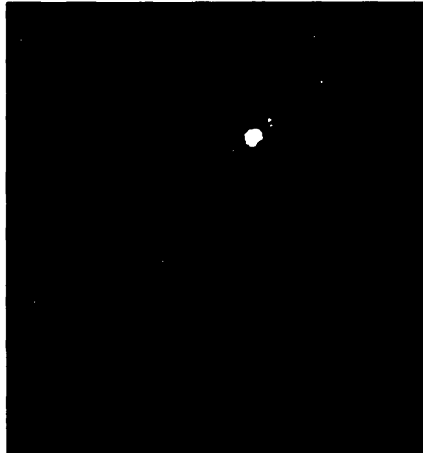
FIGURE 1a OPTICAL MICROGRAPH OF THIN JOINT REGION Bright region is a W-Fe particle.
