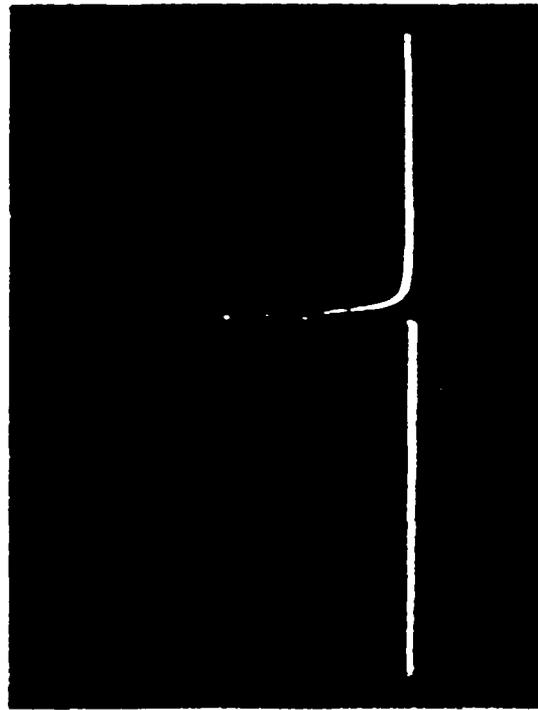
**Figure 14** - Laser output as detected by a PIN diode. (A): Relaxation mode output, 0.1V, 0.2ms/div. A calorimeter measured the total output energy in this shot to be 1.7 Joules. (B): Q-switched output, 1V, 1us/div, output energy = 0.8 J.
