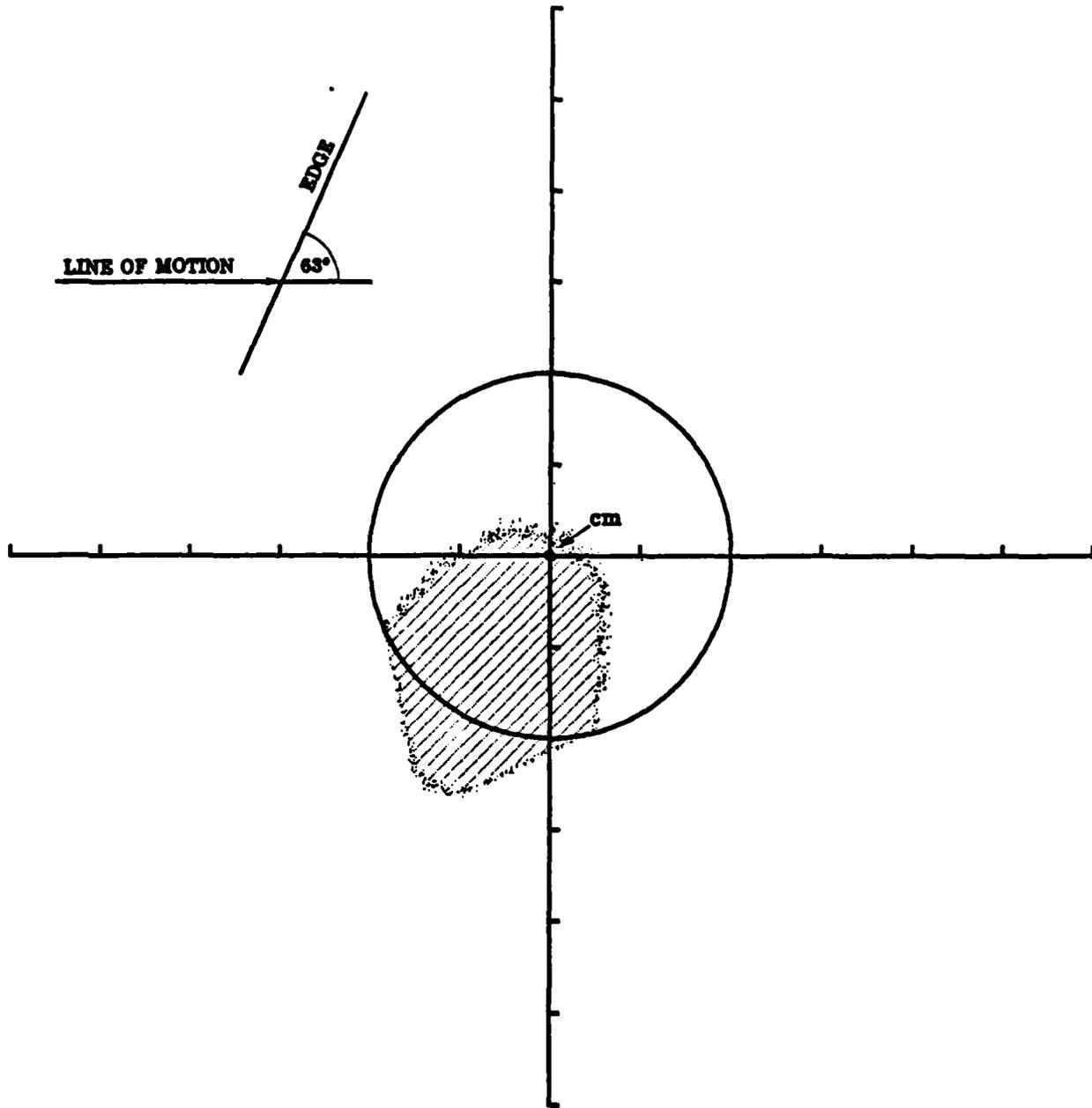
Figure 2-3: COR locus found by iterative minimization (dots)
