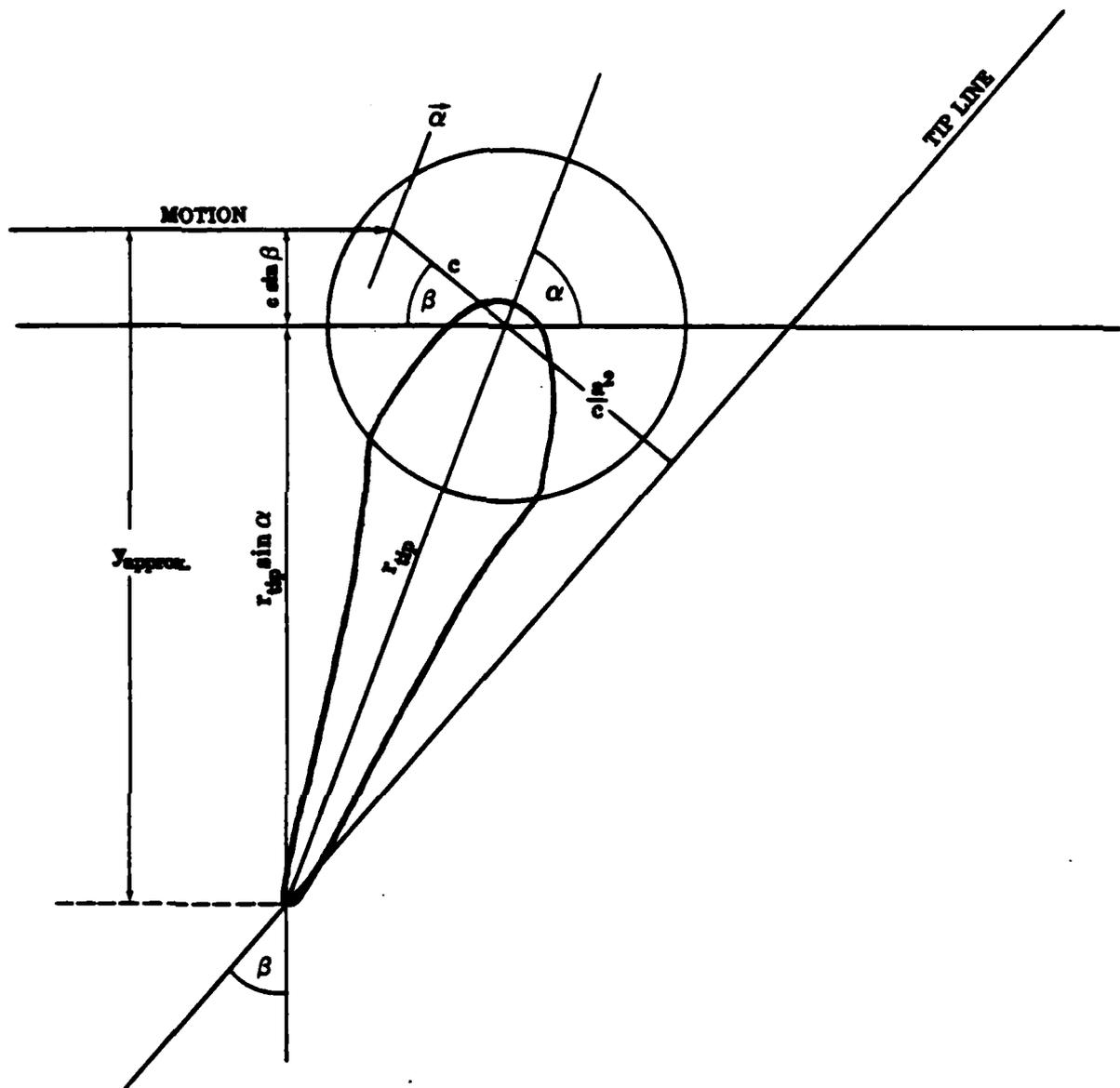
Figure 6-3:  $y_{approx}$  is the distance from the line of motion to the tip of the COR locus
