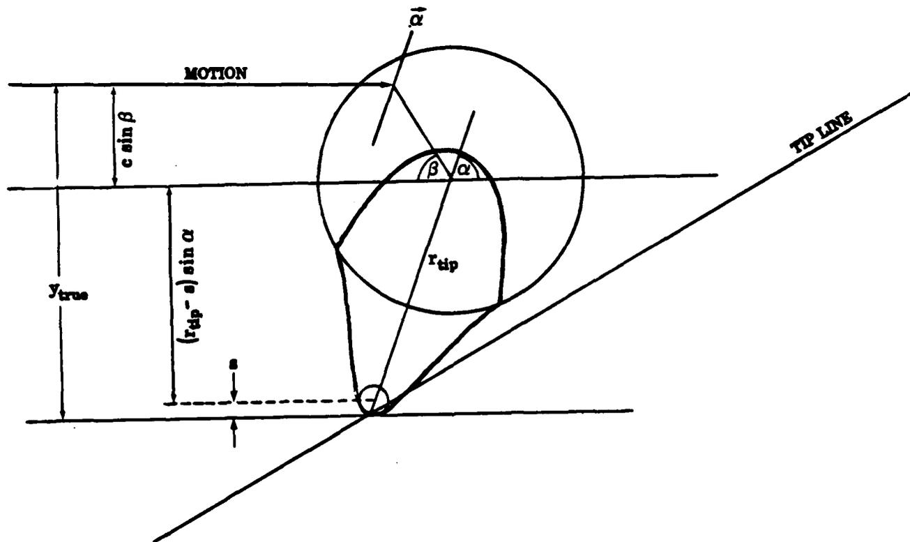
Figure 6-4:  $y_{true}$  is a bound for the distance from the line of motion to the true lowest point
