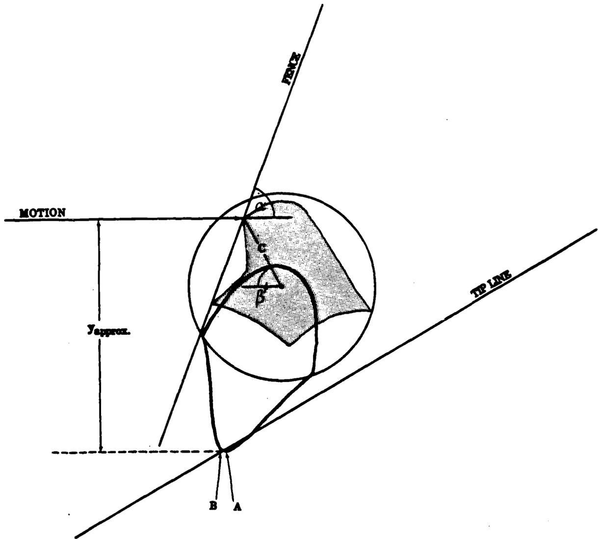
Figure 6-2: Final configuration of object and fence, and resulting COR locus
