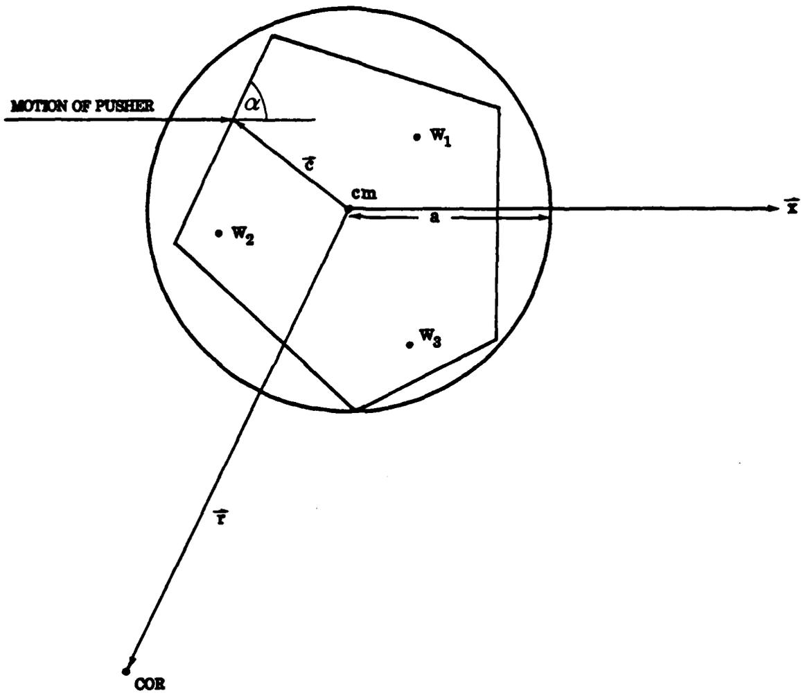
Figure 2-2: Parameters of the pushing problem
