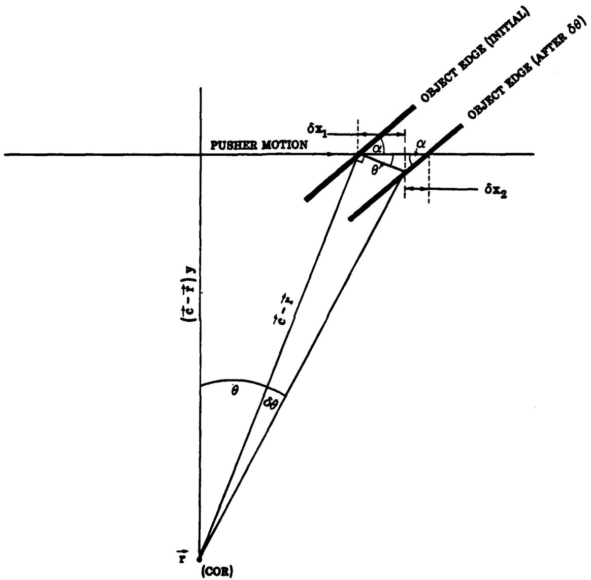
Figure 3-1: Relation between advance of pusher ( $\delta x$ ) and rotation about the COR ( $\delta\theta$ )
