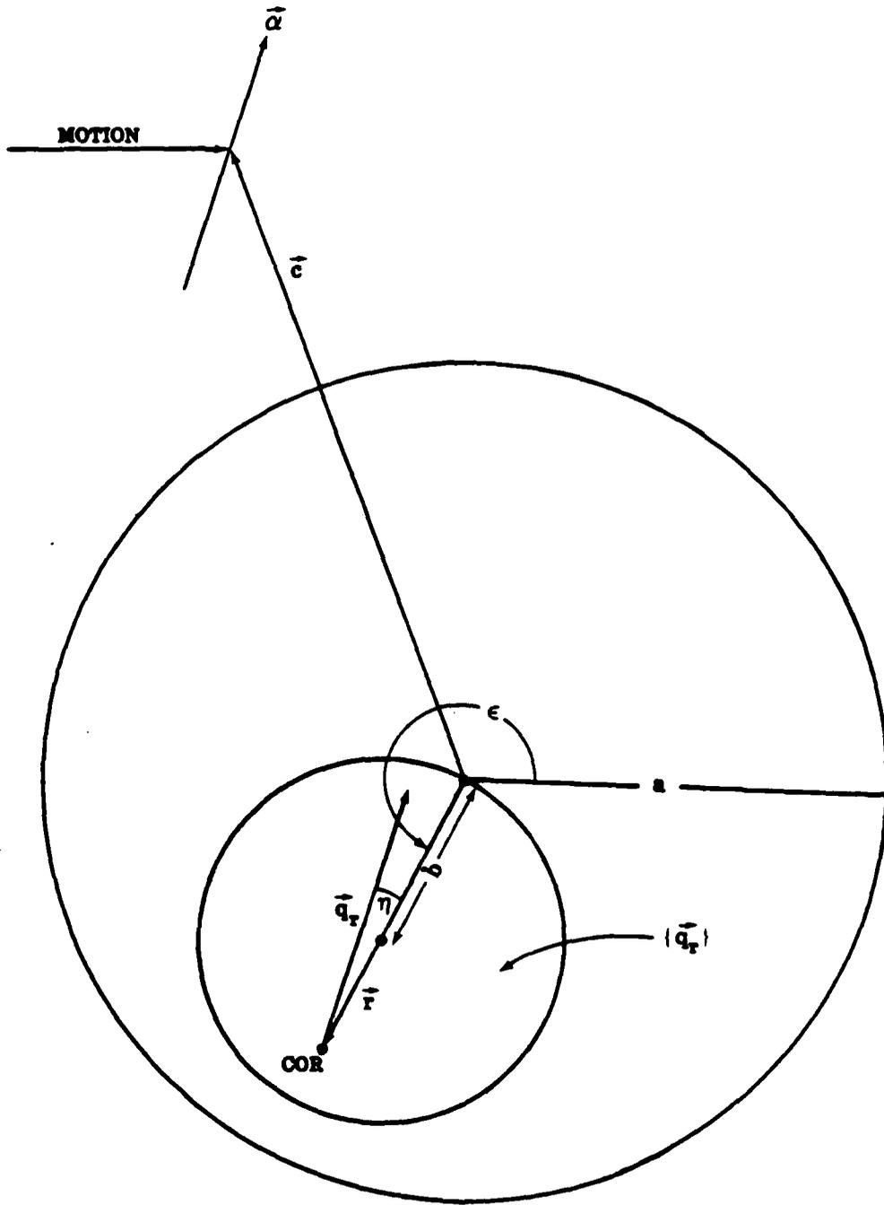
Figure 5-3: Variables of equation 23, for a value of  $\vec{r}$  in the COR locus
