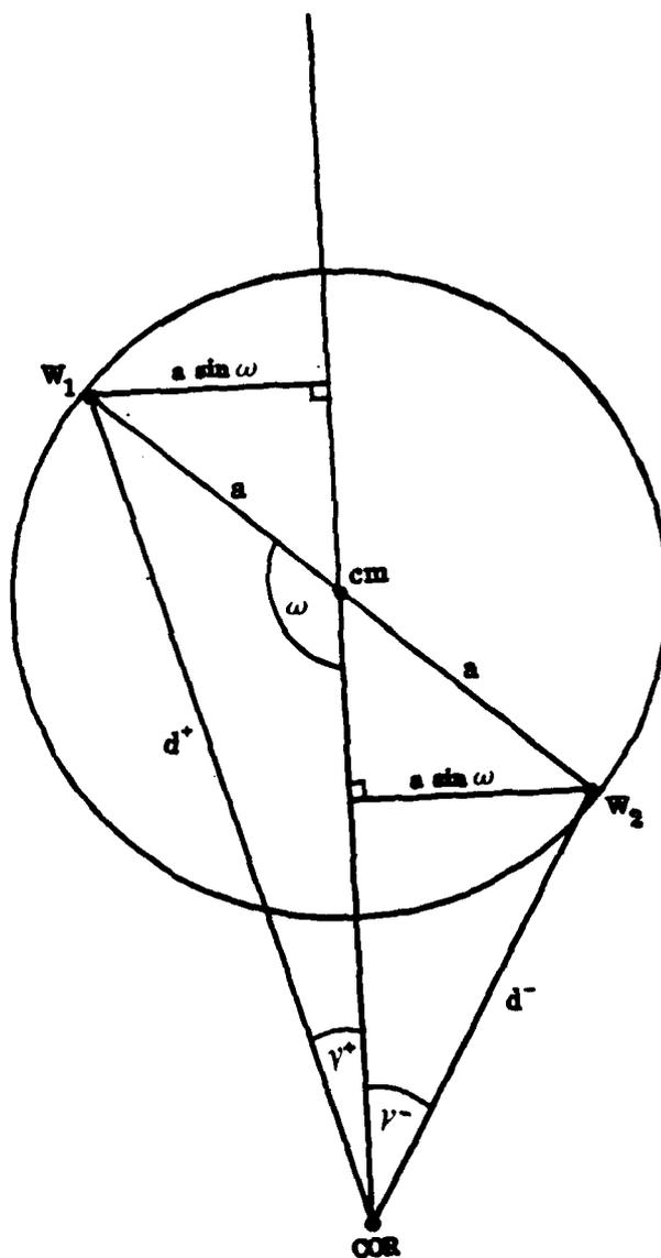
Figure 4-6: Dipoles contributing to the boundary of  $\{\vec{q}_r\}$ , for  $r > a$
