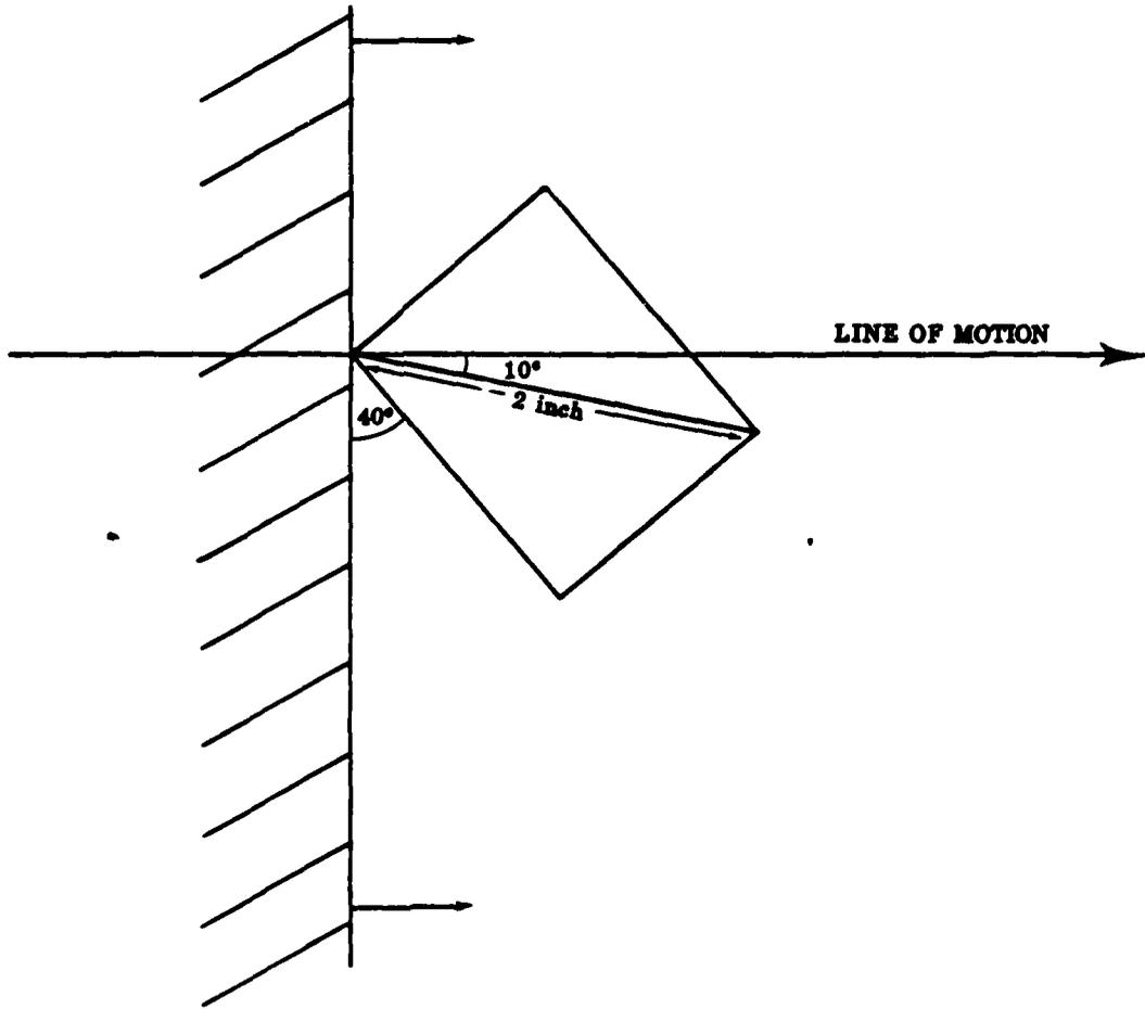
Figure 1-2: The fence must advance 2.02 inches to assure that the rectangle is aligned
