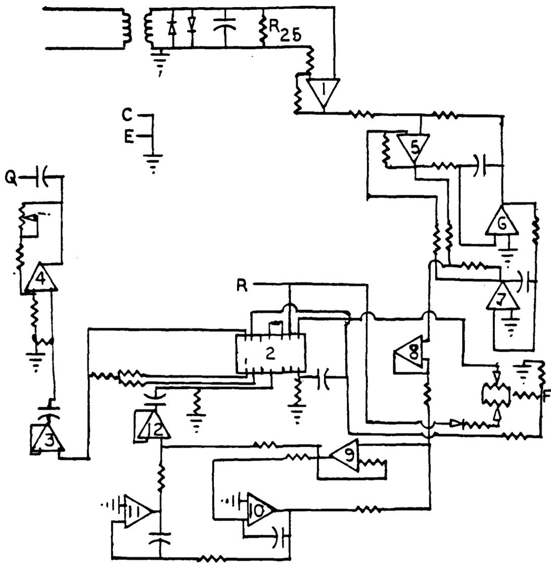
Fig. 8. Schematic of the Receiver Board of the Aerovironment Model 300.
