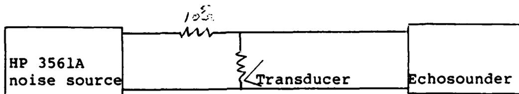
Fig. 12. Connection of Noise Source to Transducer
