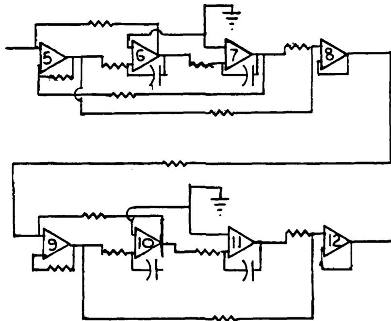
Fig. 9. Schematic of the High and Low Pass Filters of the Receiver Board of Aerovironment Model 300.
