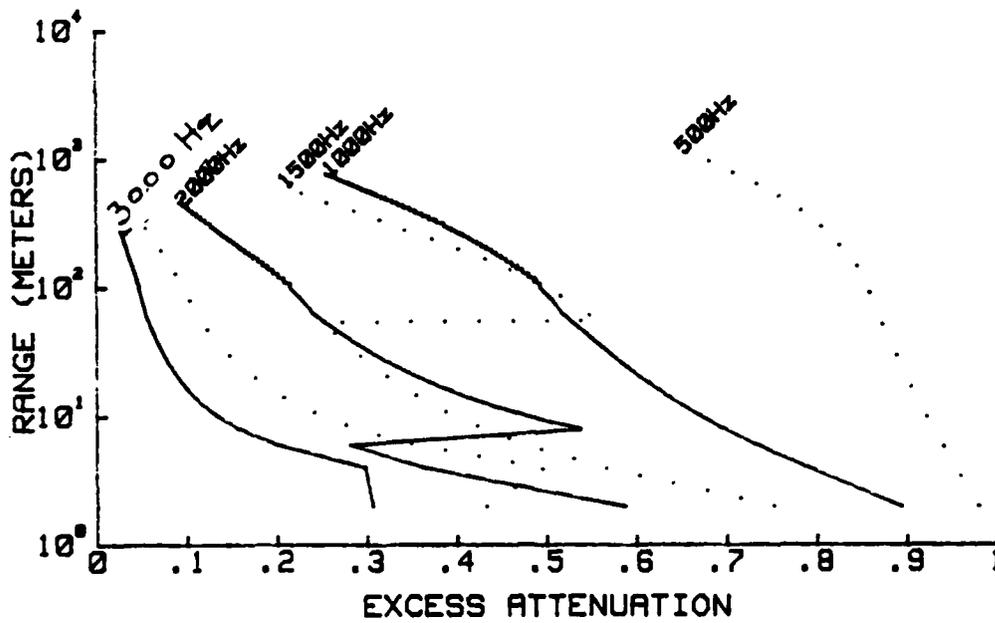
Fig. 7. Range versus Excess Attenuation for an Antenna Diameter of 1.5 m.
