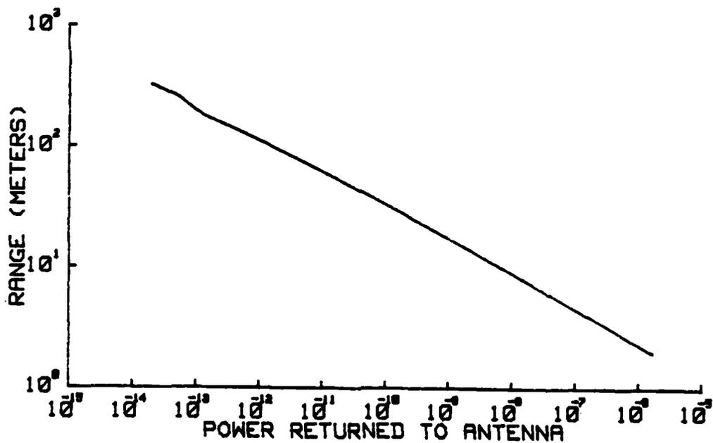
Fig. 29. Range versus Power Returned to the Antenna for  $C_T^2$  Profile 4, Parameters of the Aerovironment Model 300, and S.T.P.
