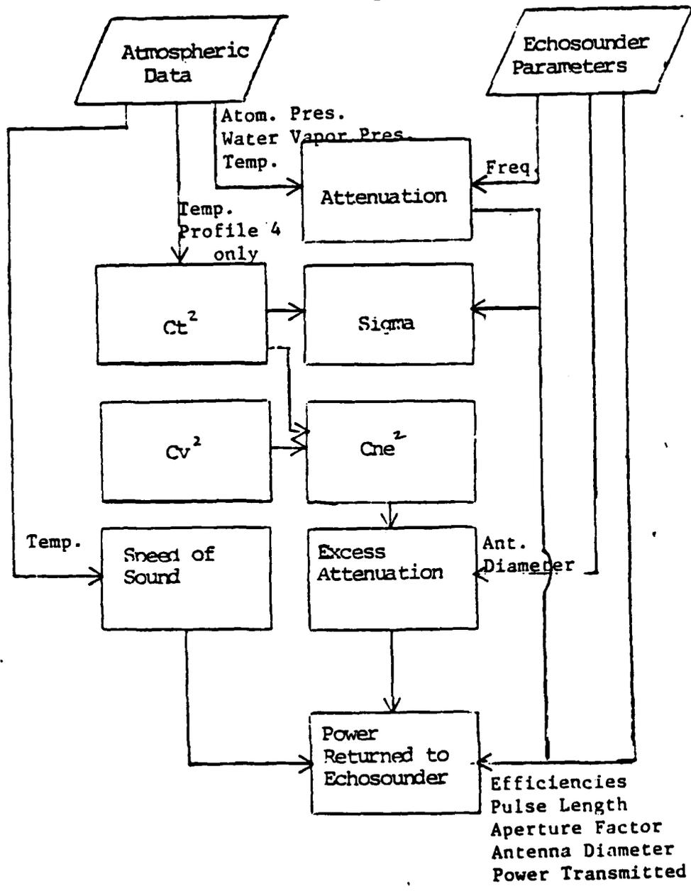
Fig. 27. Input Flow Chart for Computer Model
