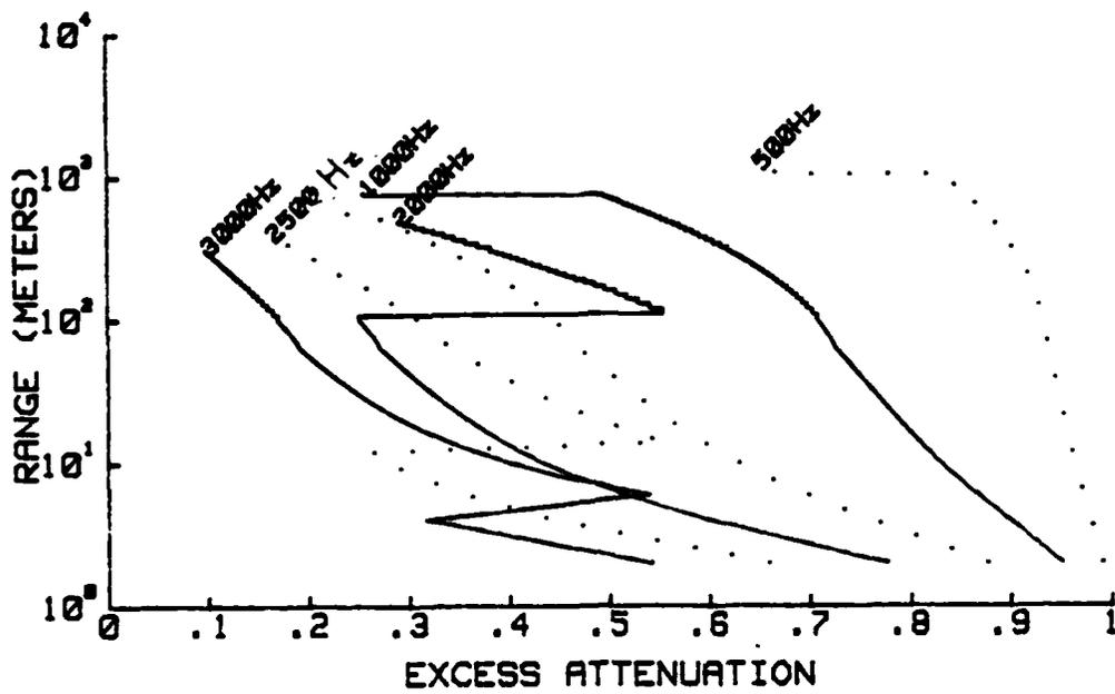
Fig. 6. Range versus Excess Attenuation for an Antenna Diameter of 1.0 m.
