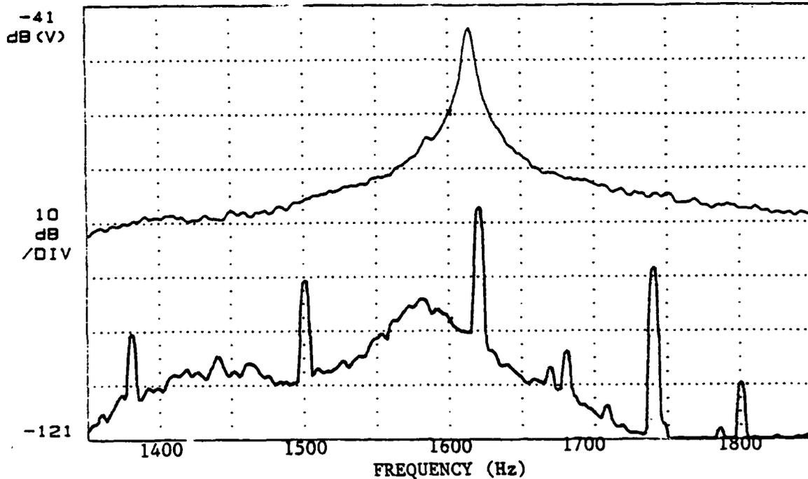
**Fig. 15. Frequency Spectrum of the Input Transformer
