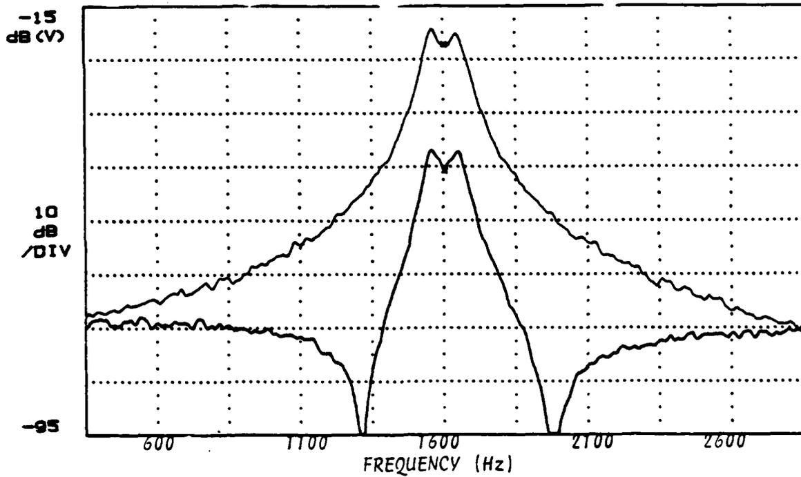
Fig. 18. Frequency Spectrum of the Receiver Board with  $R_0 = \infty$
