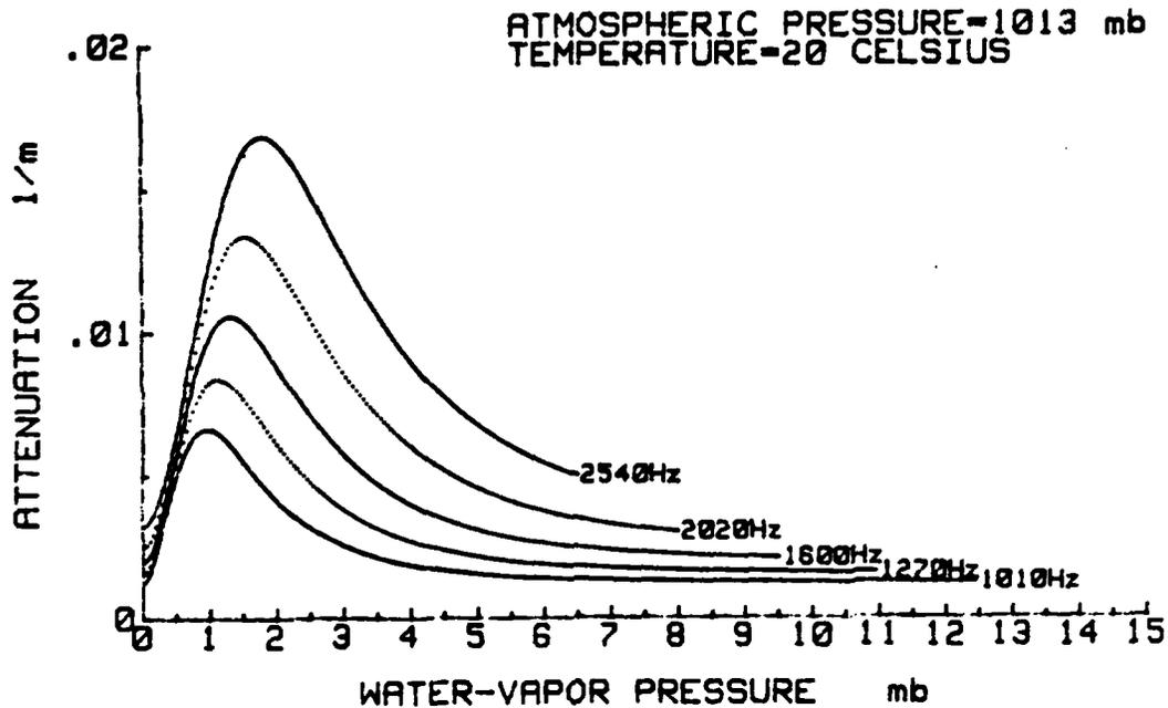
Fig. 1. Attenuation versus Water-vapor Pressure (mb.)
