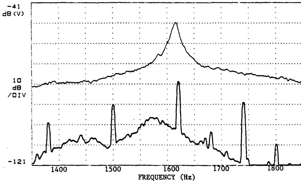
**Fig. 16. Frequency Spectrum of the Input Transformer
