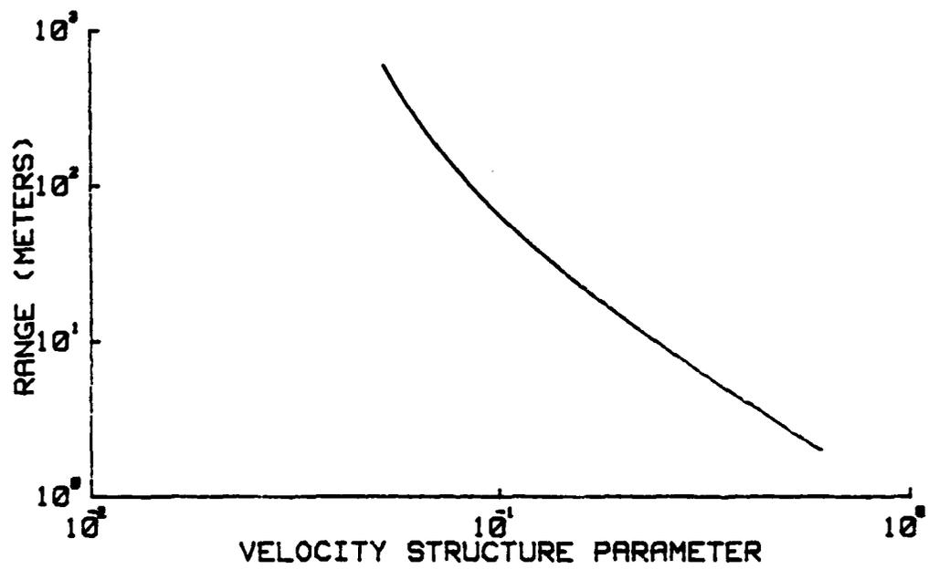
Fig. 21. Velocity Structure Parameter ( $C_v^2$ ) Profile.
