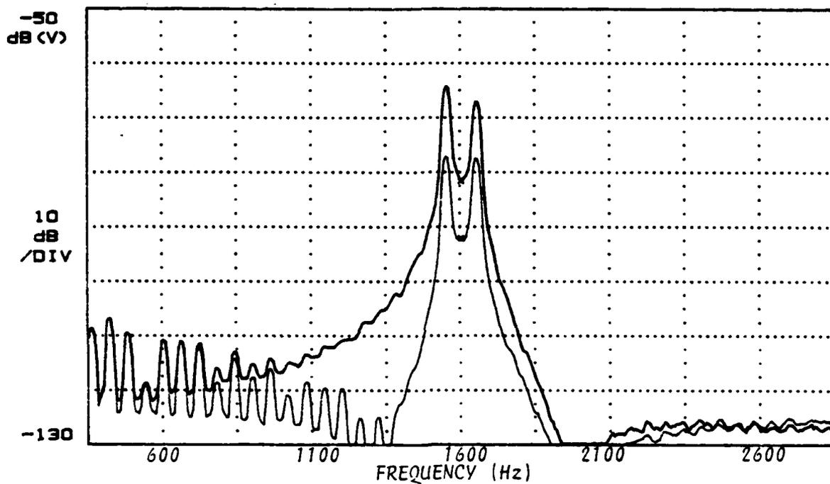
Fig. 20. Frequency Spectrum of the Receiver Board with  $R_0=560 \Omega$  (input before filters)
