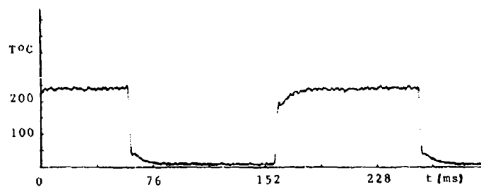
Fig. 10 Compensated junction temperature history (laser heating)
