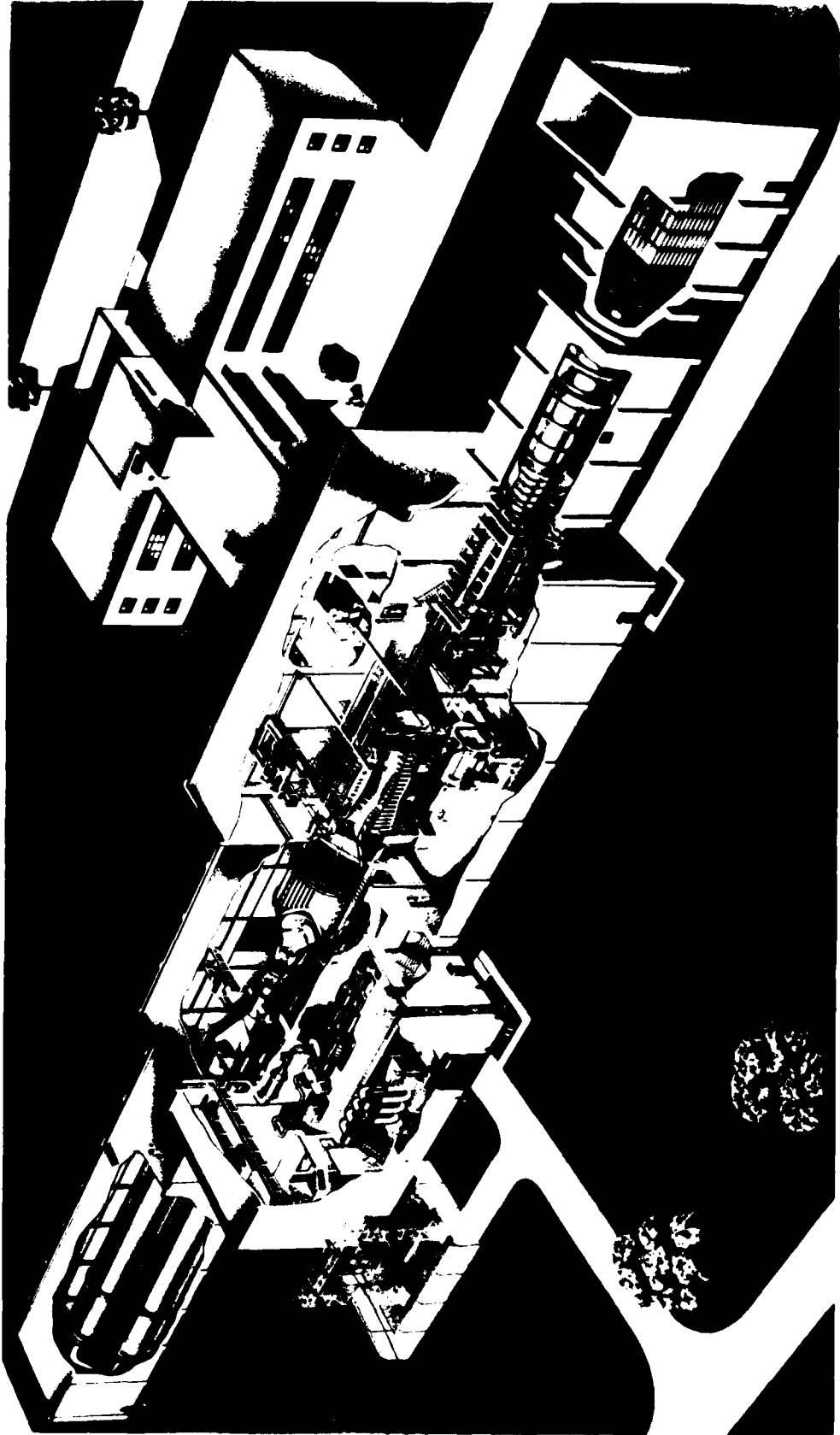
FIG. 1: CUT-AWAY VIEW OF NAE 5 FT X 5 FT WIND TUNNEL
