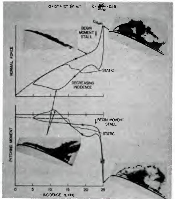
Figure 83 Normal force and pitching moment on NACA 0012 airfoil during dynamic stall. ( $\alpha = 15^\circ + 10^\circ \sin \omega t$ ,  $k = \frac{\omega c}{2U_\infty} = 0.15$ ,  $Re = 2.5 \times 10^6$ ). From McCroskey, Carr, and McAlister (1976).
