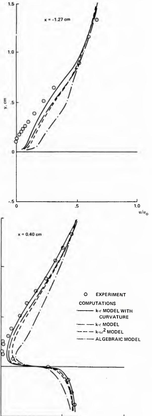
Fig. 70 Comparison between computations of Horstman (1982) and experimental mean-velocity profiles of Viswanath and Brown (1980, 1983) employing various turbulence models.  $M = 0.7$  Freestream unit Reynolds number  $4.0 \times 10^7/m$ .
