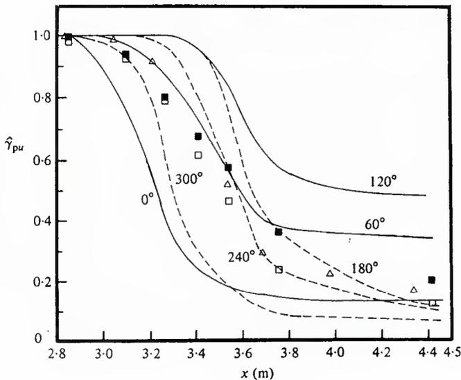
Figure 78 Phase-averaged  $\hat{\gamma}_{p_{min}}$  vs.  $x$  for different phases of a cycle shown by lines for  $k = 0.61$  Simpson et al. (1983) flow. Cycle-averaged  $\hat{\gamma}_{p_{min}}$  values shown by symbols and legend from Figure 1.
