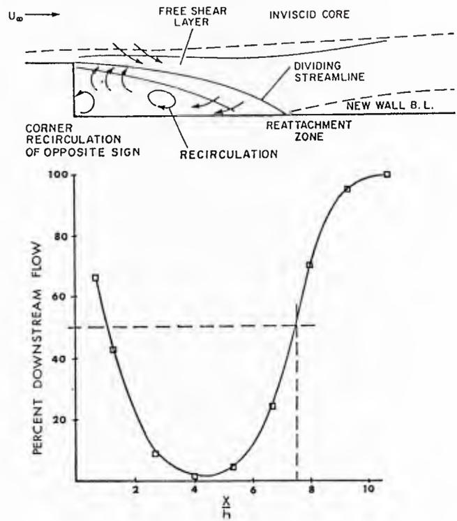
Fig. 43 Typical plot of the percent downstream flow ( $\gamma_p$ ) for the backward-facing step flow. From Eaton and Johnston (1980).
