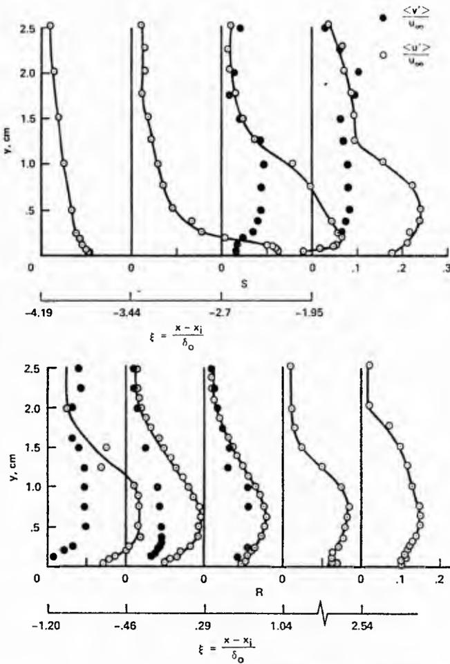
Figure 75 Turbulence intensity profiles. Modarress and Johnson (1976).
