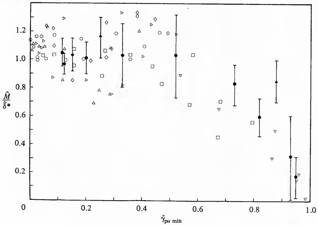
Fig. 29 Distance  $\hat{M}$  from wall to where  $\hat{\gamma}_{pu}$  is 0.99, normalized on  $\delta^*$ . Steady-flow data:  $\blacktriangle$ , Simpson et al. (1977);  $\bullet$ , Simpson et al. (1981a). Note the uncertainty bands. Unsteady flow,  $k = 0.90$ ;  $\nabla$ , 3.00 m;  $\square$ , 3.25 m;  $\triangle$ , 3.45 m;  $\diamond$ , 3.67 m;  $\circ$ , 3.98 m;  $\triangleright$ , 4.34 m. From Simpson and Shivaprasad (1983).
