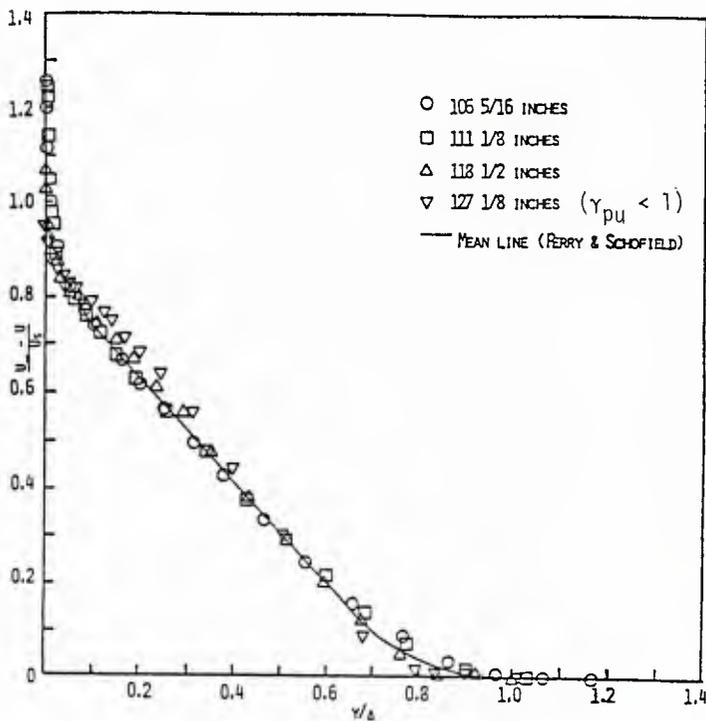
Fig. 20. Perry and Schofield outer region correlation for the Simpson et al. (1981a) data near detachment,  $(U_{\infty} - U)/U_S$  vs.  $y/\Delta$ , equation (IV.4); solid line is mean line from Perry and Schofield (1973).
