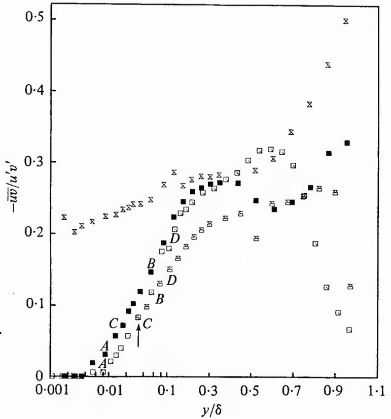
Fig. 33 Reynolds shear stress correlation coefficient profiles  $-\bar{w}w'/u'v'$  vs.  $y/\delta$  in the detached flow region:  $\times$ , 134.5 in.;  $\blacksquare$ , 138.8 in.;  $\boxplus$ , 144.8 in.;  $\square$ , 156.4 in. Letters A-D denote turbulence profile inflection points noted by Shiloh et al. (1981). The arrow denotes the location of the minimum mean velocity. Note the log-linear abscissa. From Simpson et al. (1981a).
