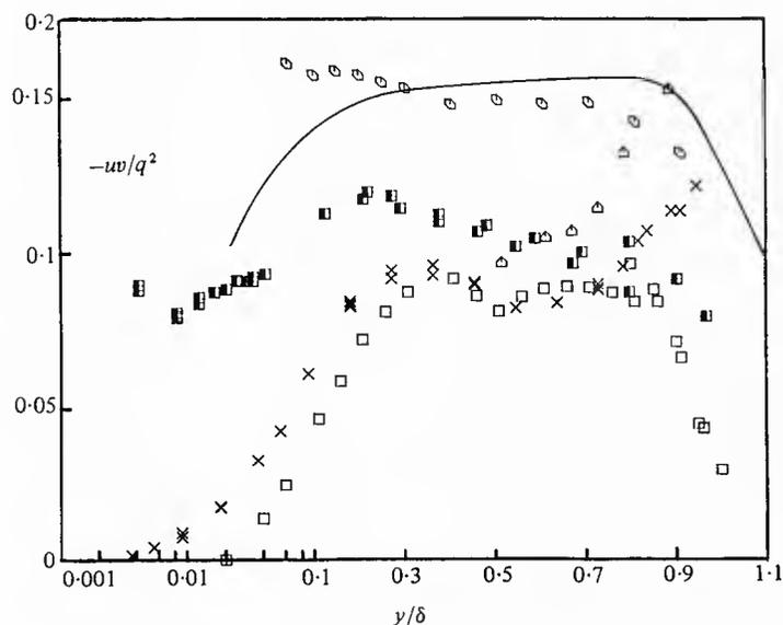
Fig. 34 Turbulence-energy correlation-coefficient  $-\overline{uv}/q^2$  distributions using the  $u'^2$ ,  $v'^2$  and  $-\overline{uv}$  data of Simpson et al. (1981a) and present  $w'^2$  data:  $\circ$ , 63.8 in.;  $\blacksquare$ , 115.5;  $\blacktriangle$ , 126.0;  $\times$ , 138.7;  $\square$ , 160.3. —, Bradshaw (1967) zero-pressure-gradient flow. Note the log-linear abscissa. From Shiloh et al. (1981).
