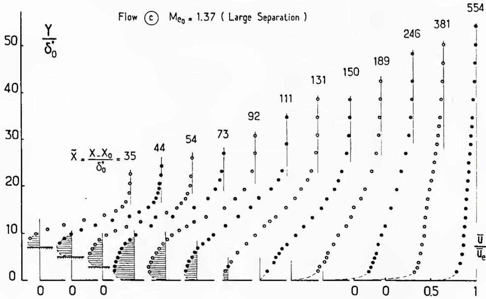
Fig. 65 Mean streamwise velocity profiles for flow C (Délery, 1983).
