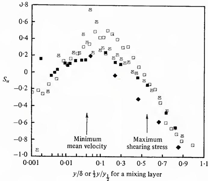
Fig. 38 Skewness-factor  $S_u$ , laser-anemometer data downstream from detachment. Note the log-linear abscissa.  $\blacksquare$ , 138.75 in.;  $\square$ , 144.9;  $\square$ , 156.4.  $\blacklozenge$ , Wygnanski & Fiedler (1970), mixing-layer data. Simpson et al. (1981b).
