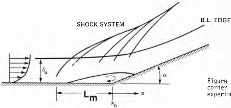
Figure 71 Geometry of supersonic compression corner shock-wave boundary-layer interaction experiment.
