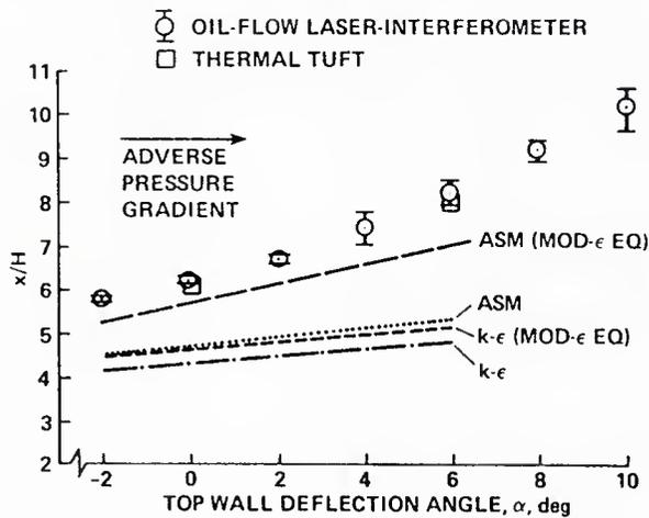
Figure 92 Reattachment location versus top-wall deflection angle. Calculations of Sindir (1982). Data of Driver and Seegmiller (1982).
