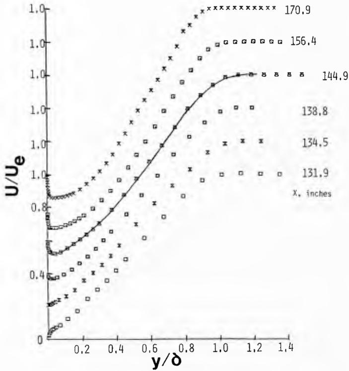
Fig. 22 Detaching flow mean velocity profiles (Simpson *et al.*, 1981a) from laser and hot-wire anemometer data. Note displaced ordinates. Solid line denotes  $Re_{\theta} = 47000$ ,  $H = 5.38$  data of Hastings and Moreton (1982).
