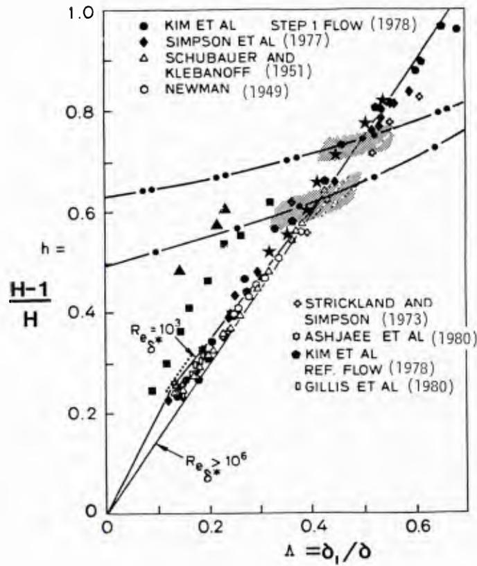
Fig. 26  $h$  vs.  $\delta^*/\delta$  plot of data for detaching and reattaching flows. Shaded regions - data reviewed by Sandborn and Kline (1961). ---, equations (6) and (7) of Kline et al. (1983); ---, equation (IV.13); ■, data of Chou and Sandborn (1973); ▲, data of Sandborn and Liu (1968); ★, data of Wadcock (1979); ·····, data of So and Mellor (1972).
