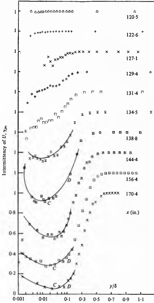
Fig. 28 Streamwise fraction of time the flow moves downstream with the locations of inflection points C and D from Shiloh et al., (1981). Solid lines are for visual aid only. Note the log-linear abscissa and displaced ordinates. From Simpson et al. (1981a).
