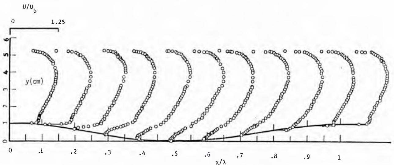
Fig. 25 Mean velocity profiles on eighth of ten waves of the Buckles et al. (1983) wavy channel flow  $U_b = 51 \text{ cms}^{-1}$ ;  $2h = 47.4 \text{ mm}$ ;  $\lambda = 50.8 \text{ mm}$ ;  $2a/\lambda = 1/8$ ;  $U_b(2h)/\nu = 12000$ .
