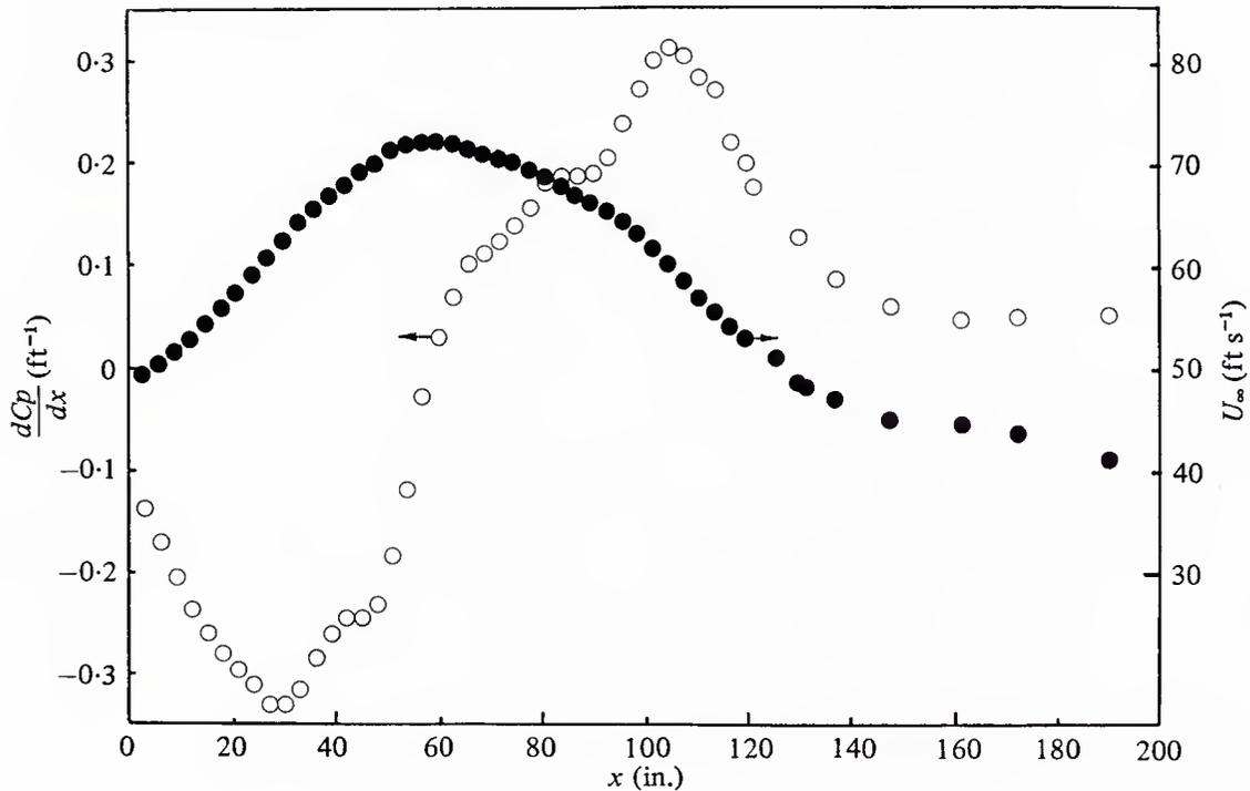
Fig. 17. Free-stream velocity and pressure gradient distributions along the tunnel centre-line.
