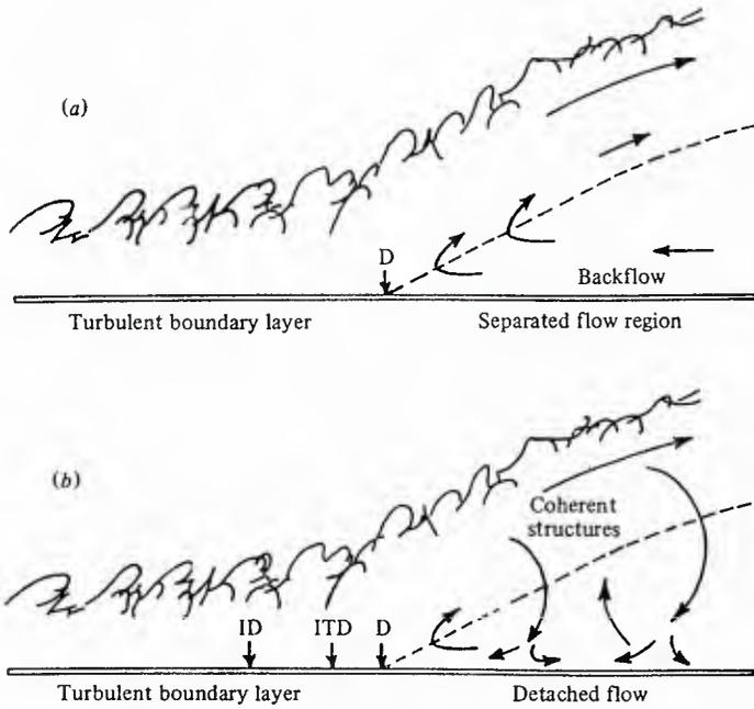
Fig. 42 (a) Traditional view of turbulent-boundary-layer separation with the mean backflow coming from far downstream. The dashed line indicates  $U = 0$  locations. (b) A flow model with the coherent structures supplying the small mean backflow. ID denotes incipient detachment; ITD denotes intermittent transitory detachment; D denotes detachment. The dashed line denotes  $U = 0$  locations. See Figure 18. From Simpson et al. (1981b).
