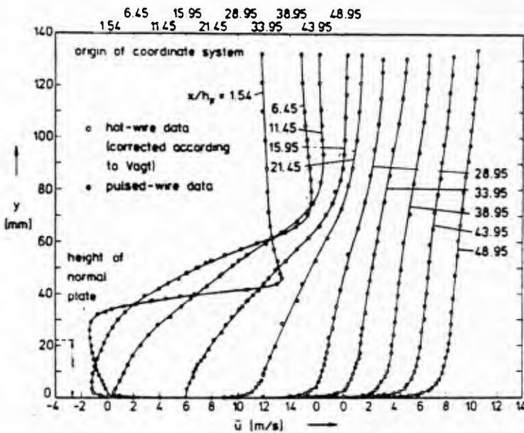
Fig. 60 Mean velocity distribution downstream of the normal plate along the centerline of the splitter plate shown in Figure 53. From Ruderich and Fernholz (1983). ( $Re_{h_p} = 1.4 \times 10^4$ )
