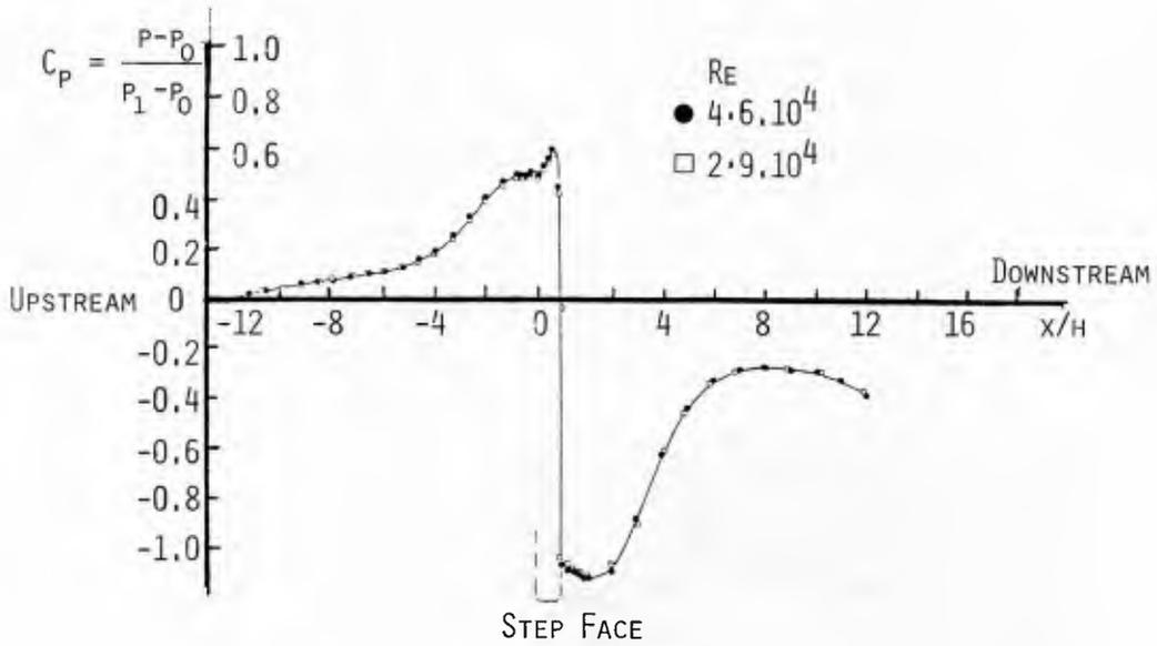
Fig. 59 Surface pressures for a front-facing step flow. From Moss and Baker (1980).
