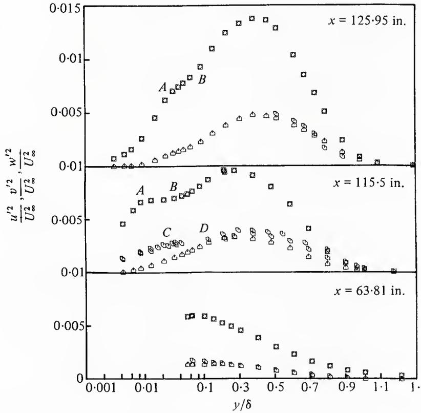
Fig. 30 Reynolds normal stresses distributions upstream of intermittent transitory detachment. Simpson et al. (1981a):  $\square$ ,  $u'^2/U_\infty^2$ ;  $\triangle$ ,  $v'^2/U_\infty^2$ ;  $\circ$ ,  $w'^2/U_\infty^2$ . Note the log-linear abscissa.
