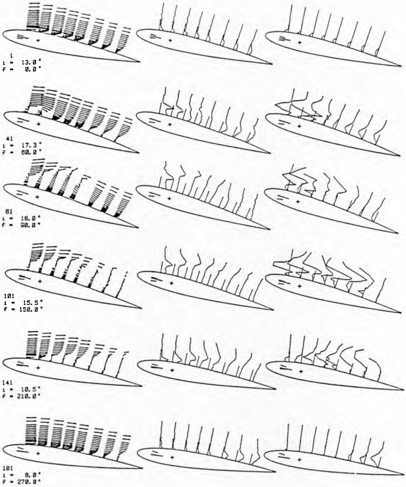
Figure 84 Slanted hot-wire anemometer measurements on a NACA 0012 airfoil oscillating sinusoidally about the quarter chord at unstalled to deeply stalled conditions.  $k = 0.3$ ;  $Re_c = 3 \times 10^5$ ;  $i$  denoted instantaneous angle of incidence;  $f$  is phase angle in cycle. From DeRuyck and Hirsch (1984).
