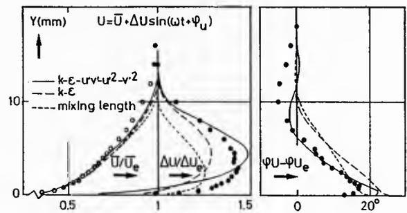
Figure 93 Unsteady turbulent boundary layer in an adverse pressure gradient. Harmonic analysis of the calculated velocity. Comparison with experiment.  $X = 390$  mm. From Cousteix, et al. in Michel et al. (1981).
