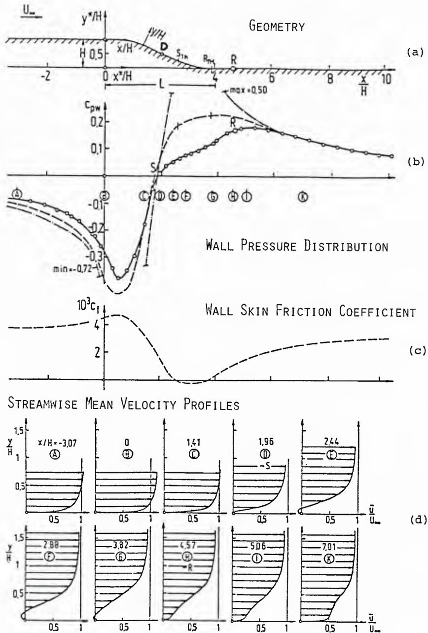
Fig. 41 Gersten, Wauschkuhn, and Pagendarm (1983) curved wall flow: (a) geometry; (b) surface pressure distribution; (c) calculated  $C_f$  from inverse method with interaction; (d) streamwise mean velocity profiles. -o-o-o-, measurements; - - - - -, potential flow theory.
