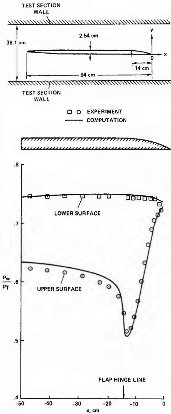
Fig. 69 Geometry and surface pressure distributions for the Viswanath and Brown (1980, 1983) trailing edge flow. Calculations by Horstman (1982) using the Jones-Lauder (1972)  $k-\epsilon$  model with Cousteix (Kline et al., 1982) curvature correction.
