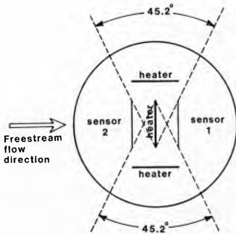
Fig. 4. Schematic planview of the modified "thermal tuft" or downstream-upstream flow direction intermittency probe. Sensors and central heater are 6 mm long 2.5 mm apart; 5 mm long side heaters are 2.5 mm from end of sensors. From Shivaprasad and Simpson (1982).
