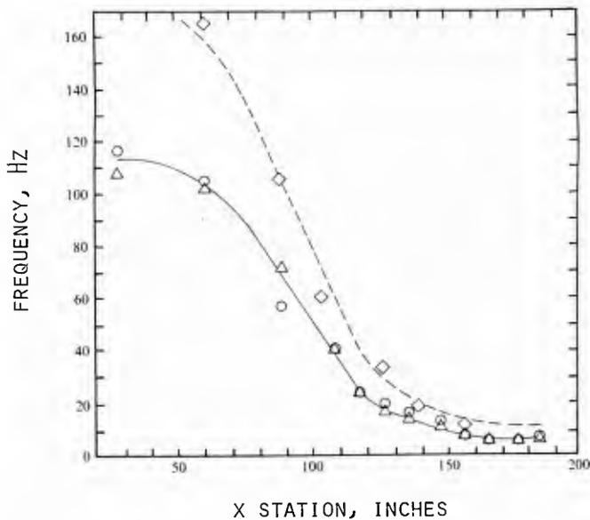
Fig. 40 Bursting and outer region turbulent-non-turbulent intermittency frequencies.  $\circ$ , autocorrelation;  $\triangle$ , spectra bursting results;  $\diamond$ , intermittency results. Lines for visual aid only. From Simpson et al. (1977).
