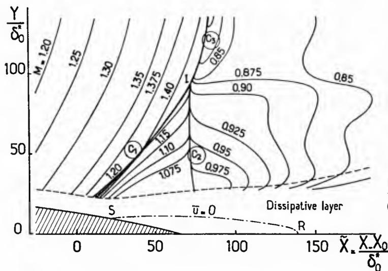
Fig. 63 Inviscid flowfield structure of flow C of Détery (1983).  $M_e = 1.37$ ,  $\delta_0^* = 0.52$  mm,  $H_{i0} = 1.27$ ,  $Re_{\theta 0} = 3800$
