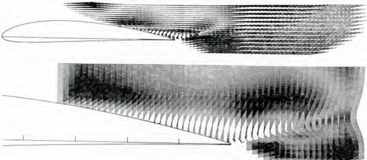
Fig. 12. Mean velocity vectors of separated flow on NACA 4412 airfoil at maximum lift and  $Re_c = 1.5 \times 10^6$ . Bottom figure is close-up of detached flow. Tick marks denote 0.1 of  $x/c$  intervals. Coles and Wadcock (1979).
