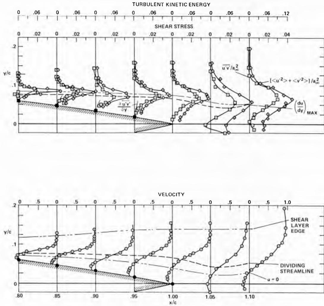
Fig. 68 Mean velocity, turbulent shear stress, and kinetic energy profiles in the shear layer downstream of detachment.  $M_\infty = 0.79$  and  $Re_c = 11 \times 10^6$ . Seegmiller et al. (1978).
