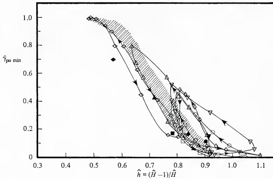
Figure 80  $\hat{\gamma}_{pu\min}$  vs.  $\hat{h}$  for the  $k = 0.90$  unsteady flow of Simpson and Shivaprasad (1983) from LDV data:◇, 3.00m;△, 3.25 m; □, 3.45 m;◇, 3.67 m;○, 3.98 m;▽4.34 m. Solid lines form hysteresis loops for data at a given streamwise position. Shaded region denotes steady-flow results presented by Simpson et al.(1983). Solid symbols denote mean unsteady-flow results.
