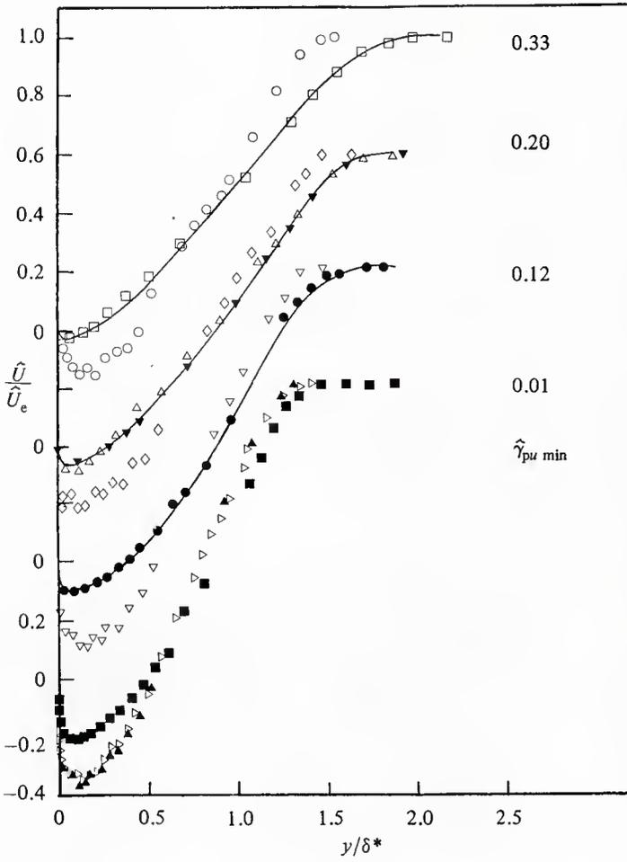
Figure 79 Phase averaged velocity profiles  $\hat{u}/\hat{u}_e$  vs.  $y/\delta^*$  for several values of  $\hat{\gamma}_{pu\min}$  for  $k = 0.90$  Simpson and Shivaprasad flow (1983). Solid lines denote profiles from the steady flow of Simpson et al.(1981a) at the  $\hat{\gamma}_{pu\min}$  value. Note displaced ordinates. Conditions for each profile are as below.
