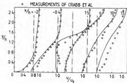
Fig. 62(a) Velocity predictions and LDA measurements for flow over square rib. — Calculations of Benodehar et al. (1983).
