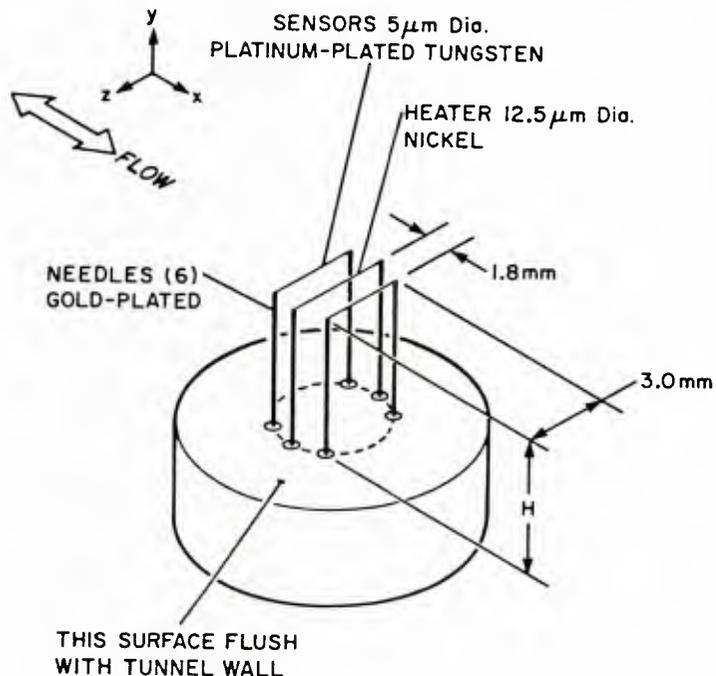
Fig. 7. Sketch of Pulsed-Wall Probe. Eaton, Westphal, Johnston (1982)
