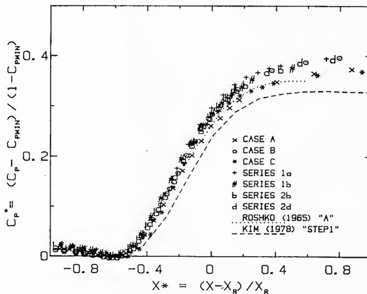
Fig. 49 Pressure distributions near reattachment, normalized as suggested by Roshko and Lau (1965). See Figure 47 for legend. From Westphal and Johnston (1983).
