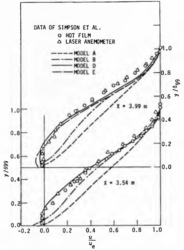
Figure 89(b) Comparison of predicted and experimental velocity profiles for the boundary layer with reversed flow measured by Simpson et al. (1977). From Pletcher (1978).
