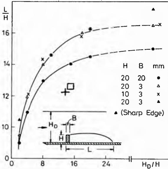
Fig. 58 Measured length of recirculation region. \* Castro and Fackrell (1978). □ Castro (1981). + Crabb et al. (1981). Other data from Durst and Rastogi (1979) with  $\delta_j = 10$  mm at 150 mm upstream of fence.
