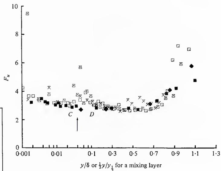
Fig. 35 Flatness-factor,  $F_u$ , profiles downstream from detachment note log-linear abscissa. C and D are the inflection points described by Shiloh et al. (1981).  $\blacksquare$ , 138.75 in.;  $\blacktriangle$ , 144.9;  $\square$ , 156.4;  $\times$ , 170.9. The arrow denotes the location of minimum mean velocity  $U$ .  $\blacklozenge$ , Wygnanski & Fiedler (1970), mixing-layer data. From Simpson et al. (1981b).
