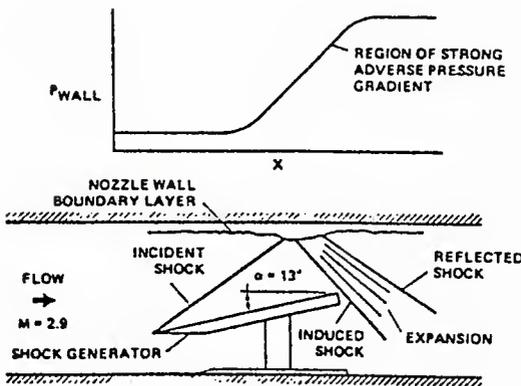
Figure 73 Flow model, shock-induced separation.  $P_{final}/P_{initial} = 5$ ;  $U_\infty/v = 5.7 \times 10^7/m$ . Modarress and Johnson (1976).
