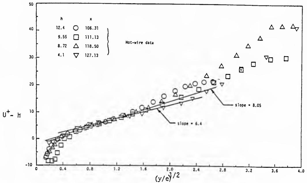
Fig. 19. Perry and Schofield inner region correlation for the Simpson et al. (1981a) data near separation,  $U^+ - h$  vs.  $(y/e)^{1/2}$ , equations (IV.6) and (IV.8) given by solid lines for 6.4 and 8.05 slopes.
