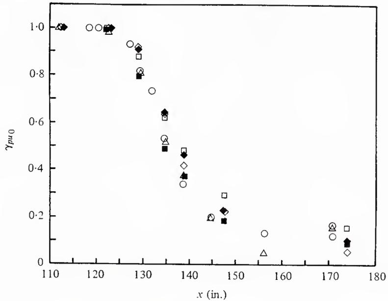
Fig. 1. Fraction of time that the flow 1.2 mm from the wall (outside viscous region) is in the downstream direction: ○, LDV direct measurement; △, LDV U and  $u'$  measurements and equation (2). Thermal tuft without side heaters: □, orientation 1; ■, reversed or orientation 2. Thermal tuft with side heaters: ◇, orientation 1; ◆, reversed or orientation 2. From Shivaprasad and Simpson (1982).
