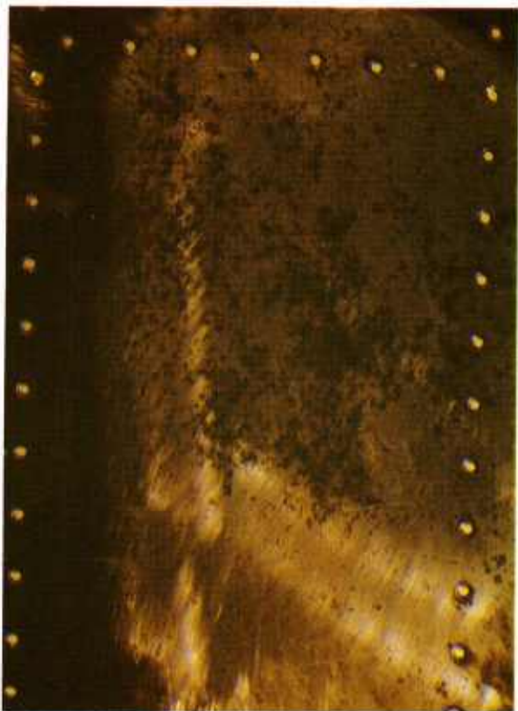
Fig. 7-4 Uniform corrosion in a magnesium alloy helicopter skin after damage to the chromate pre-treatment
