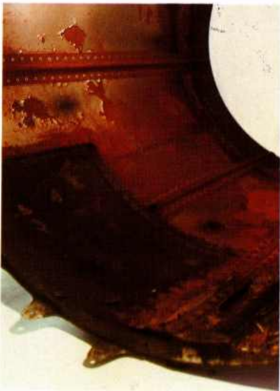
Fig. 7-2 Rusting in a jet pipe end cap liner following damage to its protective coating
