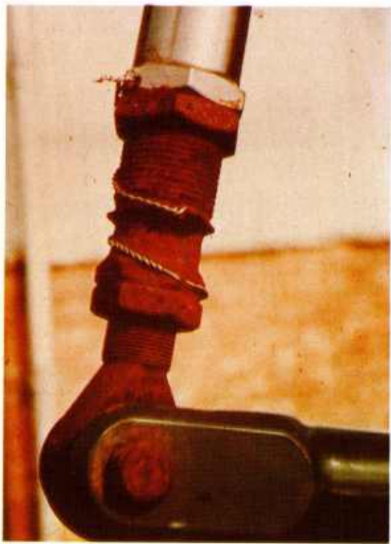
Fig. 7-1 Rusting on a steel track rod adjuster and eye after damage occurred to the protective cadmium plating
