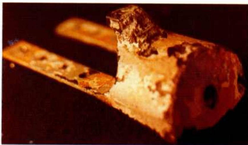
Fig. 9-1(b) Severe pitting in a cast magnesium alloy stringer end cap
