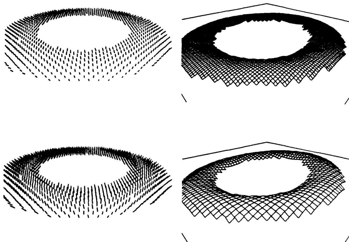
Figure 22. Reconstruction of the torus (right) from the orientation constraints provided by photometric stereo (left). (Grid dimensions  $N_x^{h_1} = N_y^{h_1} = 51$  and  $N_x^{h_2} = N_y^{h_2} = 101$ . Constraint parameters:  $\alpha^{h_j} = 4.0/h_j$ . Computation: 52.0 work units.)
