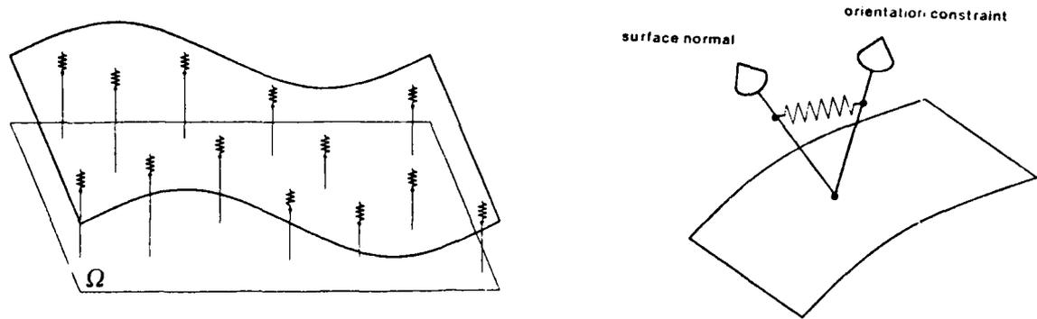
Figure 2. The physical model. Thin plate surface under tension and depth constraints (left). Local influence of an orientation constraint (right).
