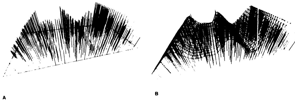
Figure 38. Scattered depth constraints consistent with sloping planes meeting discontinuously (top) and the smooth reconstructed surface (bottom).
