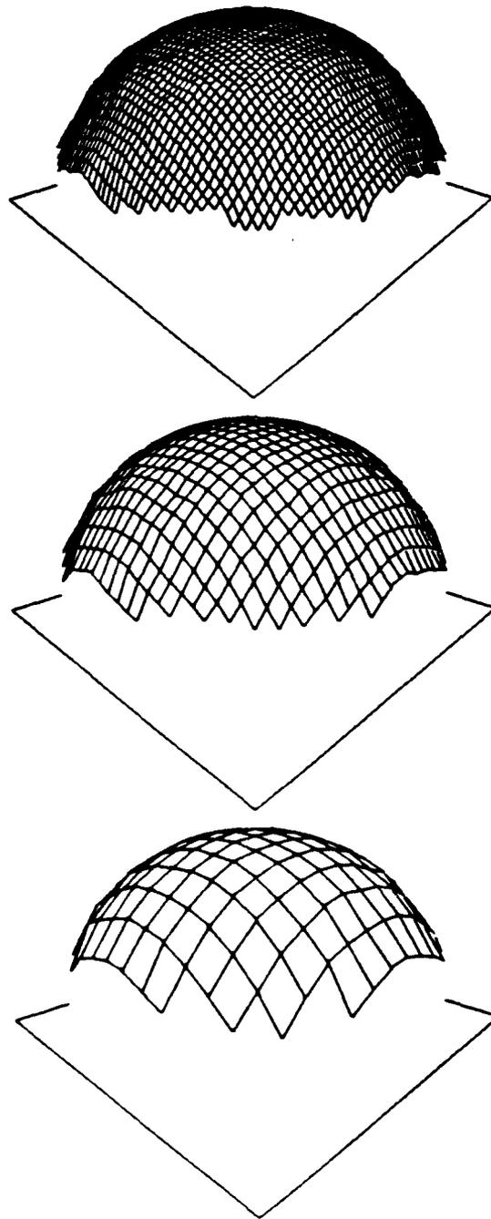
**Figure 19.** Reconstruction from depth and orientation constraints in Fig. 18. (Grid dimensions:  $N_x^{h_1} = N_y^{h_1} = 17$ ,  $N_x^{h_2} = N_y^{h_2} = 33$ ,  $N_x^{h_3} = N_y^{h_3} = 65$ . Grid spacings:  $h_1 = 0.4$ ,  $h_2 = 0.2$ ,  $h_3 = 0.1$ . Constraint parameters  $\alpha_d^{h_j} = 2.0/h_j$ ,  $\alpha_p^{h_j} = \alpha_q^{h_j} = 4.0/h_j$ . Computation: 17.75 work units.)
