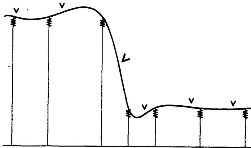
Figure 9. Cross-section of a reconstructed surface across a depth discontinuity. The significant and insignificant inflections of the surface are indicated.
