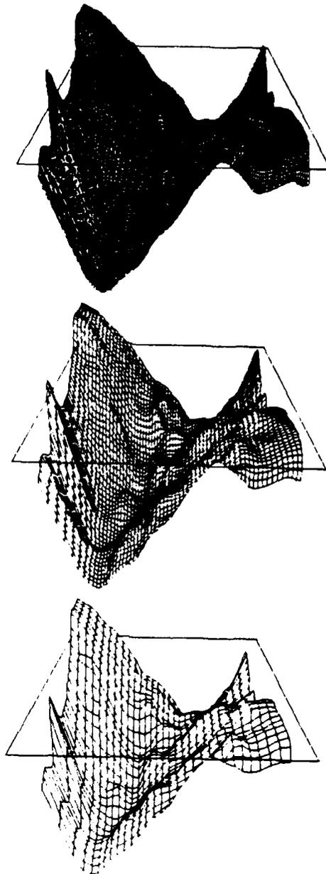
Figure 24. Reconstruction of terrain in Fig. 23. (Grid dimensions:  $N_x^{h_1} = N_y^{h_1} = 33$ ,  $N_x^{h_2} = N_y^{h_2} = 65$ ,  $N_x^{h_3} = N_y^{h_3} = 129$ ,  $N_x^{h_4} = N_y^{h_4} = 257$ . Grid spacings:  $h_1 = 0.8$ ,  $h_2 = 0.4$ ,  $h_3 = 0.2$ ,  $h_4 = 0.1$ . Constraint parameters:  $\alpha_d^{h_j} = 0.01/h_j^2$ . Computation: 29.0 work units.)
