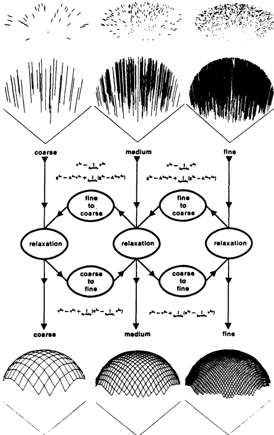
**Figure 13.** The structure of the multiresolution surface reconstruction algorithm. Iterative relaxation processes operate at each level. Fine-to-coarse and coarse-to-fine processes transfer information between levels. Synthetic orientation and depth constraints input to the algorithm are shown at the top. The dense multiscale surface representation is output at the bottom.
