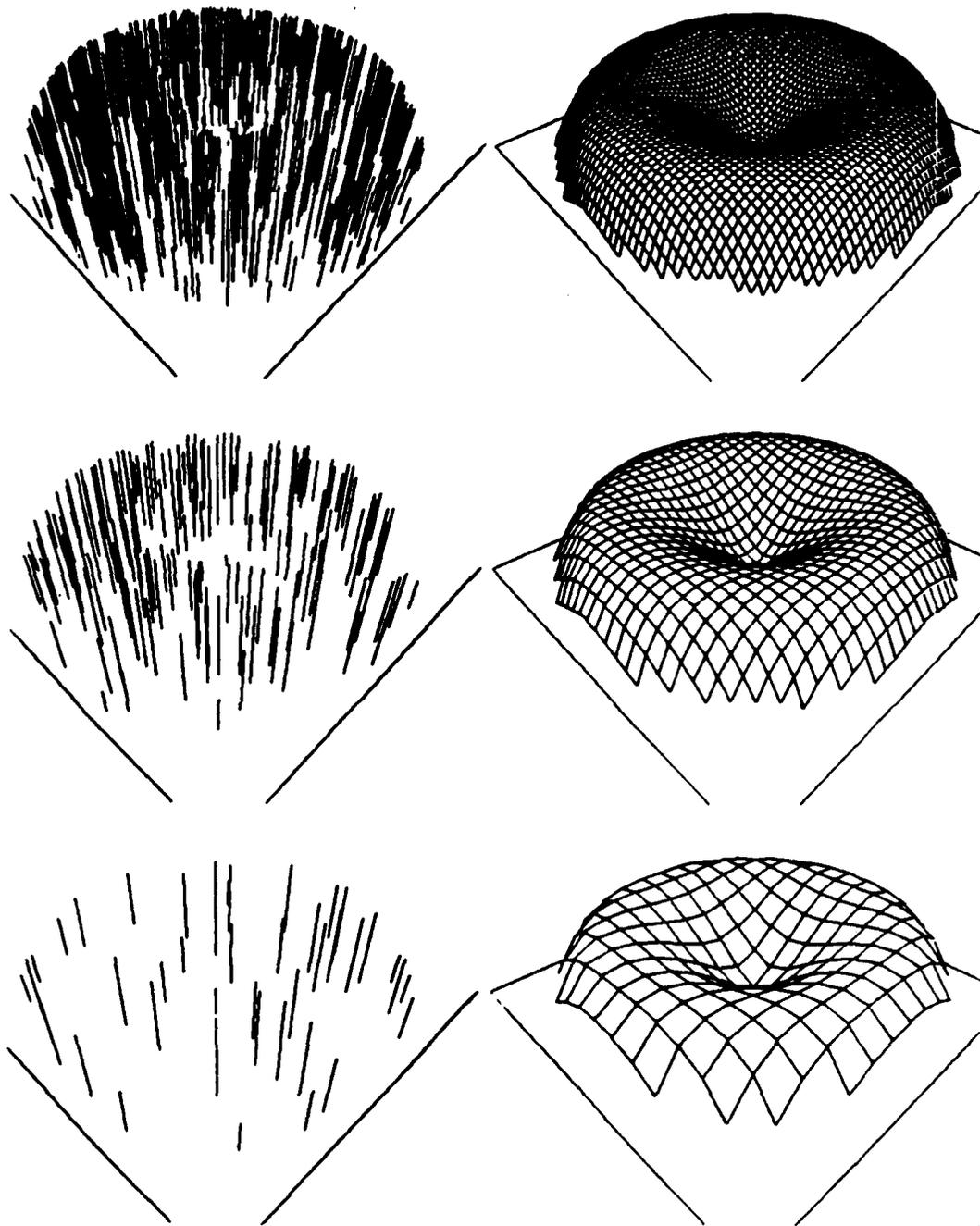
Figure 14. Reconstruction of a surface from depth constraints. (Grid dimensions:  $N_x^{h_1} = N_y^{h_1} = 17$ ,  $N_x^{h_2} = N_y^{h_2} = 33$ ,  $N_x^{h_3} = N_y^{h_3} = 65$ . Grid spacings:  $h_1 = 0.4$ ,  $h_2 = 0.2$ ,  $h_3 = 0.1$ . Constraint parameters:  $\alpha_i^{h_j} = 2.0/h_j$ . Computation: 24.25 work units.)
