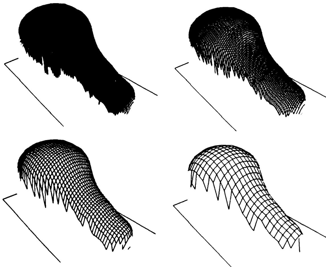
Figure 20. Reconstruction of a lightbulb from range data. (Finest grid dimensions:  $N_x^{h_4} \times N_y^{h_4} = 257 \times 281$ . Grid spacings:  $h_1 = 0.8$ ,  $h_2 = 0.4$ ,  $h_3 = 0.2$ , and  $h_4 = 0.1$ . Constraint parameters:  $\alpha_d^{h_j} = 0.2/h_j$ . Computation: 9.78 work units.)
