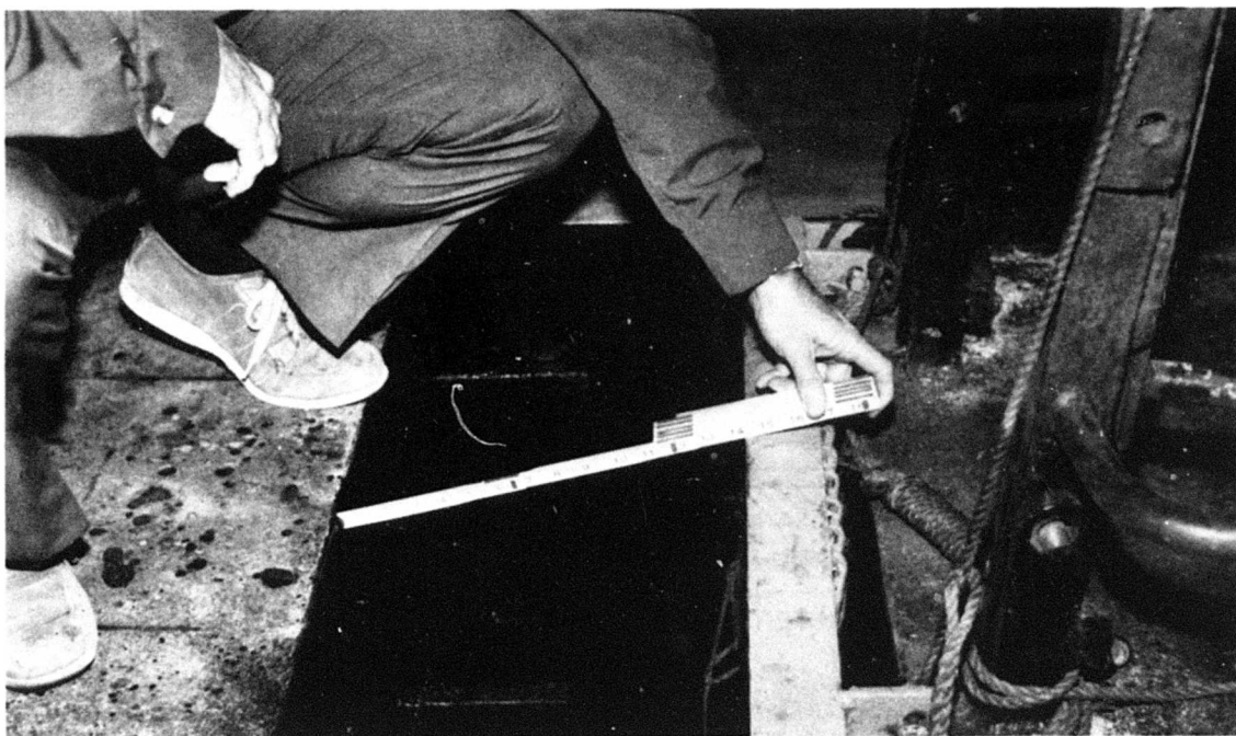
Figure 20 - Clearance between TCDF on Elevator's and Ship's Transom during Liftout
