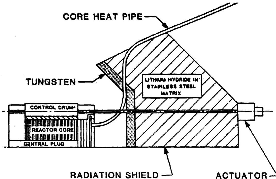
Figure 5. Axial cross-sectional diagram through the SP-100 reactor core and radiation shield.
