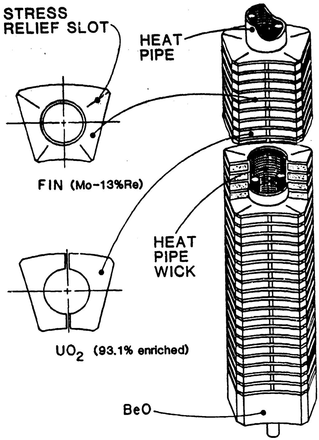
Figure 4. Drawing of the typical SP-100 fuel module.
