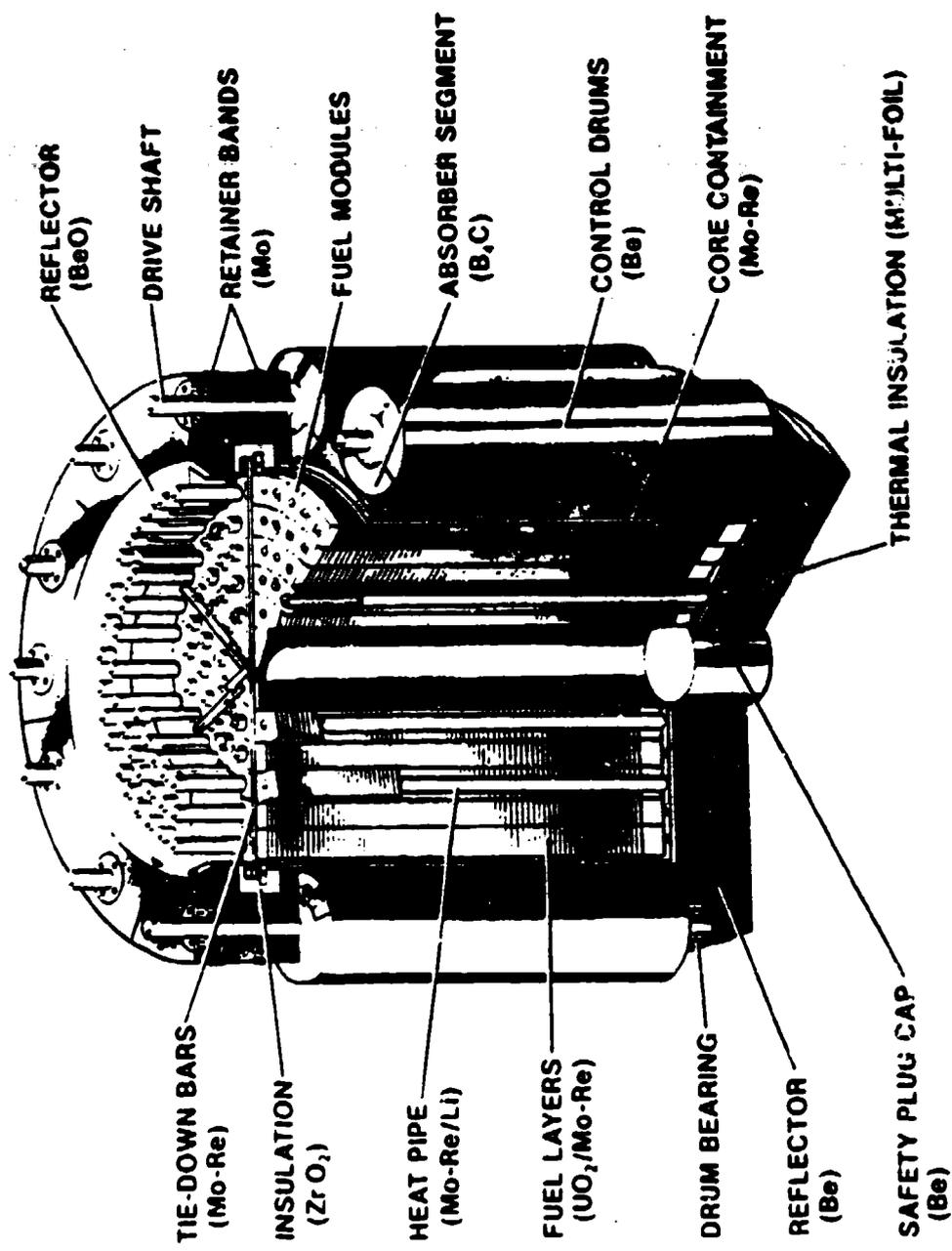
Figure 3. Cutaway drawing of the SP-100 reactor core.
