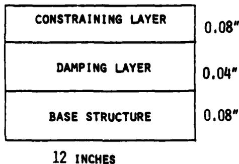
Fig. 1 First Damping System Model
