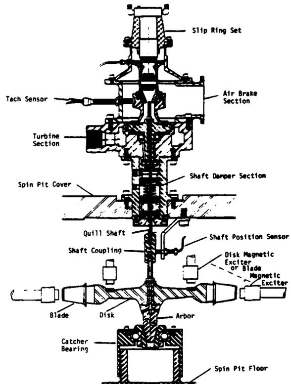
Fig. 6 Spin Test Assembly
