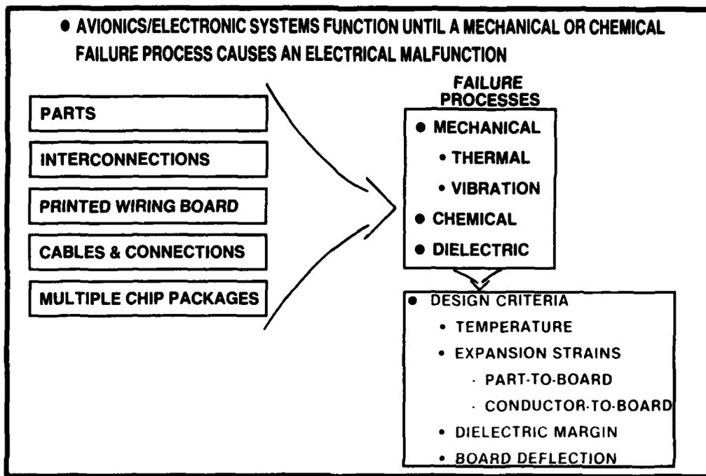
Fig. 11 -- Failure processes/criteria
