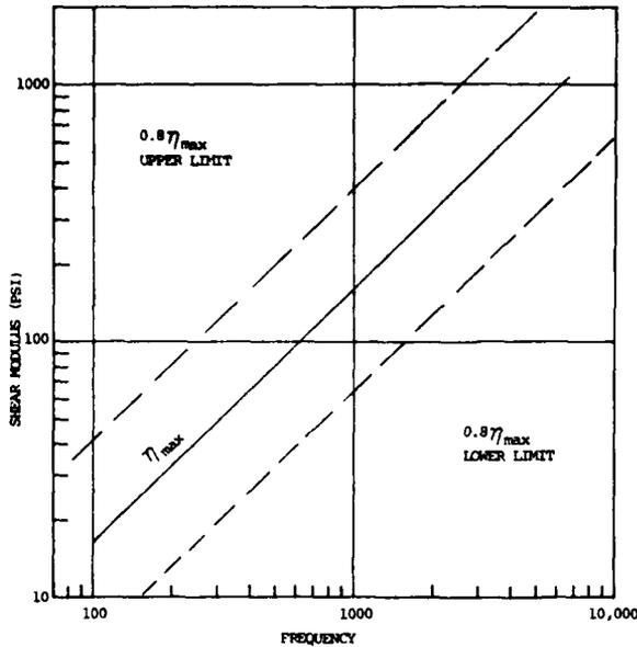
Fig. 7 Damping Material Shear Modulus VS Frequency For Maximum and 80% Maximum System Damping
