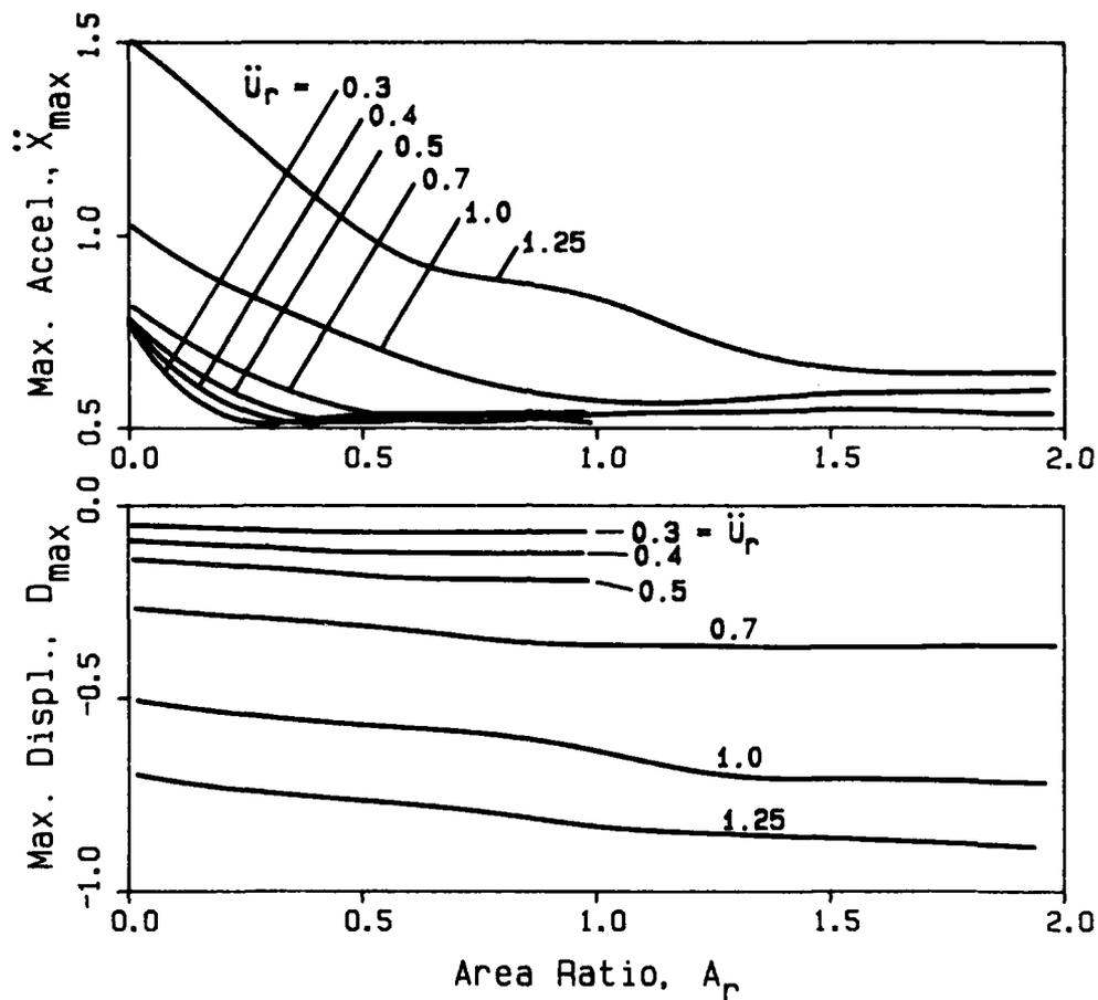
Figure 10. Determining Area Ratio for Maximum Shock Isolation
