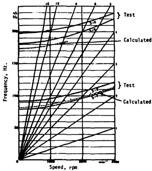
Fig. 7 Campbell Diagram for Free-Standing Low-Pressure Blade. Montoya [56]
