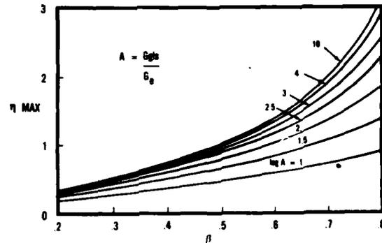
Fig. 7 - Maximum Loss Factor Versus  $\beta$  for Different Values of  $A$
