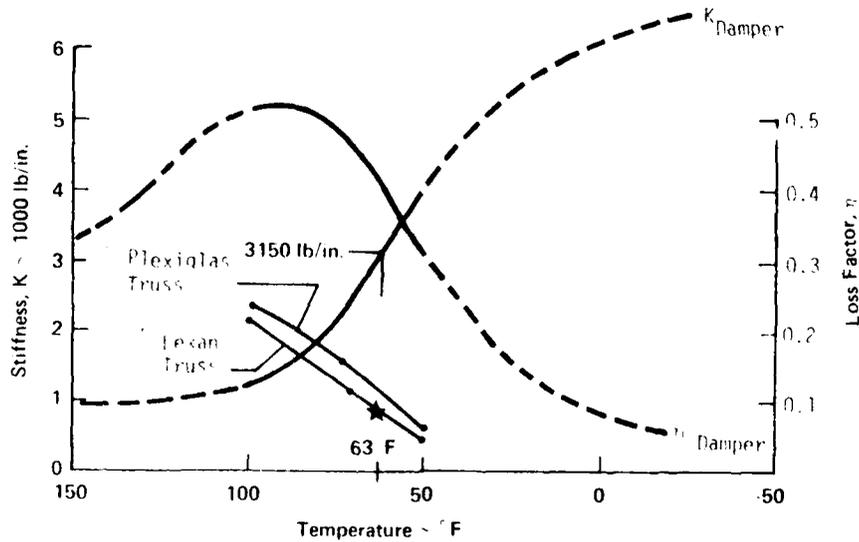
Fig. 11 - IGTA Damper Properties and Truss Loss Factor
