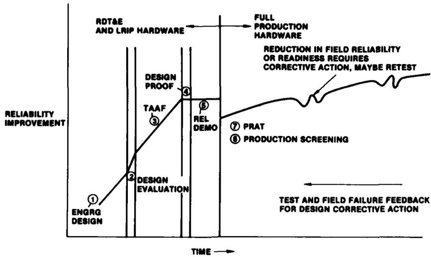
**FIGURE 5: RELIABILITY IMPROVEMENT TREND WITH ENVIRONMENTAL TESTING (IES)**
