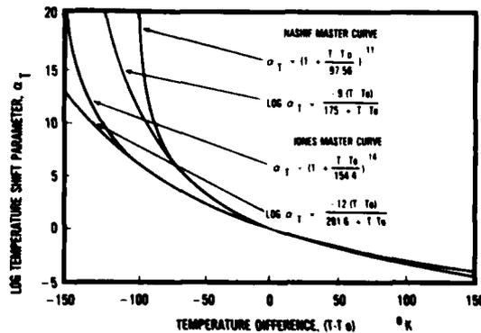
Fig. 1 - Temperature Shift Parameter Versus Temperature Difference
