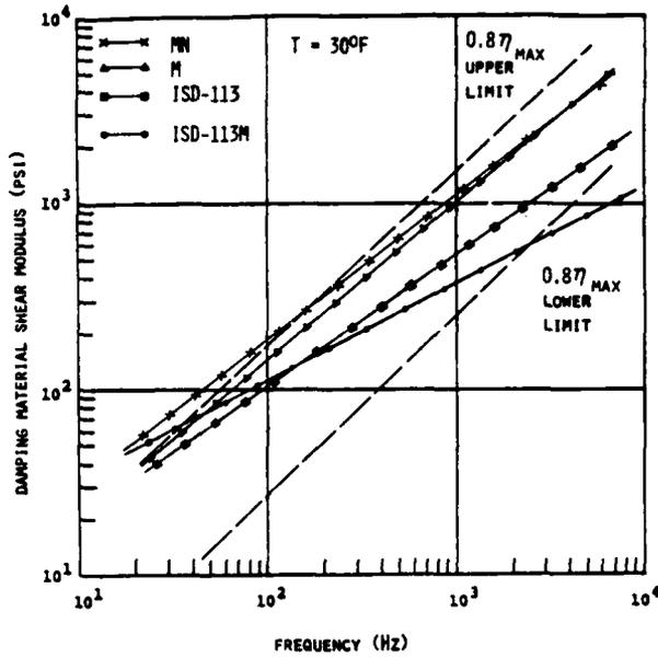
Fig. 4 - Shear Modulus - Frequency Characteristics For Maximum Damping
