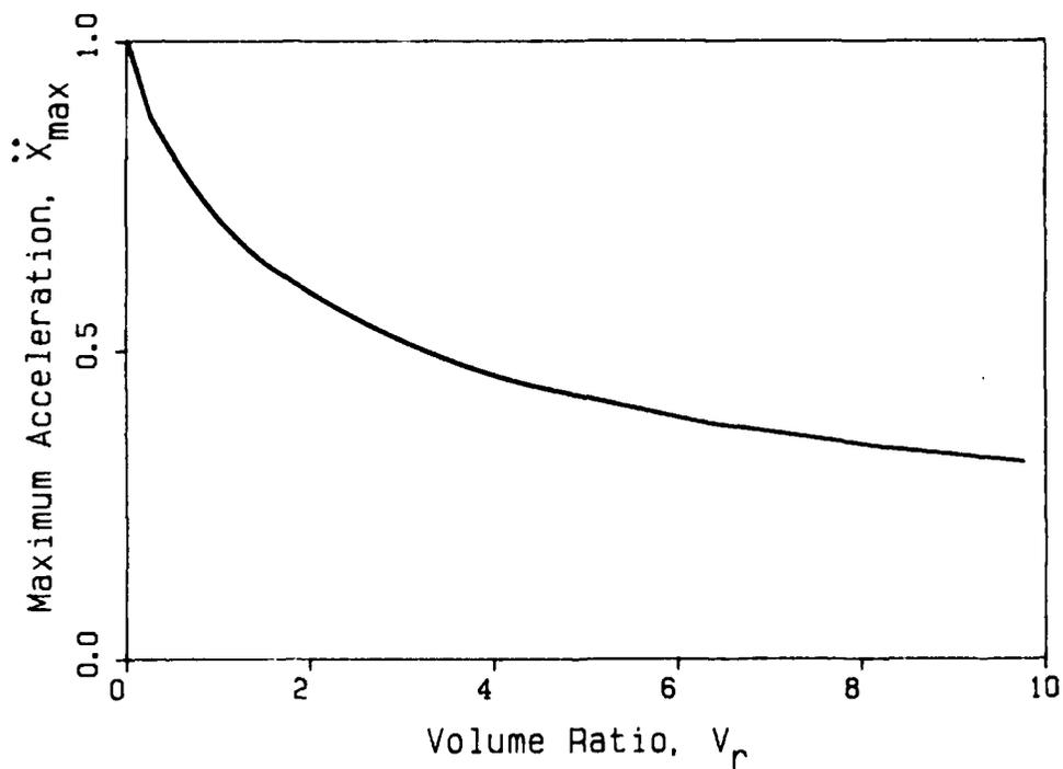
Figure 4. Change in Shock Isolation with Volume Ratio
