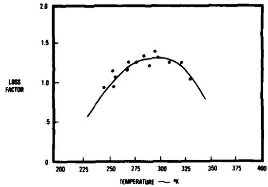
Fig. 6 - Loss Factor Versus Temperature
