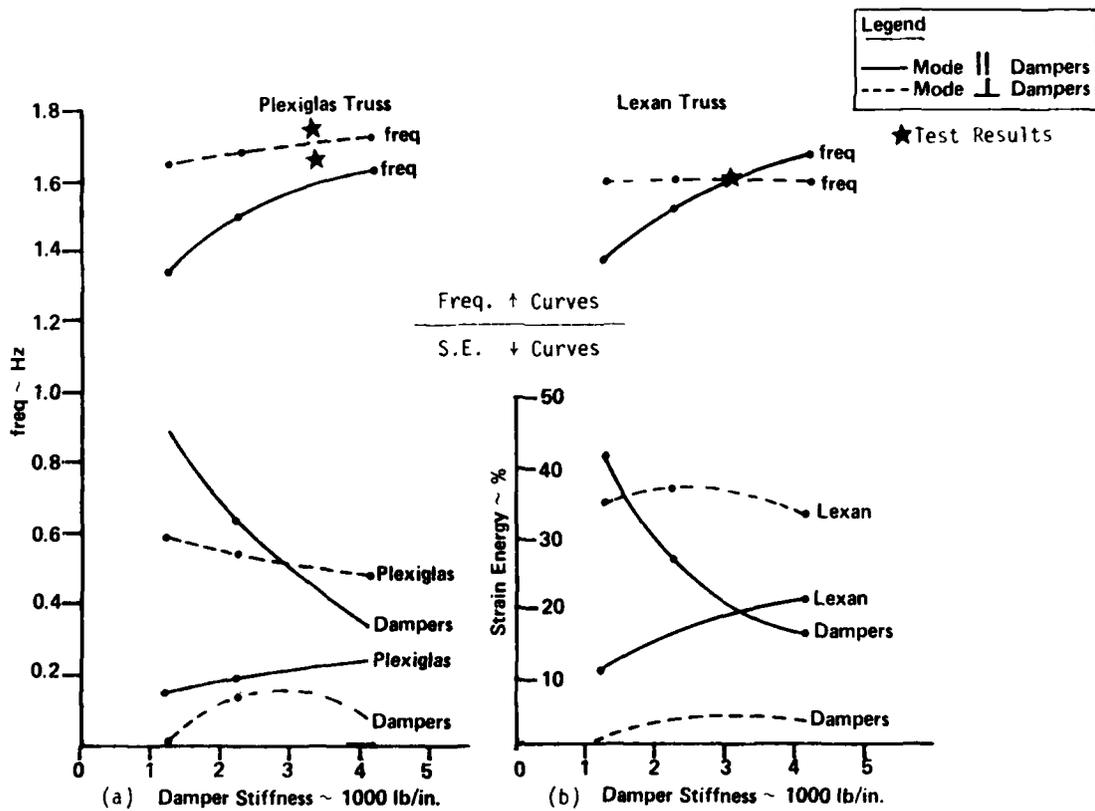
Fig. 10 - Vibration Analyses Results
