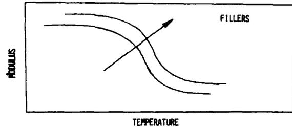
Fig. 9 The Effects of Fillers on Modulus
