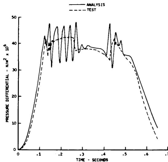
FIGURE 12 PRELIMINARY COMPRESSION PLCD VALVE ANALYSIS/TEST COMPARISON
