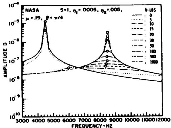
Fig. 15 Amplitude of HPFTP Blade Airfoil Mass VS Frequency of Excitation
