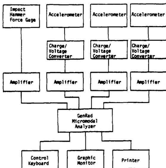
Fig. 2 - Block diagram of modal data acquisition system
