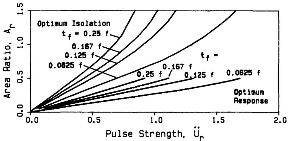
Figure 11. Optimum Area Ratios for Varying Pulse Strength
