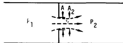
FIGURE 4 FLOW THROUGH AN ORIFICE
