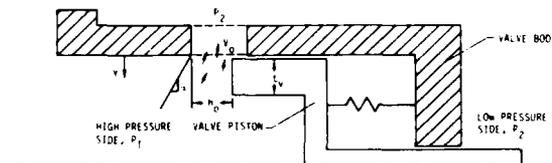
FIGURE 6 VALVE SCHEMATIC ILLUSTRATING ASSUMED FLUID STREAMLINES
