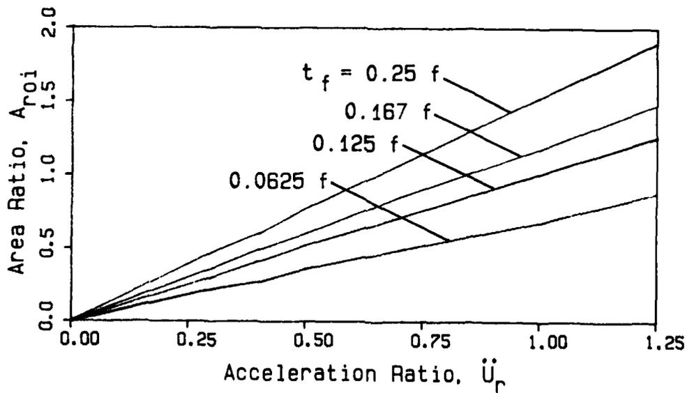
Figure 6. Area Ratios for Optimum Shock Isolation
