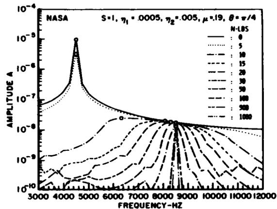
Fig. 16 Amplitude of HPFTP Blade Platform VS Frequency of Excitation
