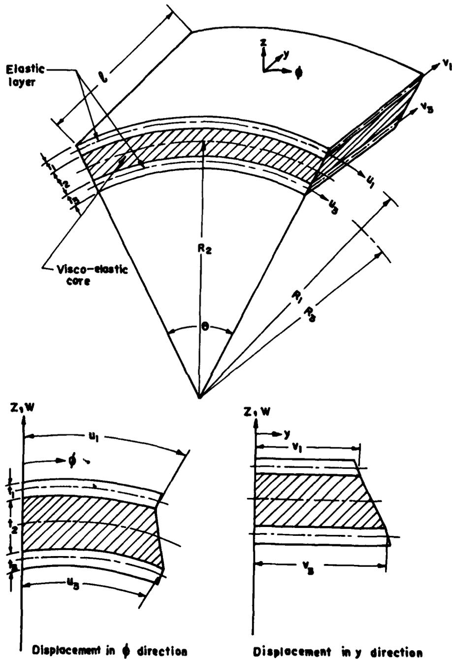
Fig. 1 Curved sandwich panel configuration and displacement pattern.
