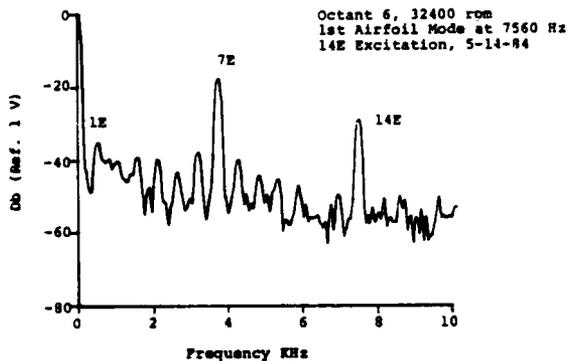
Fig. 14 Vibration Spectra-Airfoil Flex Mode-Production 0.56 Gram Dampers
