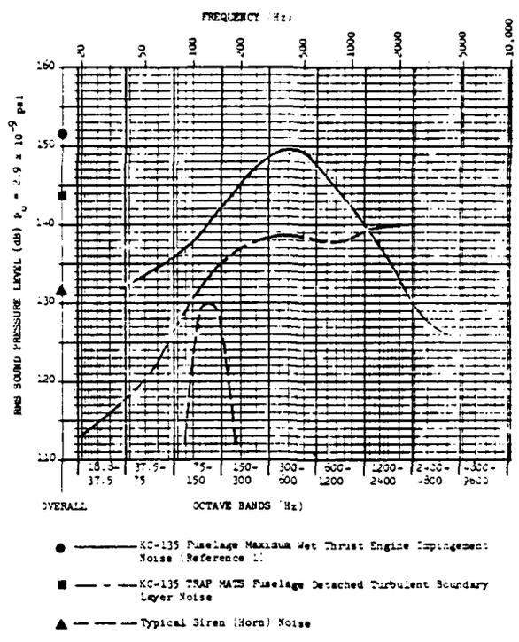
Fig. 10 - RMS sound pressure level versus frequency
