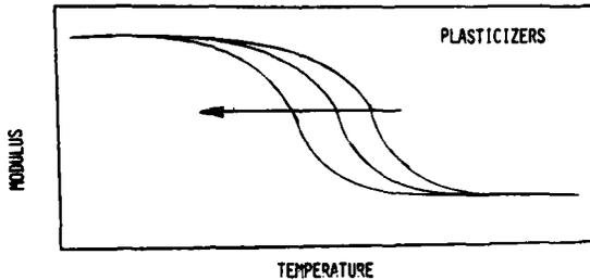
Fig. 13 The Effects of Plasticizers on Modulus
