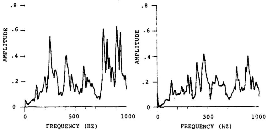
Fig. 23 - Response of test point 158 to sonic excitation before (left) and after damping installation
