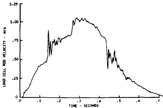
FIGURE 13 PRELIMINARY COMPRESSION PLCD VALVE VELOCITY TIME HISTORY
