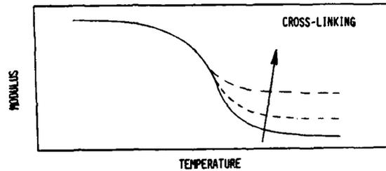
Fig. 12 The Effects of Cross-Linking on Modulus
