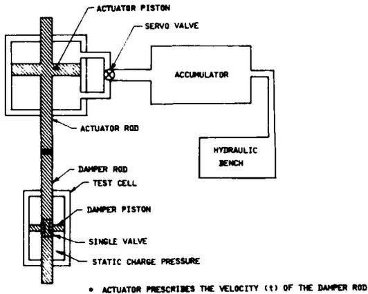
FIGURE 9 ACTUATOR DRIVEN PLCD SINGLE VALVE TEST FIXTURE
