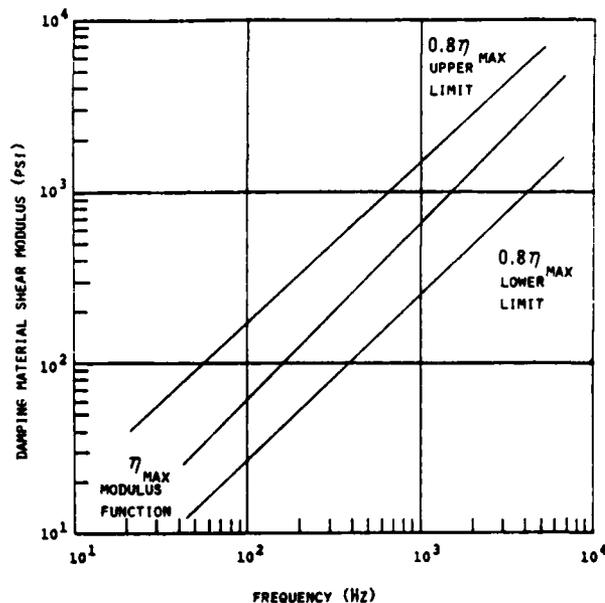
Fig. 3 Shear Modulus - Frequency Characteristics For Maximum Damping
