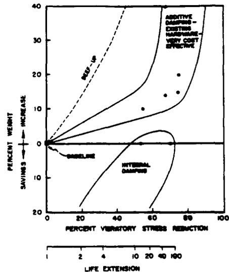
Fig. 25 - Comparison of approaches to extension of resonant fatigue life (Ref. [3])
