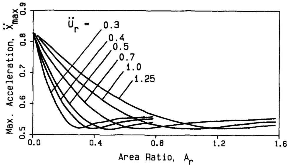
Figure 5. Shock Isolation for Different Area Ratios
