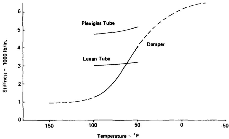
Fig. 9 - Stiffness Properties from Component Testing
