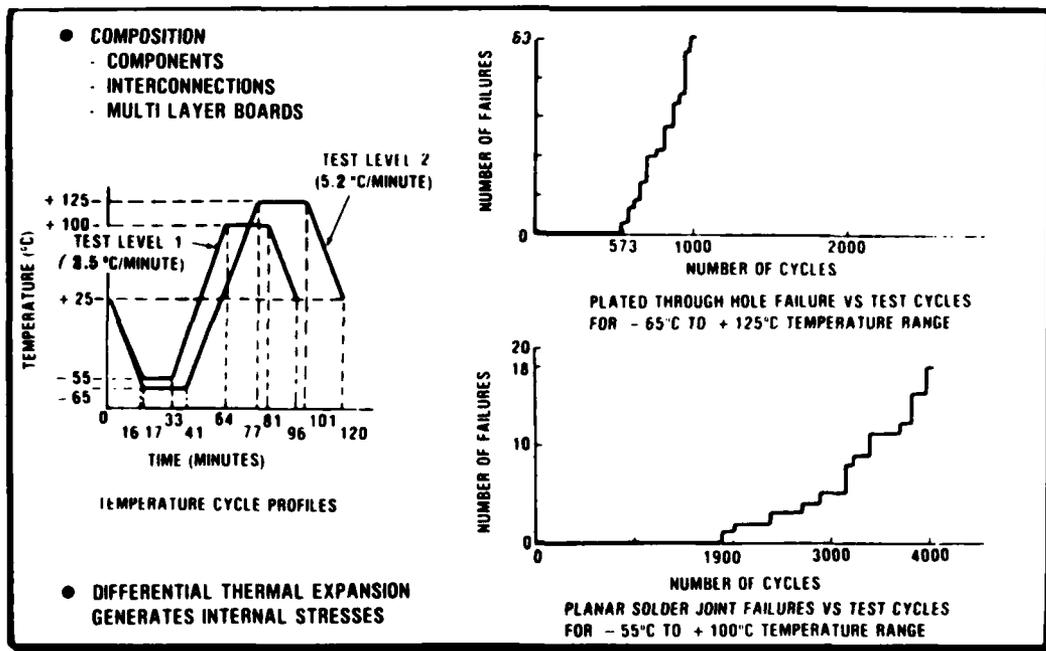
Fig. 8 — Fatigue failures in printed wire board assemblies
