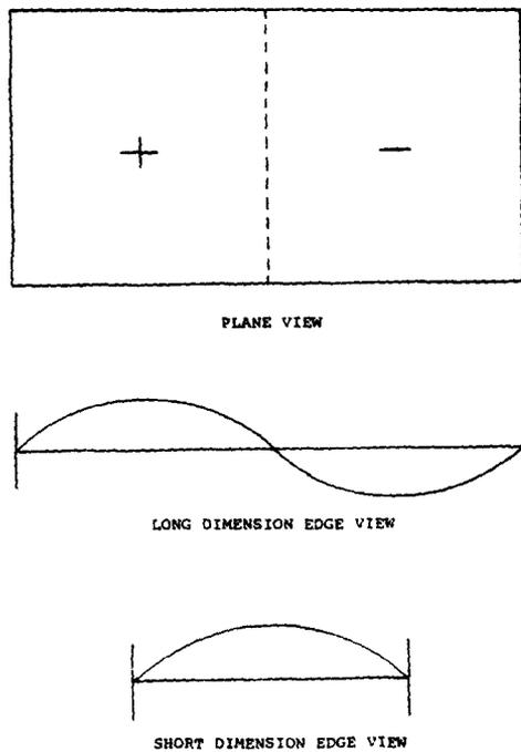
Fig. 15 - Modal model used for damping design
