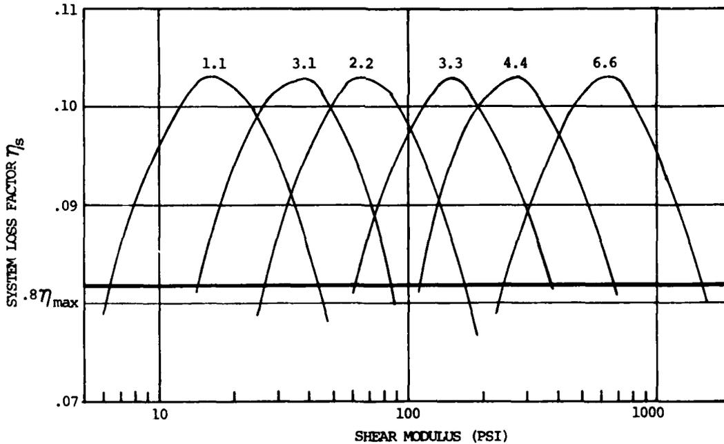
Fig. 6 System Loss Factor VS Damping Material Shear Modulus for Example Number 2.
