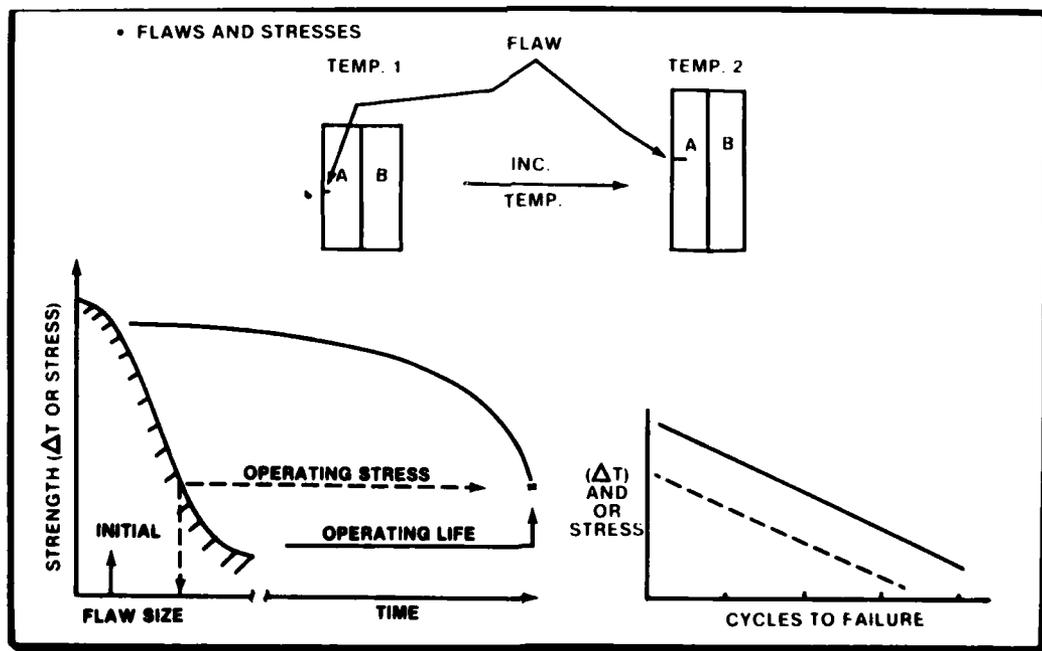
Fig. 4 — Relation between flaws and structural strength
