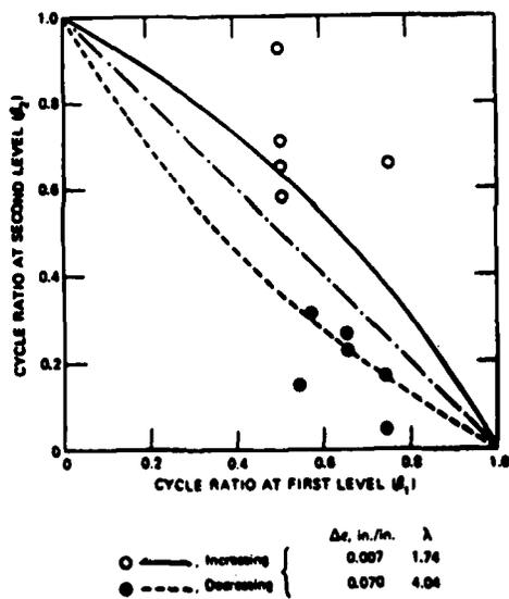
Fig. 18 Double Linear-Damage Concept. Conway et al [46]
