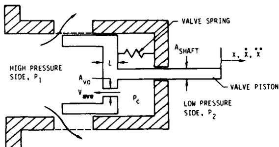
FIGURE 5 VALVE SCHEMATIC DETAILING VALVE DAMPING GEOMETRY
