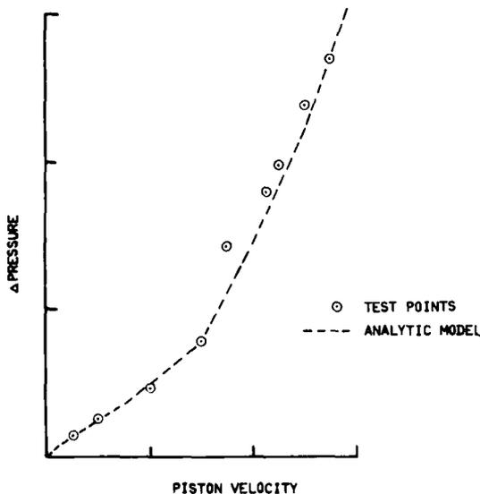
FIGURE 14 EXTENSION PLCD VALVE STEADY STATE BEHAVIOR
