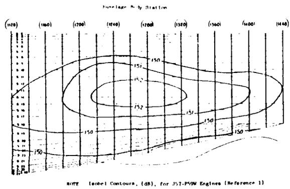
Fig. 9 - C/KC-135 aft fuselage maximum wet thrust engine impingement noise isobel contours
