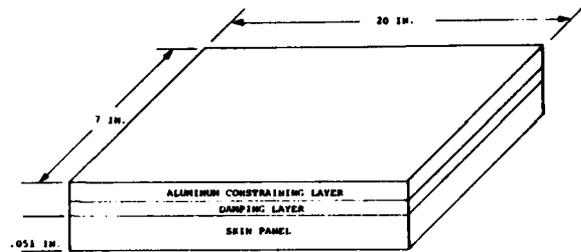
Fig. 14 - Constrained layer damping model
