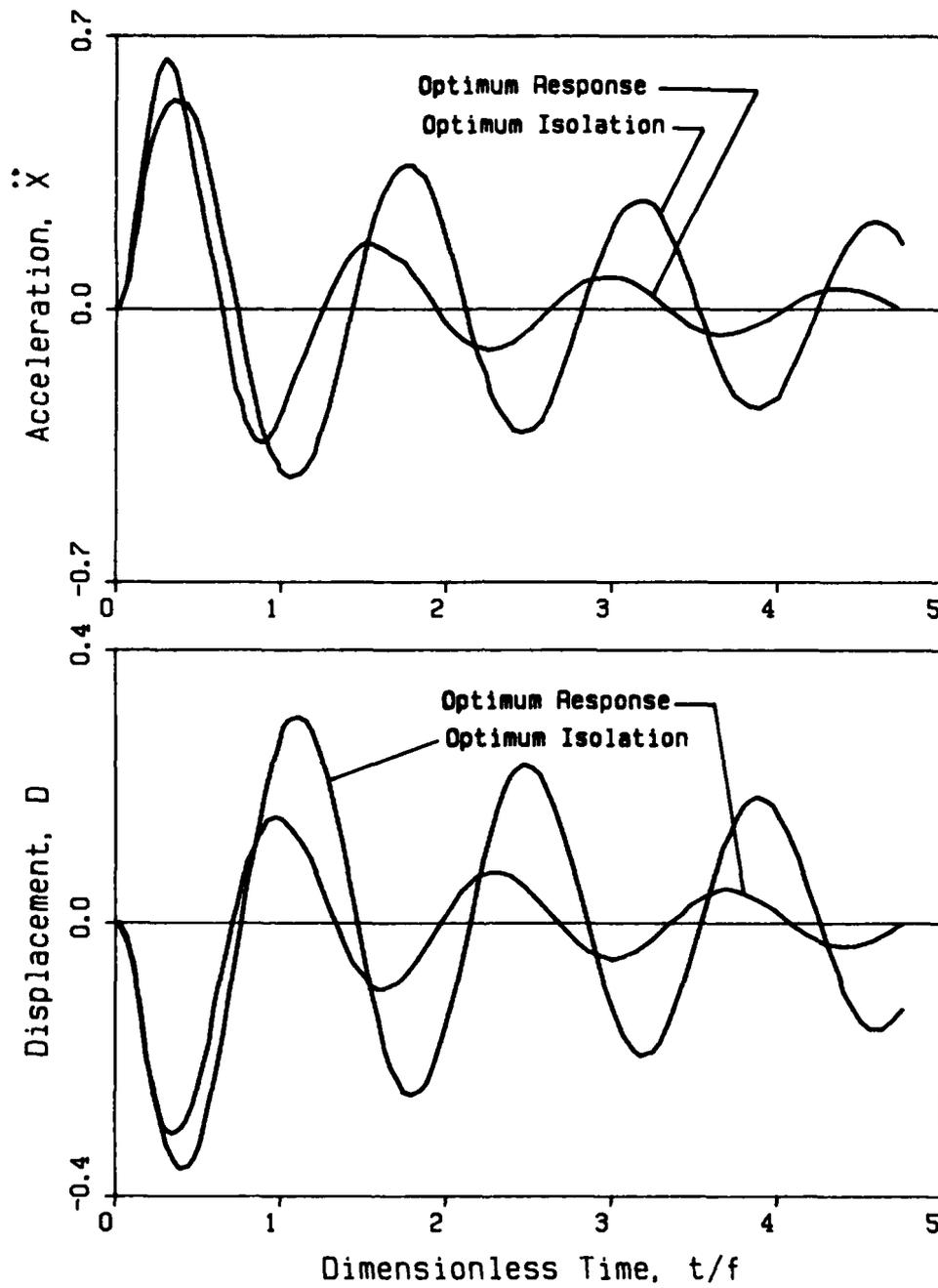
Figure 9. Use of Area Ratios for Optimum Response and Isolation
