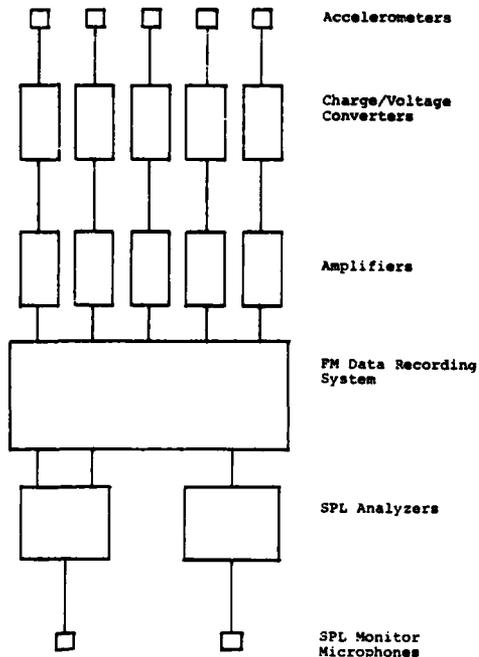
Fig. 12 - Block diagram of sonic response data acquisition system
