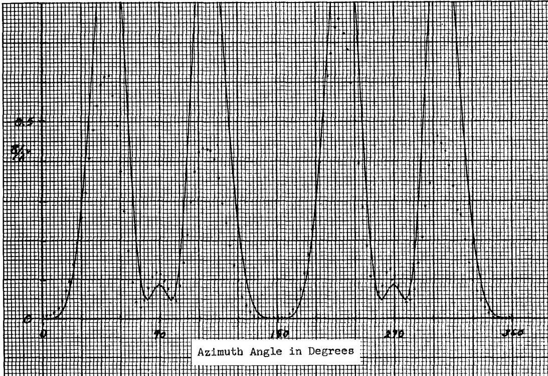
FIGURE 7. RADAR CROSS SECTION. Tungsten wire experimental (points) and theoretical (solid lines); 2l/\lambda = 0.992 , 2l/d = 834 .
