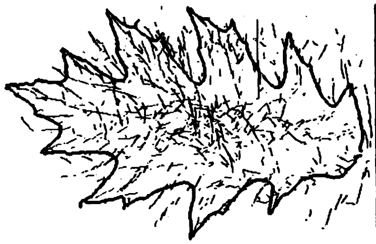
Figure 6-3. The Smoothed Local Symmetries of an oak leaf. The darker lines are the boundaries of the leaf and the finer lines are the axes of Smoothed Local Symmetries. Symmetries whose boundaries are close to one another compared to their lengths seem salient, whereas symmetries whose boundaries are far apart for their lengths seem like random junk in the analysis. This is perceptual evidence for locality of computation. (The vertical line represents a color boundary in the background on which the leaf was photographed.)
