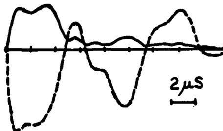
Figure 17. Lite Mike output (solid line) and current coil output (dashed line) as functions of time, taken at the spark gap.
