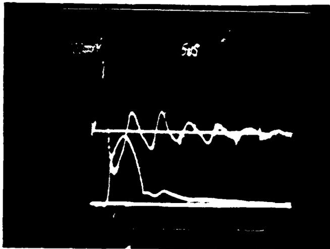
Figure 22. The voltage on the plasma cell (top trace) and the output of the Lite Mike with blue filter (bottom trace) for a 300 torr argon discharge. The main light pulse falls 4 microseconds after the first voltage pulse and the secondary pulse is 8 microseconds later.
