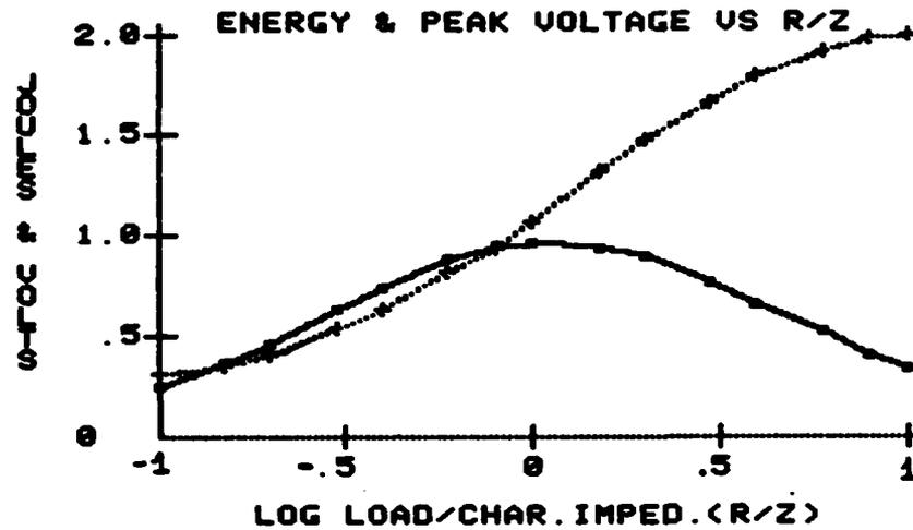
Figure 5. The fraction of total energy in the capacitors in the Blumlein network which is deposited in the load during the first pulse as a function of load ratio,  $R/Z$  (solid line) and the peak voltage.
