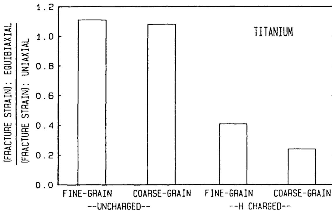
Fig. 2. The ratio of Hill equivalent strain to fracture in equibiaxial tension to that in uniaxial tension for Ti with either 0.015 or 0.030mm grain size and 25 or 1850 wt ppm H.
