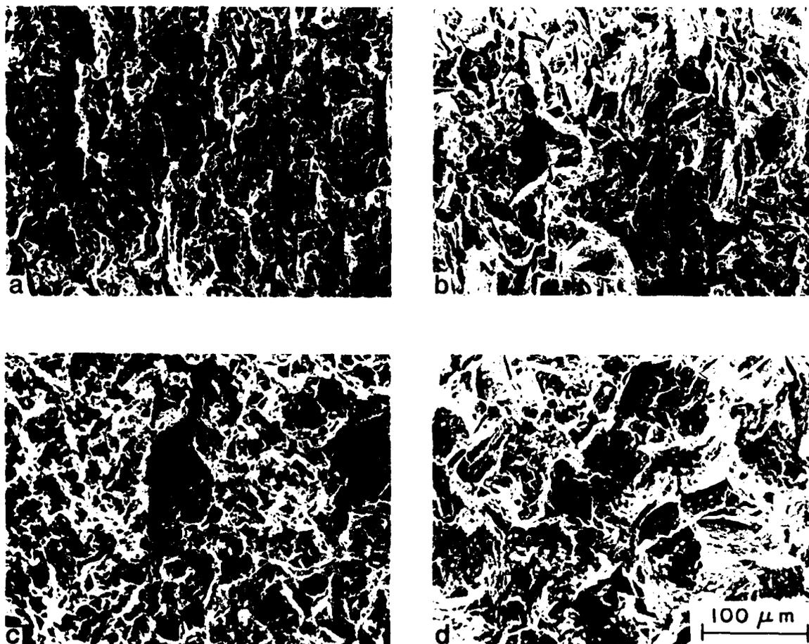
Fig. 3. Scanning electron fractographs of titanium containing 1850 wt ppm hydrogen and tested in uniaxial tension (a and b) or equibiaxial tension (c and d). Micrographs (a) and (c) are of fine-grain material while (b) and (d) are of coarse-grained sheets.
