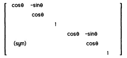
When the element matrices are assembled, the internal element forces,  $P_1$ ,  $Q_1$ ,  $Q_2$ ,  $P_2$ ,  $Q_3$ , and  $Q_4$  are canceled out by the internal element forces of adjoining elements. There may, however, be externally applied loads at the nodes, if this
