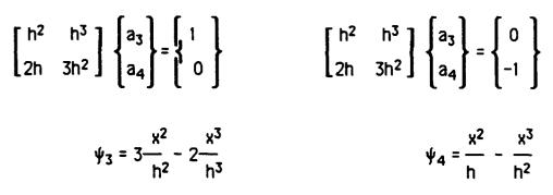
These interpolation functions are used in the above expressions for  $M_{ij}$ ,  $K_{ij}$ , and  $F_{ij}$  to derive the beam element matrices. The cross section of the element and the transverse loading function F(x,t) are allowed to vary linearly, but the modulus of elasticity is held constant.
