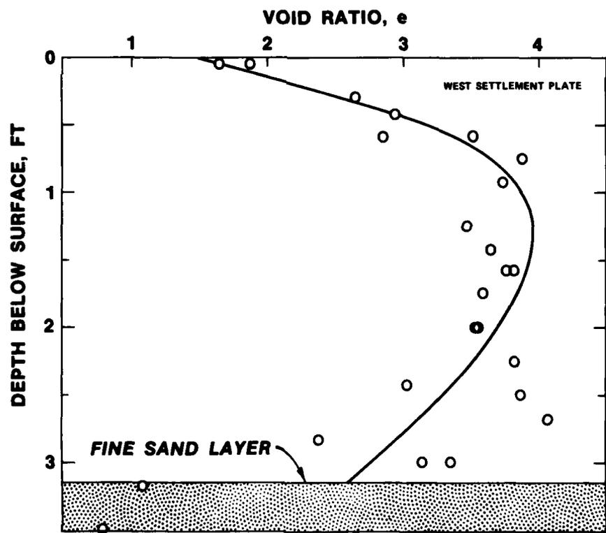
Figure 13. Void ratio profiles at Canaveral Harbor
