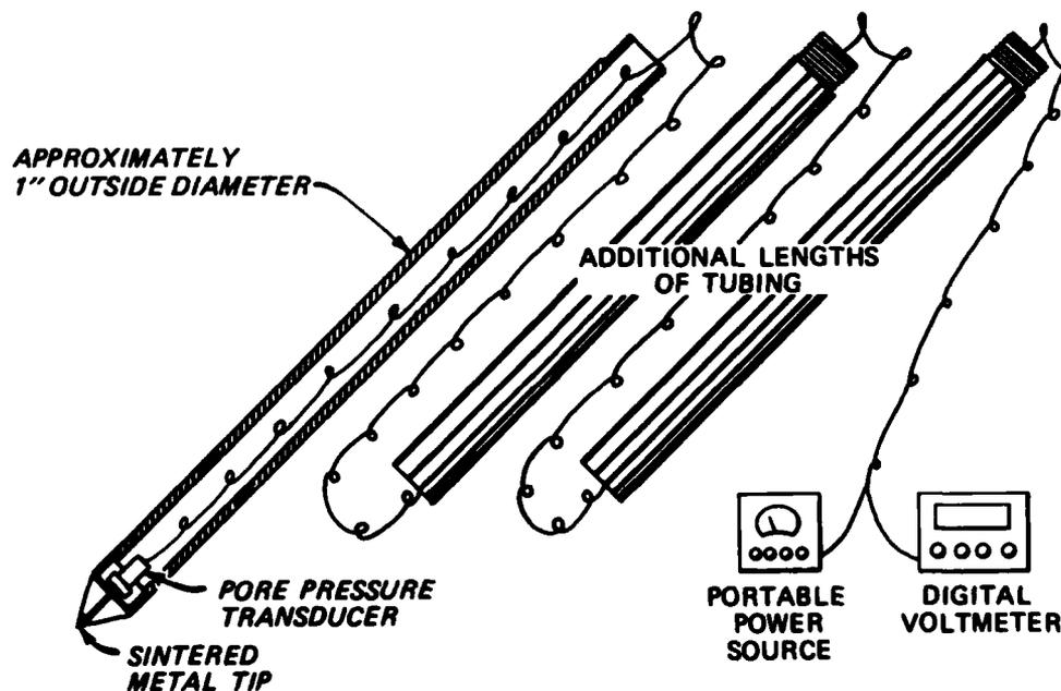
Figure E2. Typical pore pressure measurement probe
