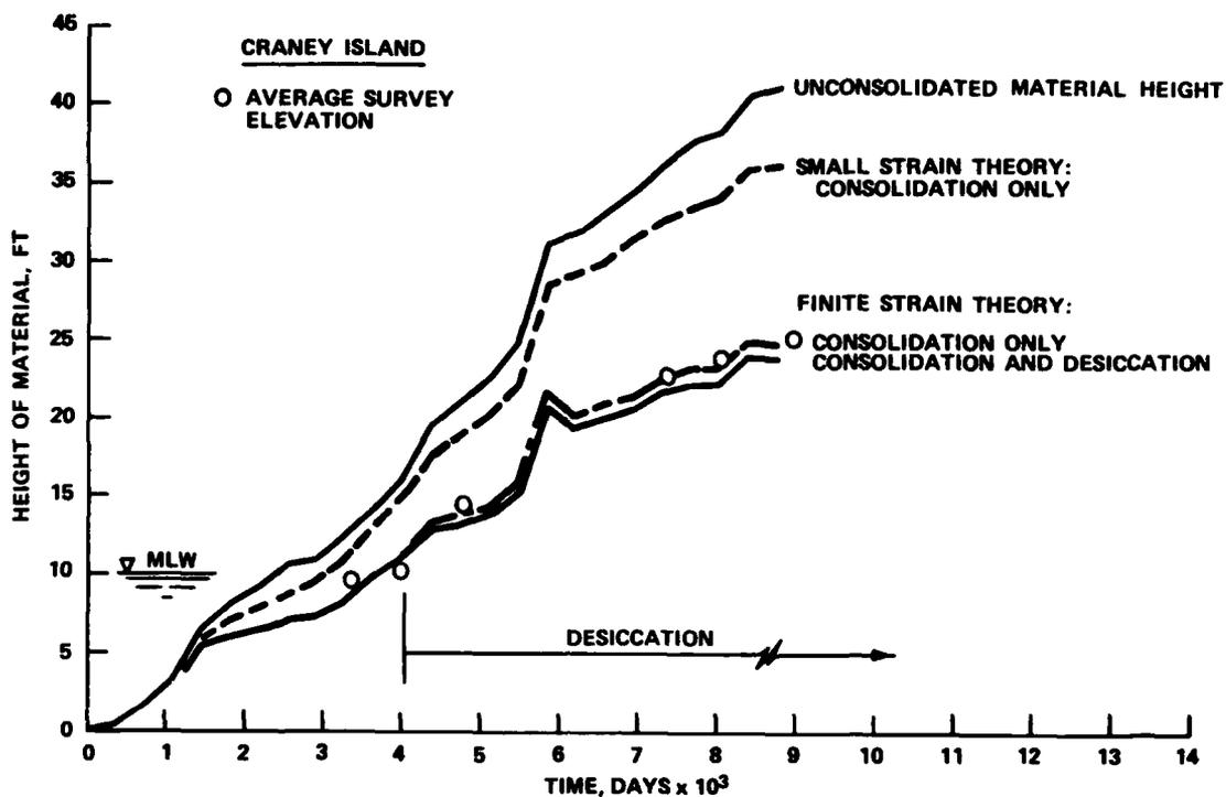
Figure 19. Measured and predicted material heights at Craney Island
