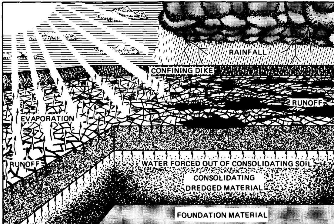
Figure 1. Water balance in a soil element of large areal extent suggested by the figure, the change in the amount of water contained in the upper crust over a finite period of time can be expressed as
