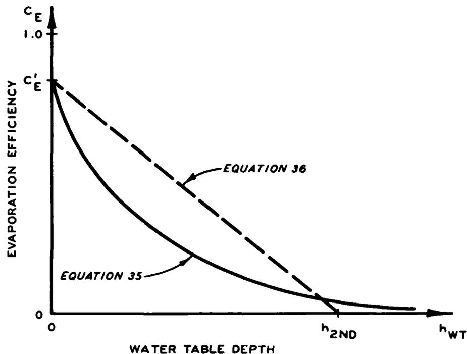
Figure 5. Soil evaporation efficiency as a function of water table depth
