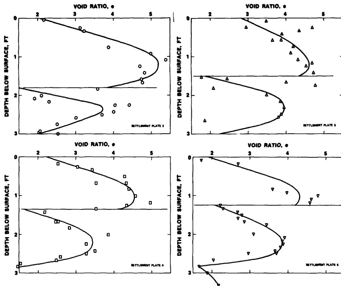
Figure 17. Void ratio profiles at Drum Island
