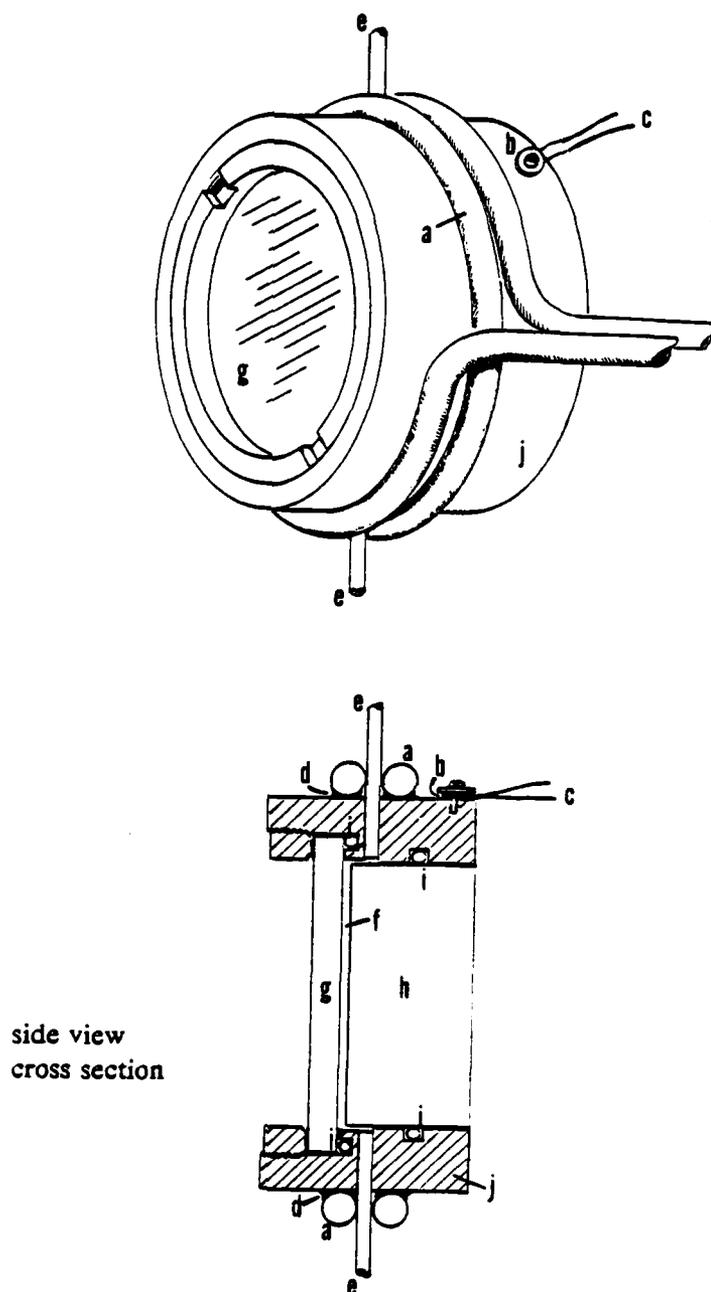
**Figure 15: Cooled Spectroscopy Cell**
