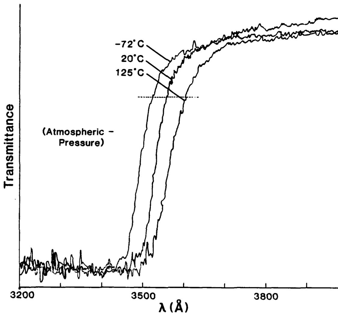
**Figure 17: CS<sub>2</sub> Spectrum Showing Red Edge Of Absorption Band**
