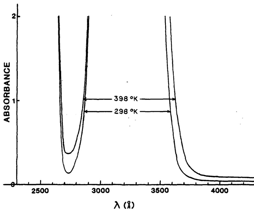
**Figure 18: Spectrum Of Liquid CS<sub>2</sub>**
