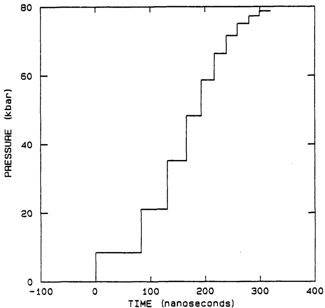
**Figure 8: Pressure History Of  $\text{CS}_2$  In A Typical Experiment**
