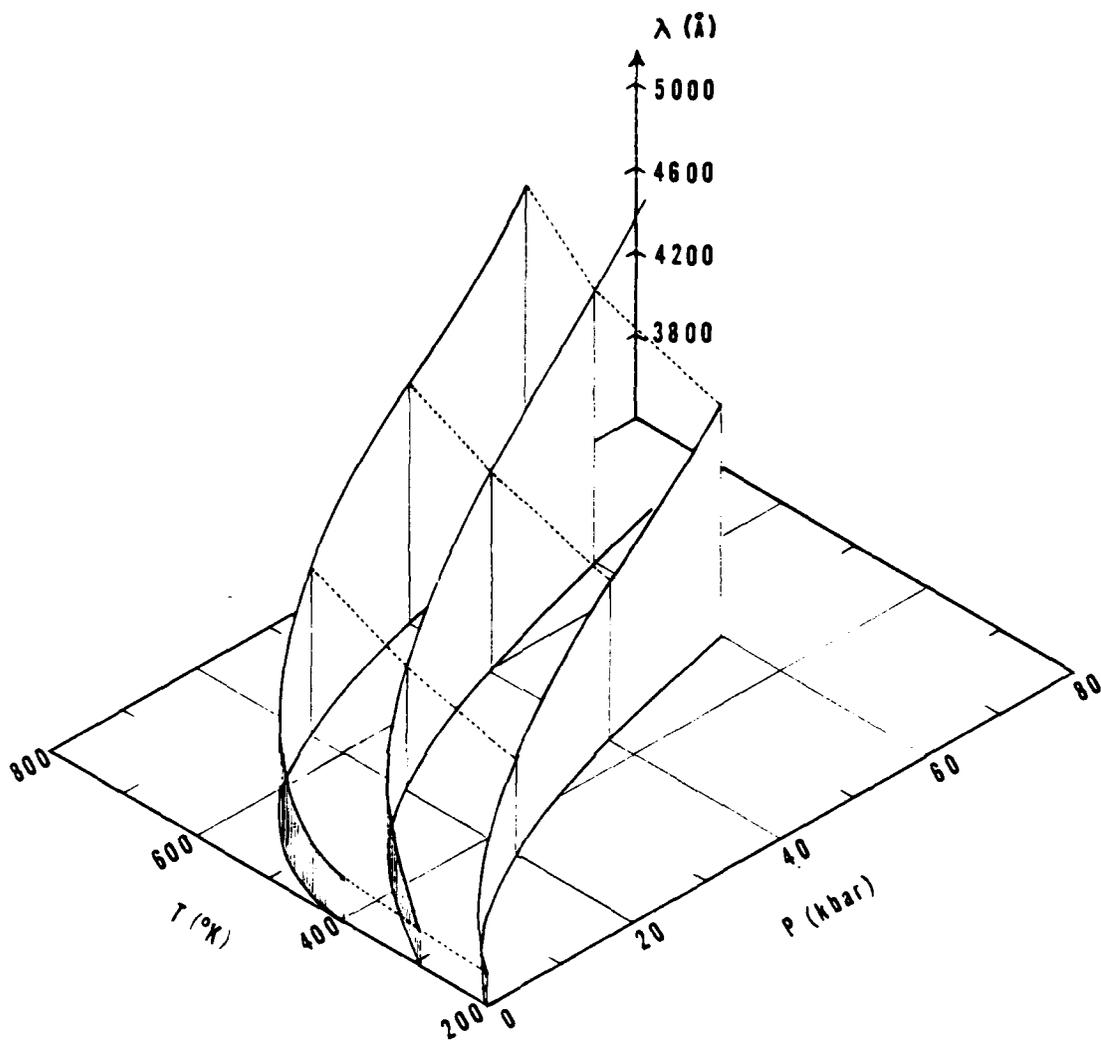
**Figure 2: P-T- $\lambda$  Surface For Liquid CS<sub>2</sub>**
