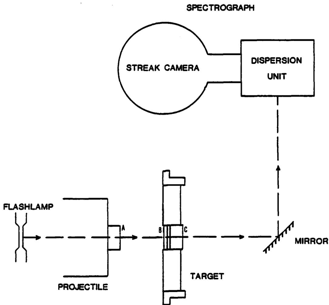
**Figure 3: Outline Of A Spectroscopy Experiment**
