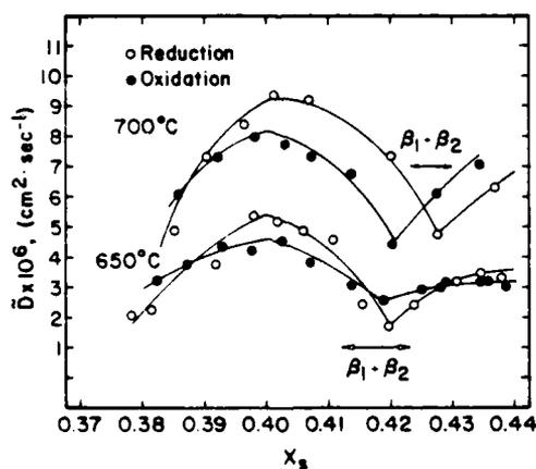
Fig. 6. Chemical diffusion coefficient,  $\bar{D}$  as a function of sulfur mole fraction for  $\beta\text{-Ni}_{3+x}\text{S}_2$  at  $650^\circ\text{C}$  and  $700^\circ\text{C}$ .
