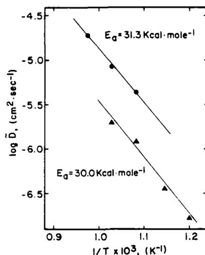
Fig. 8. Temperature dependence of the chemical diffusion coefficient,  $\bar{D}$  for  $\beta_1\text{-Ni}_{3-x}\text{S}_2$ . ●: Present study ( $X_s = 0.400$ ); ▲: Stoklosa and Stringer.<sup>9</sup>
