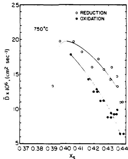
Fig. 7. Chemical diffusion coefficient,  $\bar{D}$  as a function of sulfur mole fraction for  $\beta\text{-Ni}_{1-x}\text{S}_2$  at 750°C.
