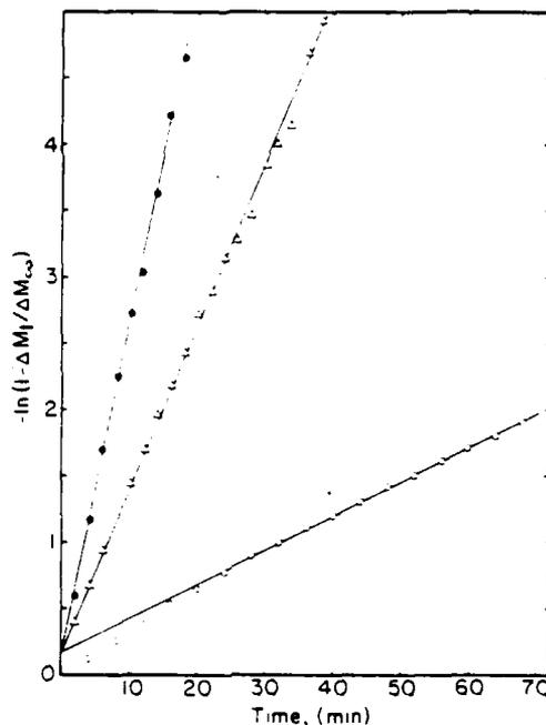
Fig. 5. Plots of  $-\ln(1 - \Delta M_t / \Delta M_\infty)$  vs.  $t$ . ●  $P_{H_2S} / P_{H_2} = 0.102$  to  $0.084$  at  $650^\circ\text{C}$ . △  $P_{H_2S} / P_{H_2} = 0.045$  to  $0.060$  at  $700^\circ\text{C}$ . □  $P_{H_2S} / P_{H_2} = 0.029$  to  $0.041$  at  $750^\circ\text{C}$ .
