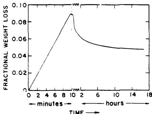
Fig. 6 Oxidation of  $\text{Ni}_3\text{S}_2$  in oxygen at 700°C
