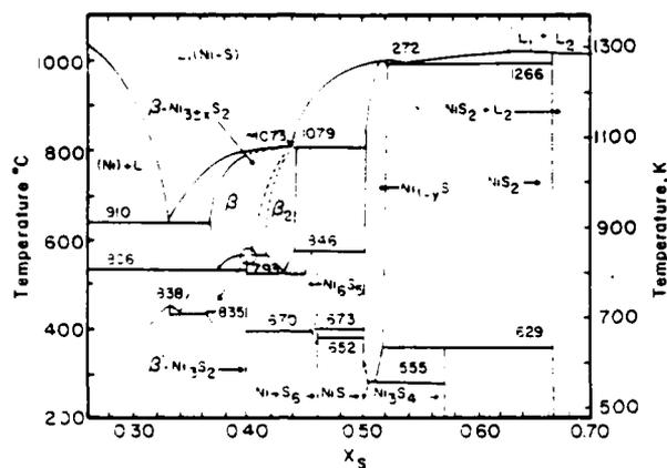
Fig. 1. Phase diagram for the nickel-sulfur system.<sup>4</sup>
