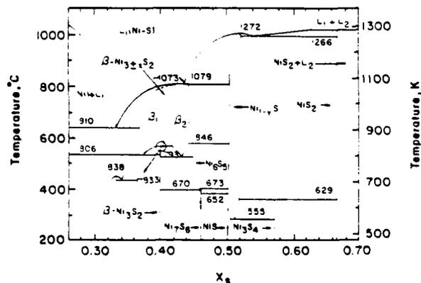
Fig. 2. Nickel-sulfur phase diagram, after Lin *et al.* (2)
