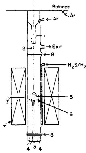
**Fig. 2.** Reaction chamber for the chemical diffusion and electrical conductivity measurements. (1): gas restriction to protect the balance from  $\text{H}_2\text{S}$ ; (2): platinum wire; (3): Pt/Pt-10% Rh thermocouple; (4): platinum lead wires for electrical conductivity measurement; (5): platinum mesh basket; (6): sample for electrical conductivity measurement; (7): furnace; (8): O-ring joint.
