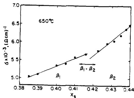
Fig. 9. Electrical conductivity as a function of sulfur mole fraction for  $\beta$ - $\text{Ni}_3\text{S}_2$  at 650°C.
