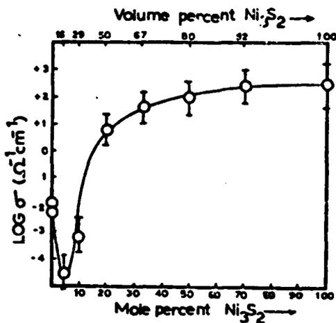
FIG. 2. Electrical conductivity as a function of composition of NiO-Ni<sub>3</sub>S<sub>2</sub> mixtures at 600 °C.
