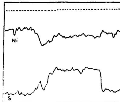
FIG. 5. Concentration profile of Ni and S across the Ni<sub>3</sub>S<sub>2</sub> particle shown in Fig. 6.
