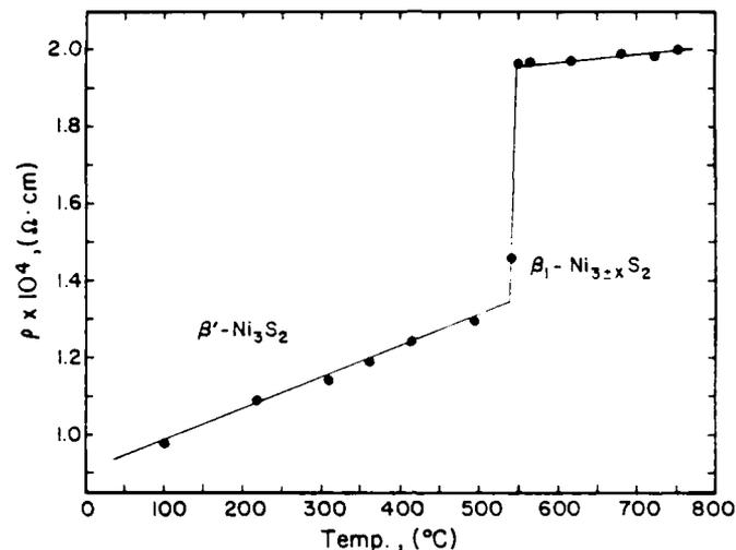
Fig. 10. Electrical resistivity as a function of temperature for  $\text{Ni}_3\text{S}_2$ .
