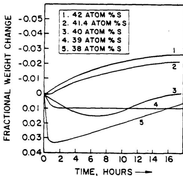
Fig. 1. Oxidation of  $\text{Ni}_x\text{S}_y$  in oxygen at  $700^\circ\text{C}$  for various compositions.
