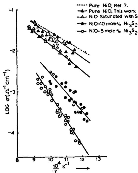
FIG. 1. Electrical conductivity as a function of reciprocal temperature for various NiO- $\text{Ni}_3\text{S}_2$  compositions.
