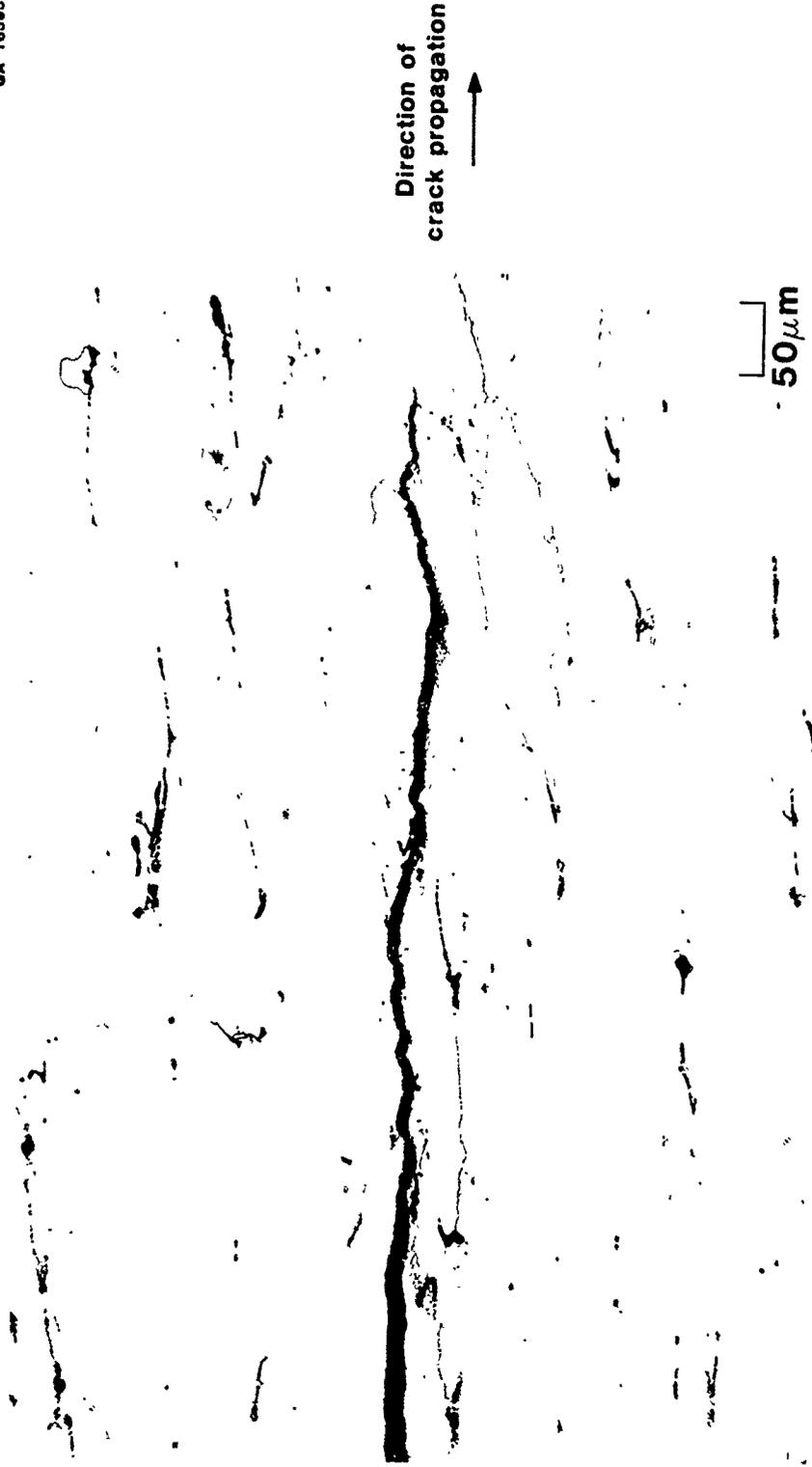
Photomicrograph of tip of the crack in DCB SCC specimen from sample 504412 (7075-T651 plate)
