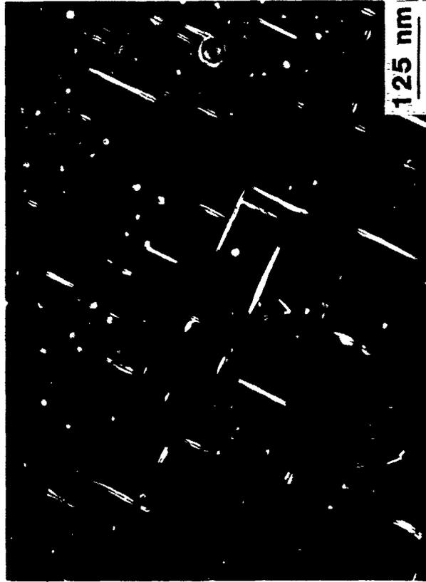
(a) Dark field showing  $\delta'$  and  $\theta'$ -like precipitates
