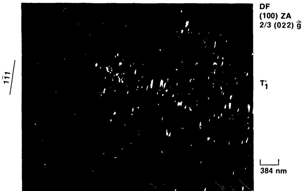
(b) Dark field image showing  $T_1$  along  $(1\bar{1}1)$ .
