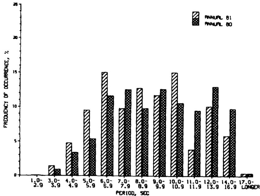
Figure 18. 1981 and 1980 wave period distributions for gage 625
