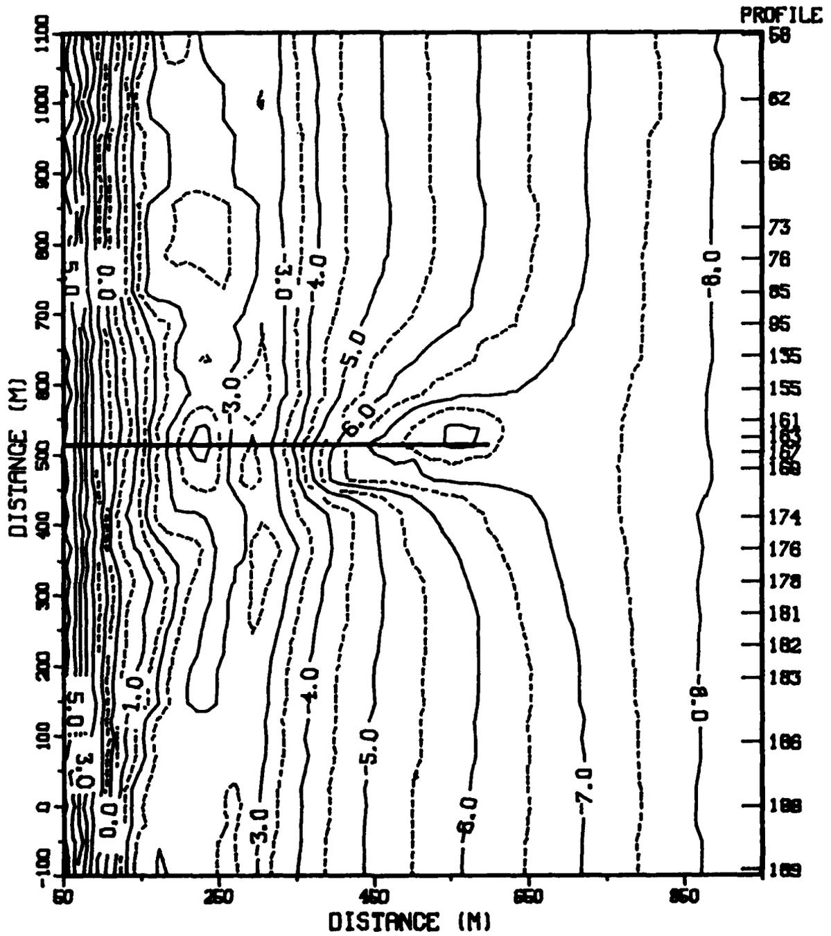
Figure 41. Contour diagram of FRF bathymetry, 3 November 1981
