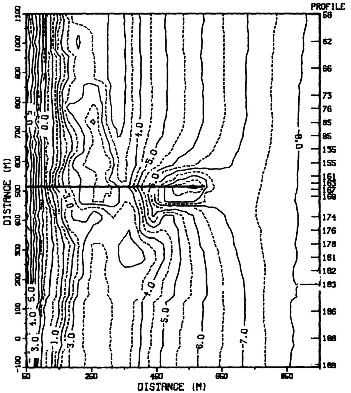
Figure 42. Contour diagram of FRF bathymetry, 16 November 1981
