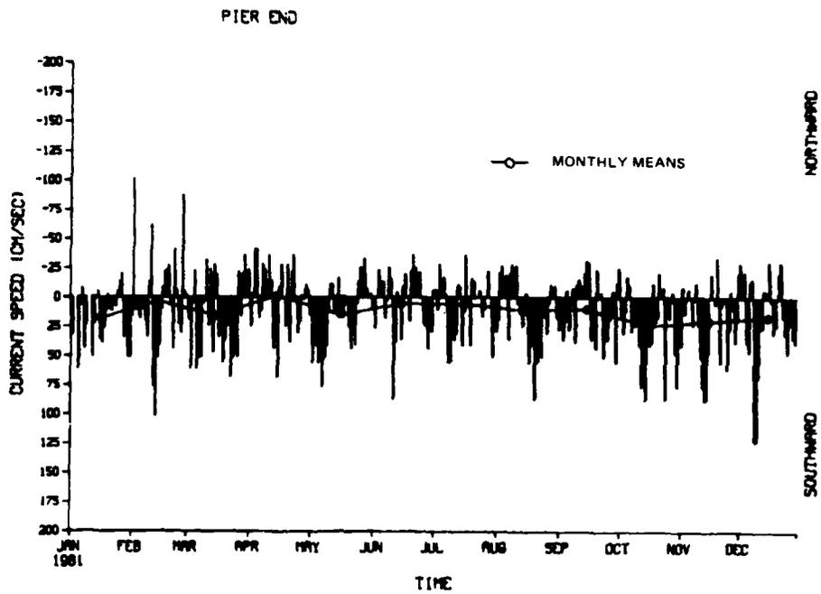
Figure 23. 1981 longshore surface current speed and direction at seaward end of FRF pier
