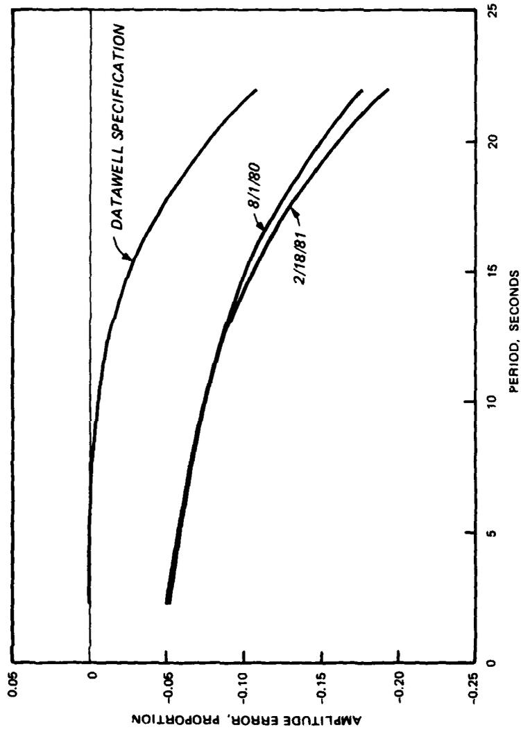
Figure A1. Waverider 66967 calibrations, NOAA Engineering Support Office
