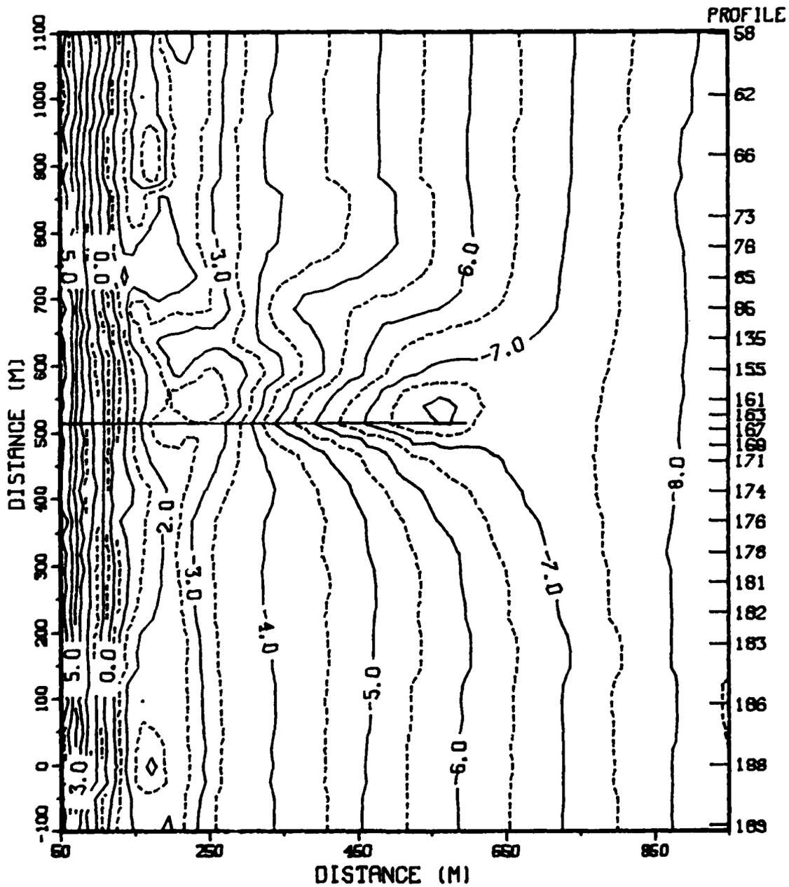
Figure C4. FRF bathymetry for 17 July 1981, contours in meters
