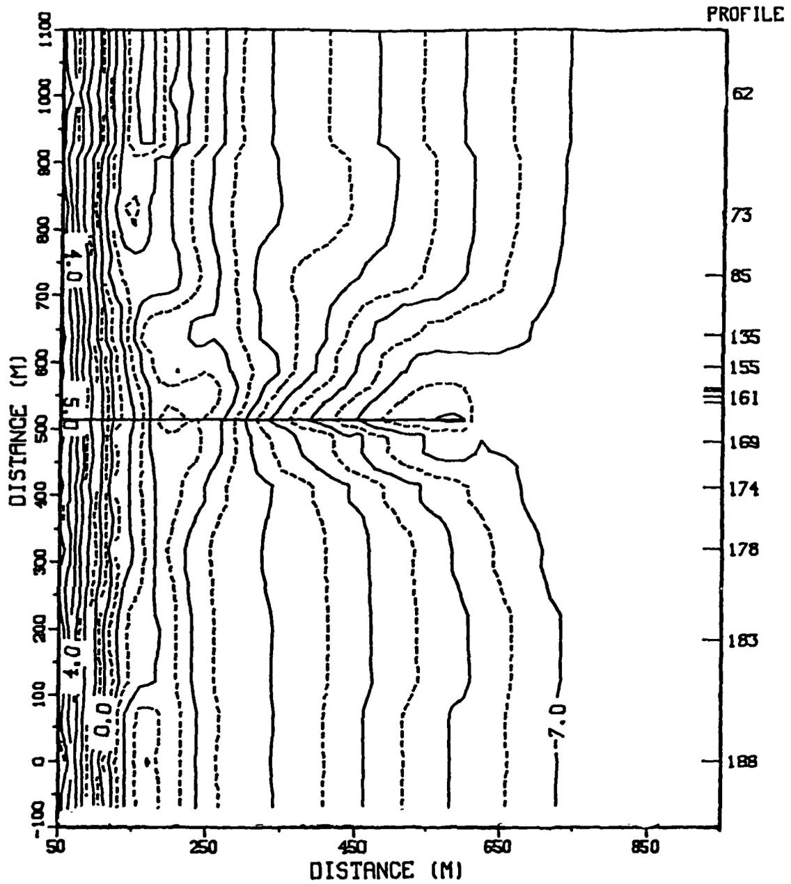
Figure C5. FRF bathymetry for 4 August 1981, contours in meters
