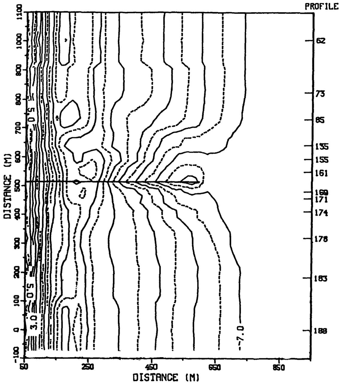
Figure C3. FRF bathymetry for 2 July 1981, contours in meters
