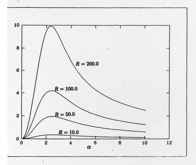
Graph of the coefficient of  $-\epsilon \bar{\varsigma}$  in  $\frac{\partial \sigma}{\partial l_1}(l_1=0)$  versus  $\alpha$  for R=10.0, 50.0, 100.0, 200.0. The amplitudes decay to zero for large  $\alpha$ . As R approaches  $27\pi^4/4$ , the peak amplitude proaches infinity and the location of the peak approaches  $\alpha=\pi/\sqrt{2}$ .
