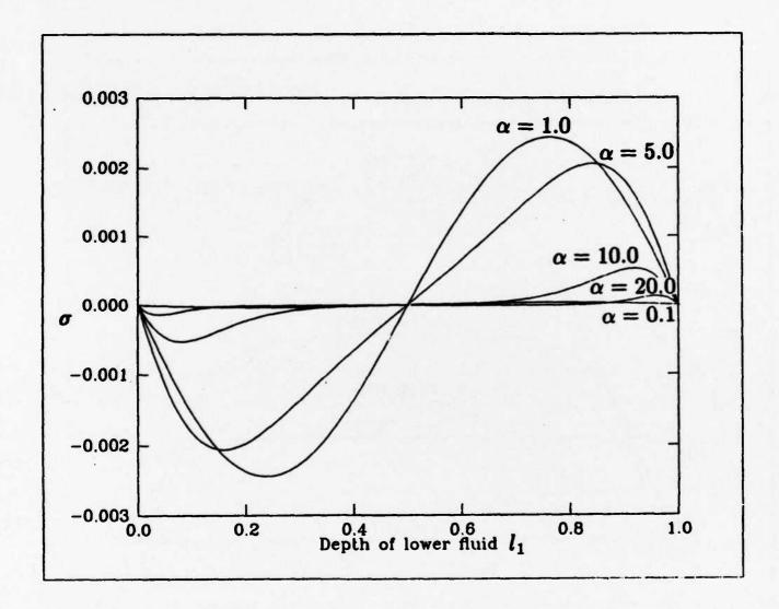
Graph of  $\sigma$  versus  $l_1$ , the depth of the lower fluid.  $\alpha_1\Delta T^*=0.001,\,R=1,$   $\tilde{\varsigma}=1,\,\alpha=0.1,1.0,5.0,10.0,20.0.$
