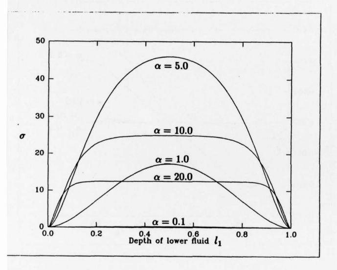
Graph of  $\sigma$  versus  $l_1$ , the depth of the lower fluid.  $\alpha_1\Delta T^*=0.001$ . R=1,  $\bar{\tau}=1,~\alpha=0.1,1.0,5.0,10.0,20.0$ .
