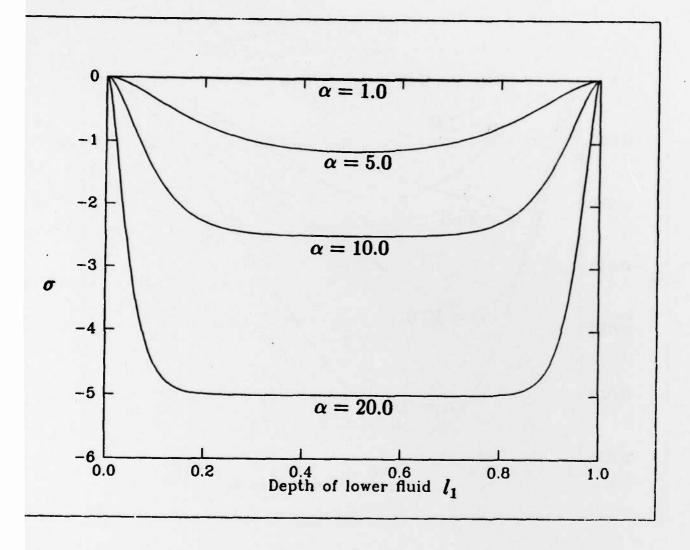
Graph of  $\sigma$  versus  $l_1$ , the depth of the lower fluid.  $\alpha_1\Delta T^+=0.001,\,R=1,\,\bar{S}=1,\,\alpha=0.1,1.0,5.0,10.0,20.0.$
