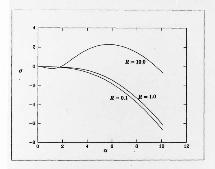
Graph of  $\sigma$  versus  $\alpha$ .  $\bar{r}=0.1$ ,  $\bar{\zeta}=100.0$ ,  $\bar{\beta}=1.0$ ,  $\bar{S}=10.0$ ,  $l_1=0.05$ , R=0.1,1.0,10.0. Fluid 1 is the less dense fluid. At R=0.1 and 1.0, the arrangement is linearly stable for all  $\alpha$ . As R increases, the arrangement will become less stable. For example, at R=10.0, the arrangement is unstable.
