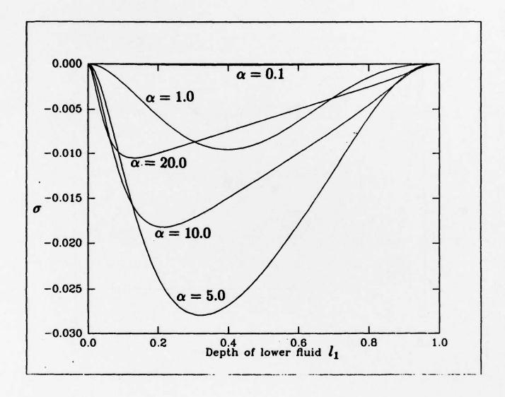
Graph of  $\sigma$  versus  $l_1$ , the depth of the lower fluid.  $\alpha_1 \Delta T' = 0.001$ . R = 1,  $\bar{\beta} = 1$ ,  $\alpha = 0.1, 1.0, 5.0, 10.0, 20.0$ .
