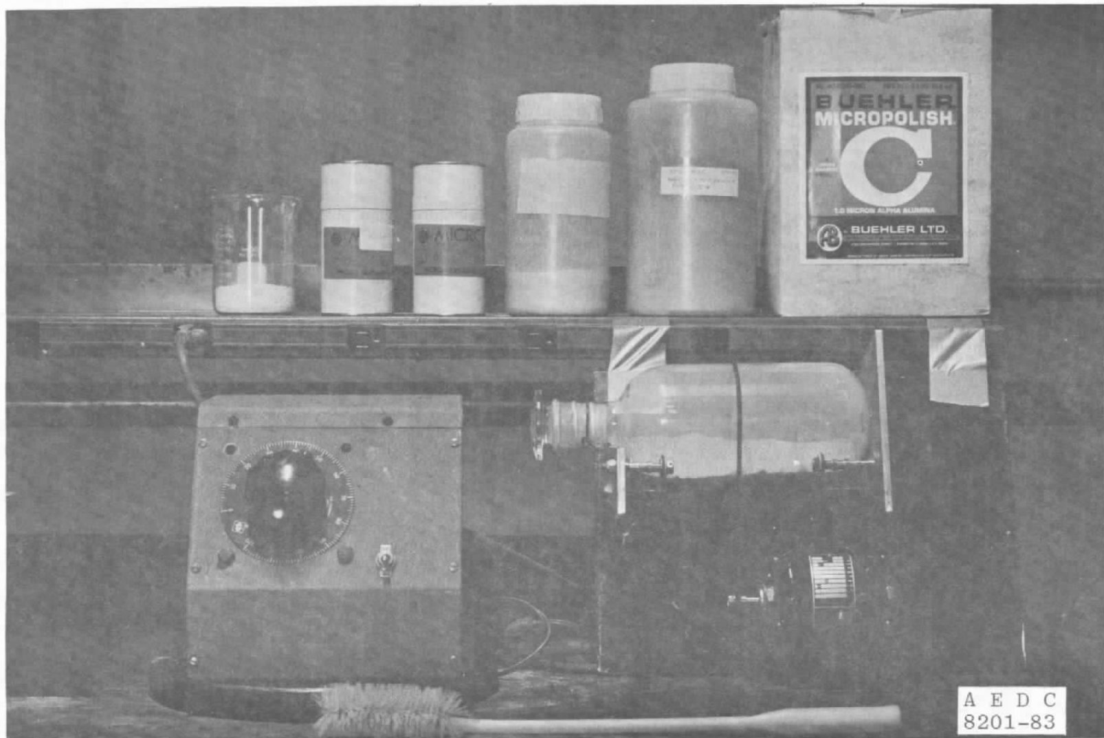
Figure 4. Agglomerate generation apparatus.
