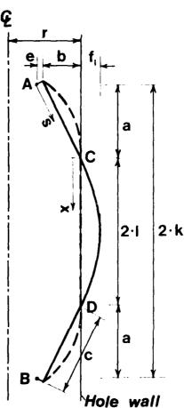
Figure 1. Leaf spring geometry
