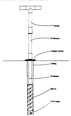
Figure 1. Lightweight hand auger with casing.
