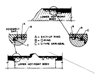
Figure 2. Hermetic sealing method of the instrument chamber
