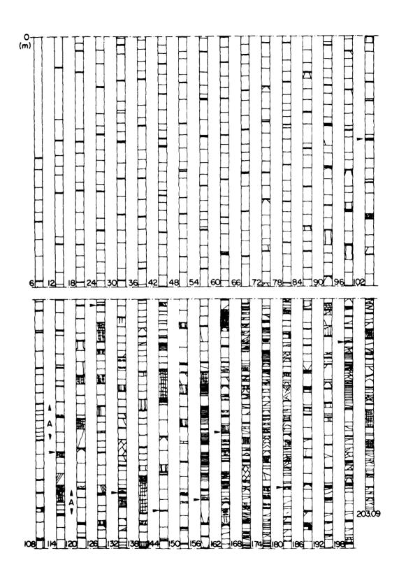
re 5. Core logging information at Site D 57, showing the different core fracs observed in the ice. The thick horizontal lines correspond to the limit of the s obtained in each run. The symbol "A" indicates runs made with the core barrel at Dome C (No. I).
