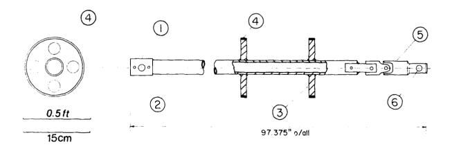
Figure 4. Connecting rod for reamer attachment. (1) Connection to clutch output shaft (see Fig. 1c item no. 21). (2) Main shaft. (3) Bearing wheels. (4) Teflon surface. (5) Universal coupling. (6) Connection to reamers.
