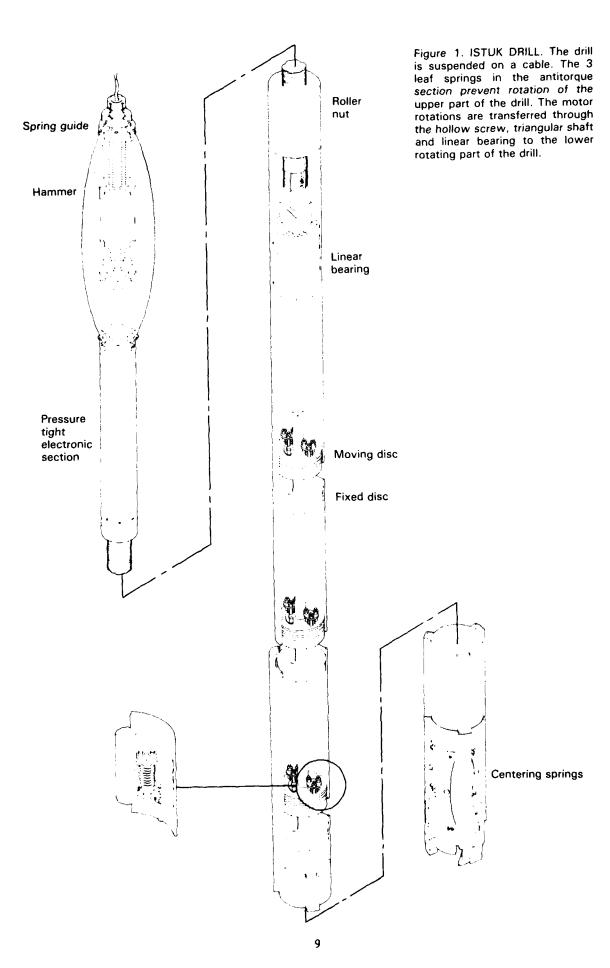
In fact, this concept is so effective that power transfer capacity is second to mechanical strength in specifying the cable. A 6.4 mm cable can power a drill 3300 m downhole!
