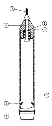
Figure 1. ETB-1 electro-thermal core drill. (1) Heater shoe. (2) Core barrel.
