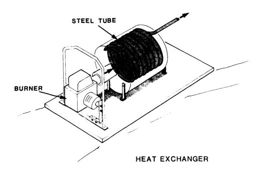
Figure 2. An illustration of the water heater. Either diesel fuel or turbo fuel (JP-4) can be used to supply the heat. The total weight of the unit is about 150 kg.
