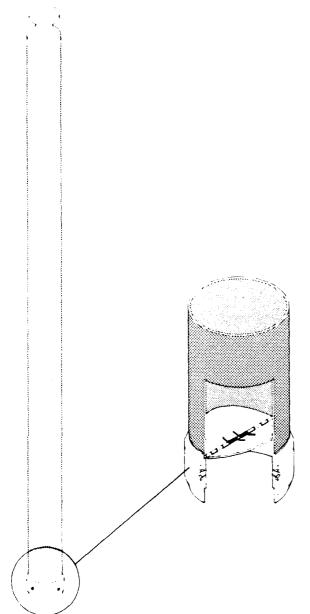
Figure 8. Downbore hole filter. The spring-loaded valves at the bottom of the filter (lower right) open when the filter moves through the hole liquid, collecting the floating chips.
