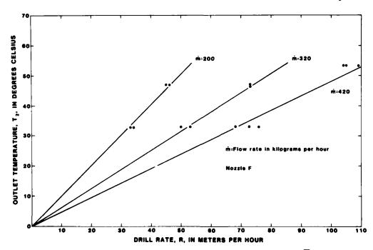
Figure 4. Data of figure 3 for nozzle F, with slope of lines  $\overline{d}$  = 5.92 cm at the mass flow rates indicated. Drill rate proportional to outlet water temperature,  $T_2$ .
