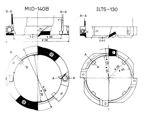
Figure 3. Cutter shoe assemblies of the MID-140B and ILTS-130C drills.
