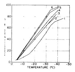
Figure 3. Dependence between the viscosity of an ethyl alcohol-water-glycol solution and its freezing temperature. Curves 1 through 6 correspond to 0 % chrough to 5 % glycol by weight.
