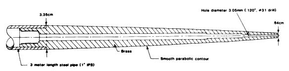
Figure 9. Drawing of the nozzle shown in figure 8.
