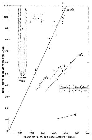
Figure 2. Test results for a longer nozzle E.
