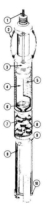
Figure 3. Schematic diagram of the electro-mechanical drill. (1) Electro-mechanical cable. (2) Springs. (3) Submersible motor. (4) Filter. (5) Centrifuge basket. (6) Propeller. (7) Gear reducer. (8) Hollow shaft. (9) Rectangular tubes. (10) Cutters.
