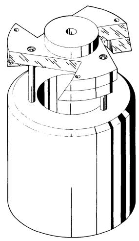
Figure 9. Reamer. The reamer is mounted on the exit shaft of the electronic section. The front cylinder centers the unit in the hole.
