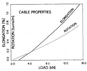
Figure 13. Cable elongation and rotation versus cable tension.
