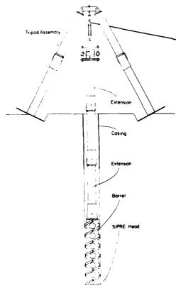
Figure 4. Lightweight auger with tripod assembly.
