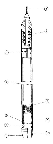
Figure 1. Schematic diagram of the ETB-3 electro-thermal core drill.
