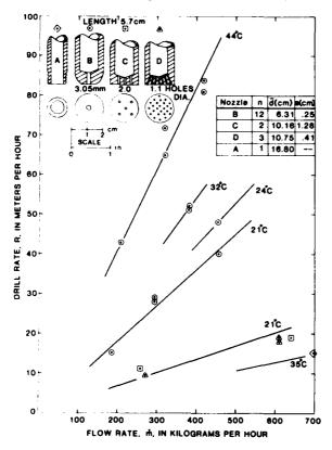
Figure 1. Block Ice Tests. Number of data points, n, with lines of slope d calculated from equation 1 at the nozzle water temperature indicated; s, the standard deviation of each set. Test nozzles made of brass. Drill rate proportional to flow rate.
