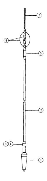
Figure 2. Electro-thermal "Needle" drill. (1) Conical heater bit. (2) Central pipe.
