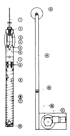
Figure 1. Schematic diagram of the drill, tower and winch assembly. (1) Electromechanical cable. (2) Cable termination. (3) Knocker weight. (4) Spring. (5) Slipring. (6) Submersible motor. (7) Gear reducer. (8) Clutch. (9) Chip inlets. (10) Auger flights. (11) Core barrel.
