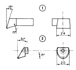
Figure 2. Cutter design. (1) Electromechanical drill No. I used at Dome C. (2) Electro-mechanical drill No. II used at site D57 and James Ross Island. (Dimensions are in mm).
