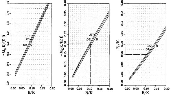
Figure 2d. Maximum absolute bending moment as function of b/k for the indicated values of the dimensionless eccentricity of the spring support.
