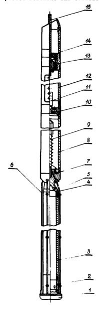
Figure 1. The TBZS-152M thermal core drill. (1) Heater ring (2) Core lifter (3) Core barrel (4) Drain adapter (5) Water pipes (6) Heater power cable (7) Water heater (8) Tank (9) Water pipe (10) Pump adapter (11) Pump (12) Electrical section (13) Cable termination (14) End cap (15) Electro-mechanical cable.
