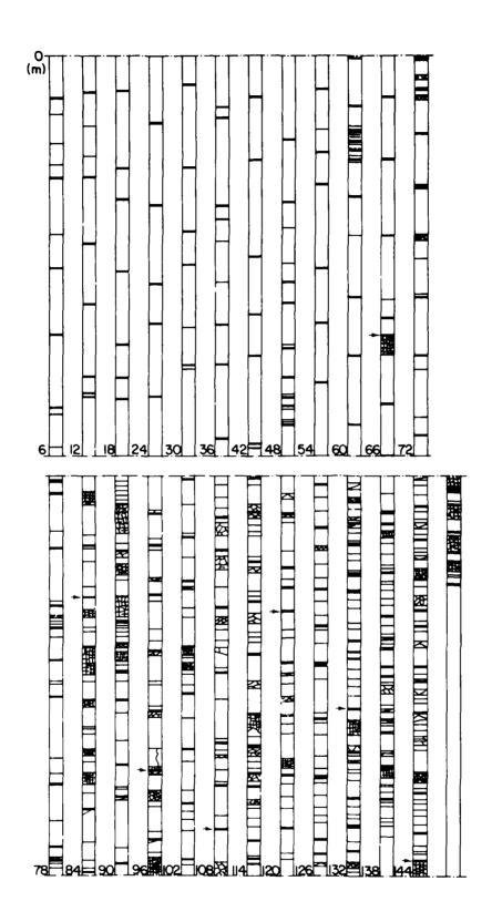
There 7. Core logging information for the James Ross Island site, showing the interest core fractures observed in the ice. The thick horizontal lines correspond to the cores obtained in each run.
