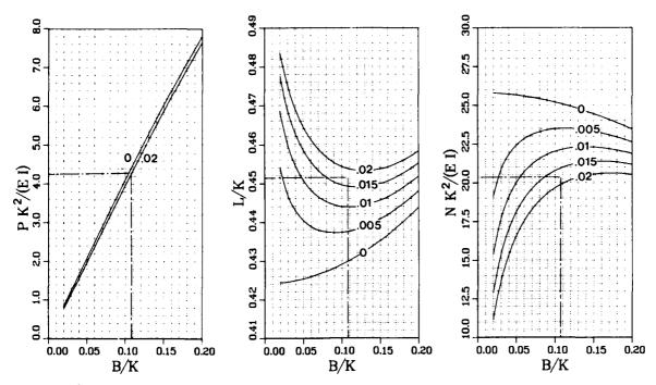
Figure 2a. Dimensionless transverse supporting force as function of b/k for the indicated values of the dimensionless eccentricity of the spring support.
