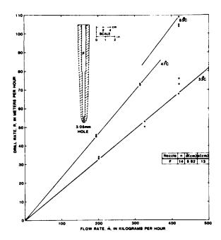
Figure 3. Test results for a larger and more pointed nozzle F. Both d and s have smaller values indicating smoother, more efficient drilling.
