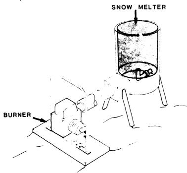
Figure 3. A snow melter for creating the initial water to start the hot-water drill. The snow is melted in the inner tank of two concentric tanks.
