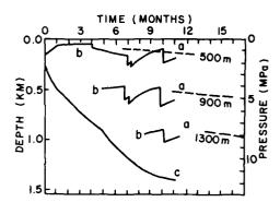
Figure 1. The calculated and observed liquid pressure in the No. 3G bore hole during the 1980 Vostok station operations. Curves (a)— the calculated and required pressures for depths of 500 m, 900 m and 1300 m. Curves (b)— the observed pressure values for depths of 500 m, 900 m and 1300 m. Curve (c) is the drilling progress plot.
