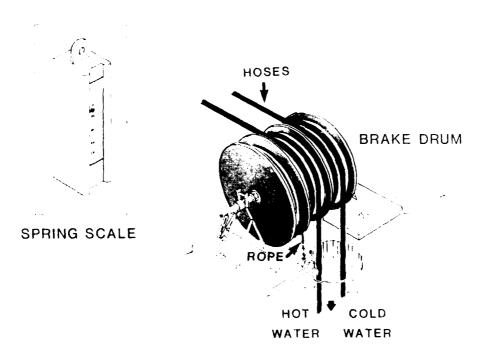
igure 5. An illustration of the brake drum that is used to provide an upward force on the hoses. This tension, which is less than the weight of the drill head, helps to keep the hoses (and thus the hole) plumb. The inset indicates the spring scale which shows the retarding force. An electric drive can be fit over the square shaft. This turns the brake into a capstan to help raise the drill.
