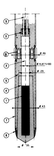
Figure 1. Cross section of the hot point. (1) High power density cartridge; element resistance =  $46~\Omega$ . (2) Cold part of cartridge. (3) Glass-metal sealing. (4) Copper cylinder brazed to cartridge. (5) Ceramic coating used as thermal insulation. (6) Stainless steel tip brazed onto the copper cylinder. (7) Stainless steel tube. (8) Cooling flange brazed onto the cartridge. The holes are used for setting the ceramic around the copper cylinder. (9) Copper wire used for power conductor.
