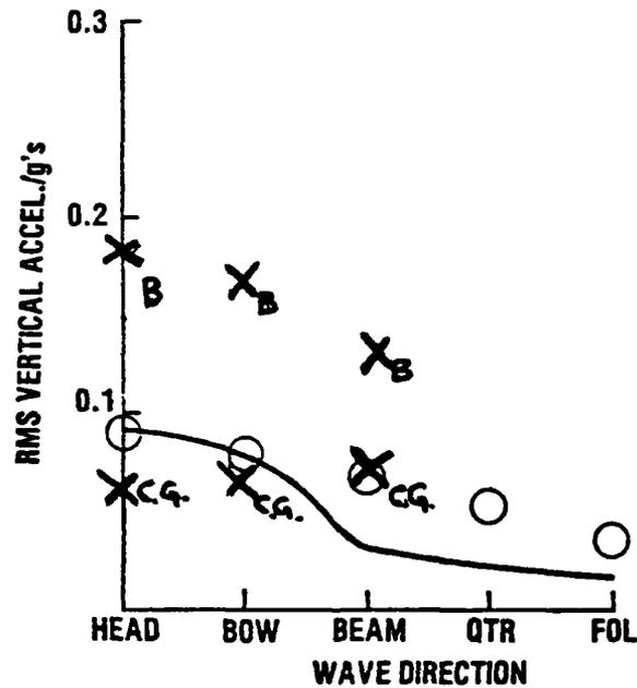
Figure 4.5-1. COMPARISON OF PCH-1 AND EPH VERTICAL MOTIONS
