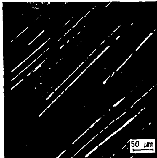
(b) Close-up view of shear offset due to sliding of debonded fibers; stress axis vertical.
