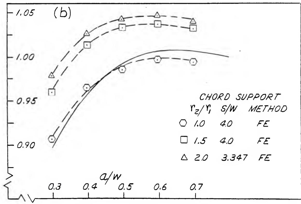
Figure 5. Crack mouth displacement,  $v$ , versus  $a/W$  for bend specimens of various geometry.
