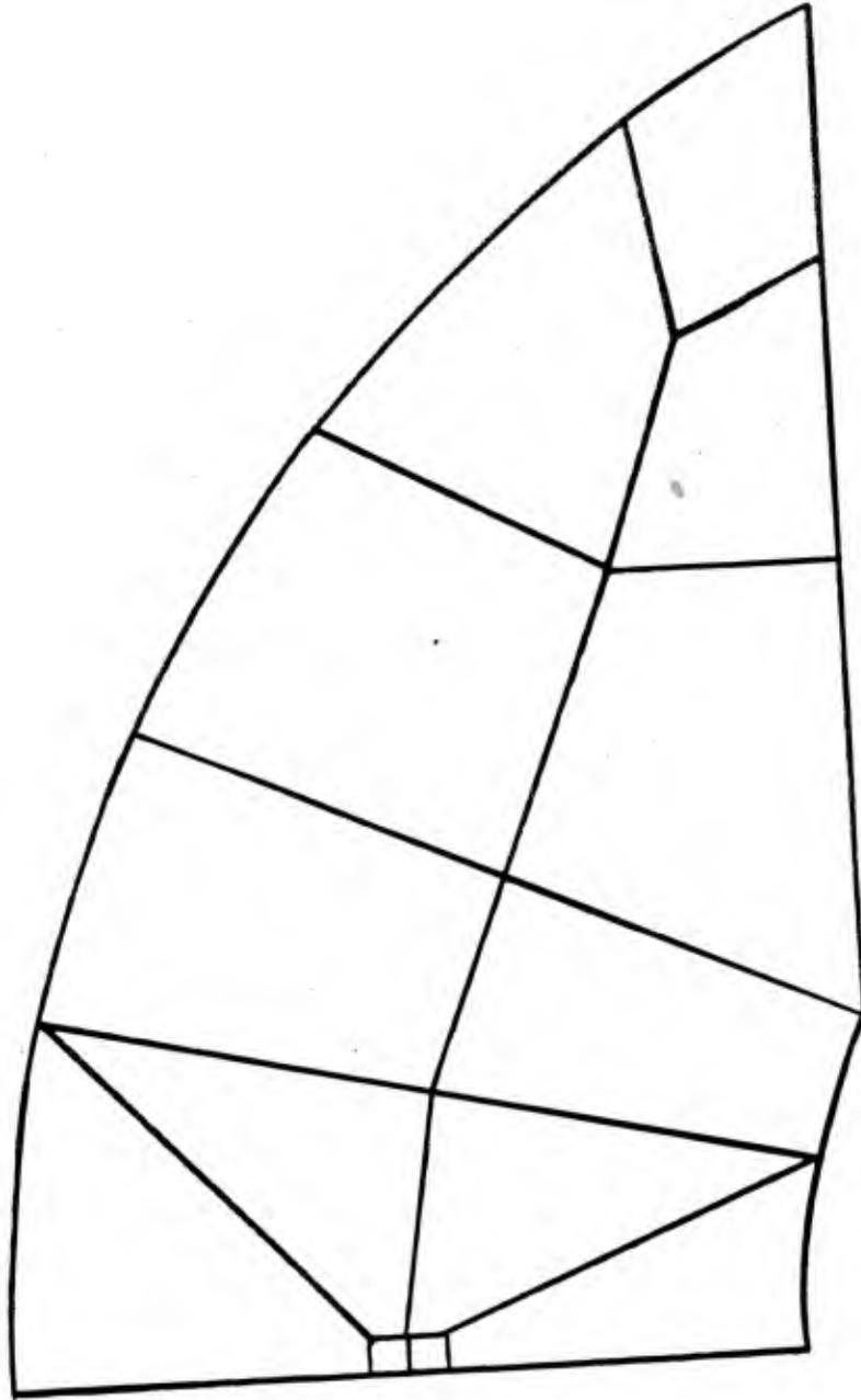
Figure 3. Finite element arrangement for arc bend-chord support specimen;
