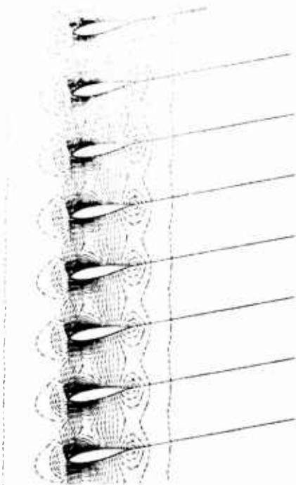
Fig.10 3D iso-Mach curves  $r/k = 0.2$ ,  $M_0 = 0.8$
