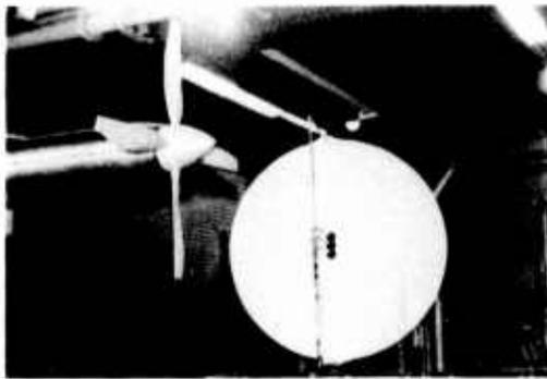
Fig. 4 Propeller No. 3 (with Q-Tips) and acoustic mirror telescope
