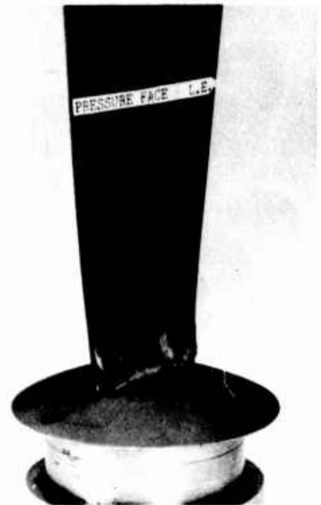
Fig. 6 Damaged composite blade subsequently run at 8000 rpm
