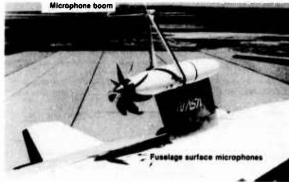
Figure 32. Microphone boom and fuselage surface microphones on Jetstar
