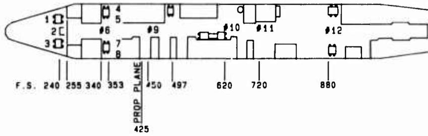
Figure 1 P-3 Aircraft Measurement Locations
