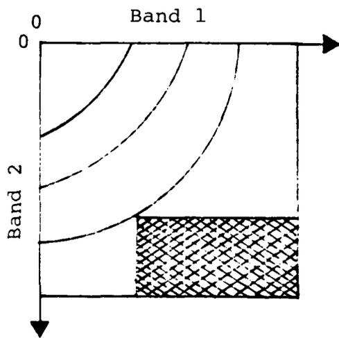
Figure 2. -- Determination of cumulative 2-color frequencies.
