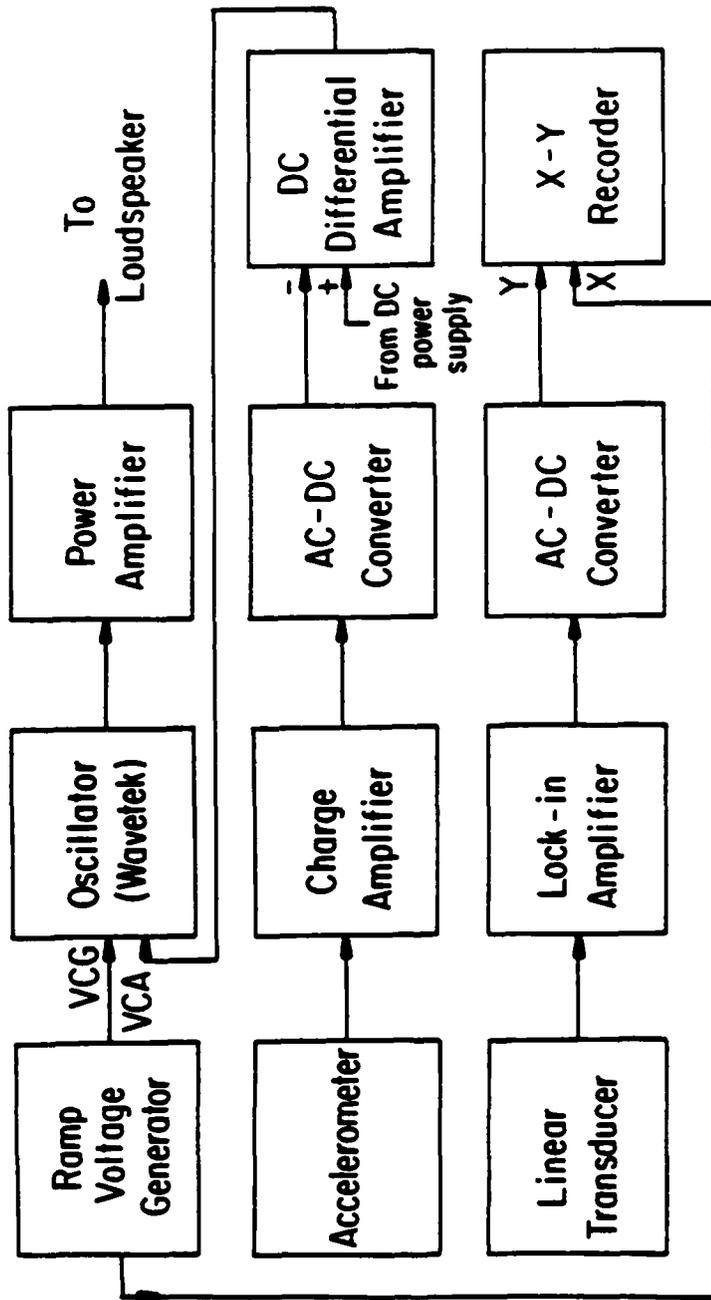
FIGURE 18 The block diagram of the electronics.
