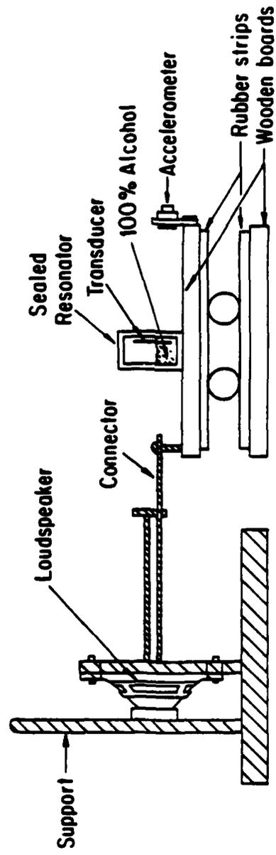
FIGURE 17 Schematic of the apparatus with direct drive.
