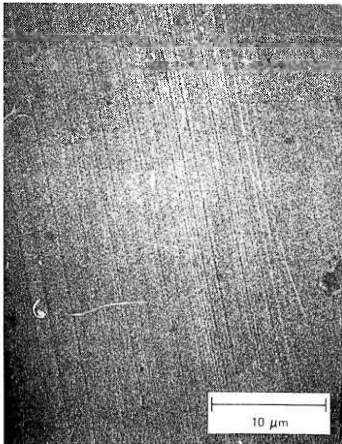
Figure 62. Ball - Williams Research Corp. 3000X Condition: Unetched
