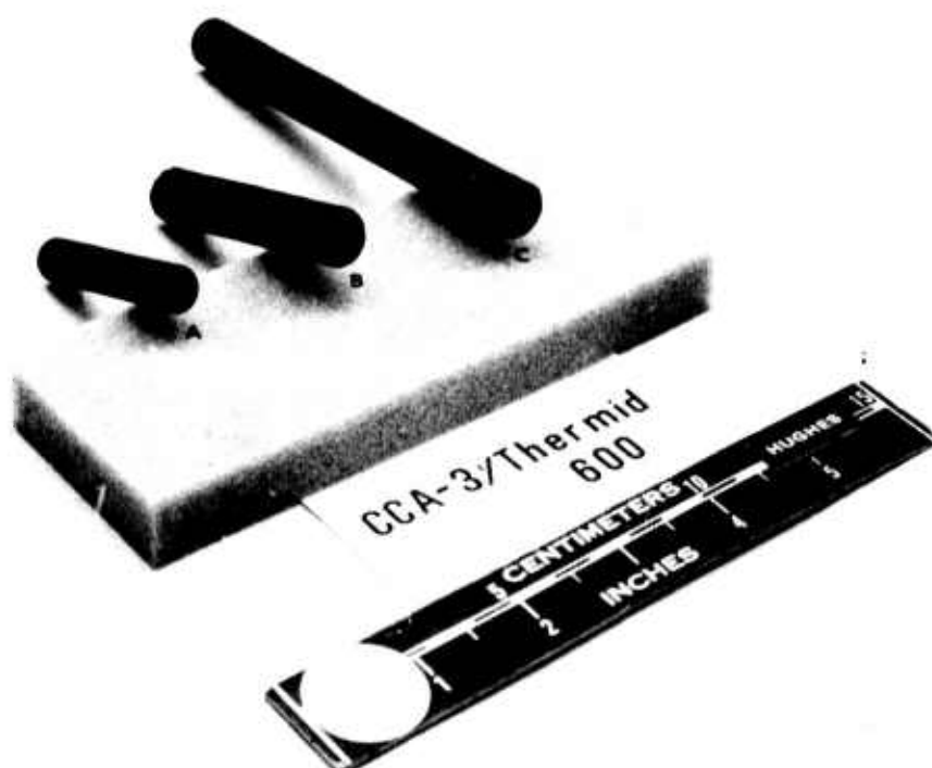
Figure 23. Improved, expanding silicone rubber plug-prepared Hughes 2D carbon/polyimide gyro bearing retainer stock.
