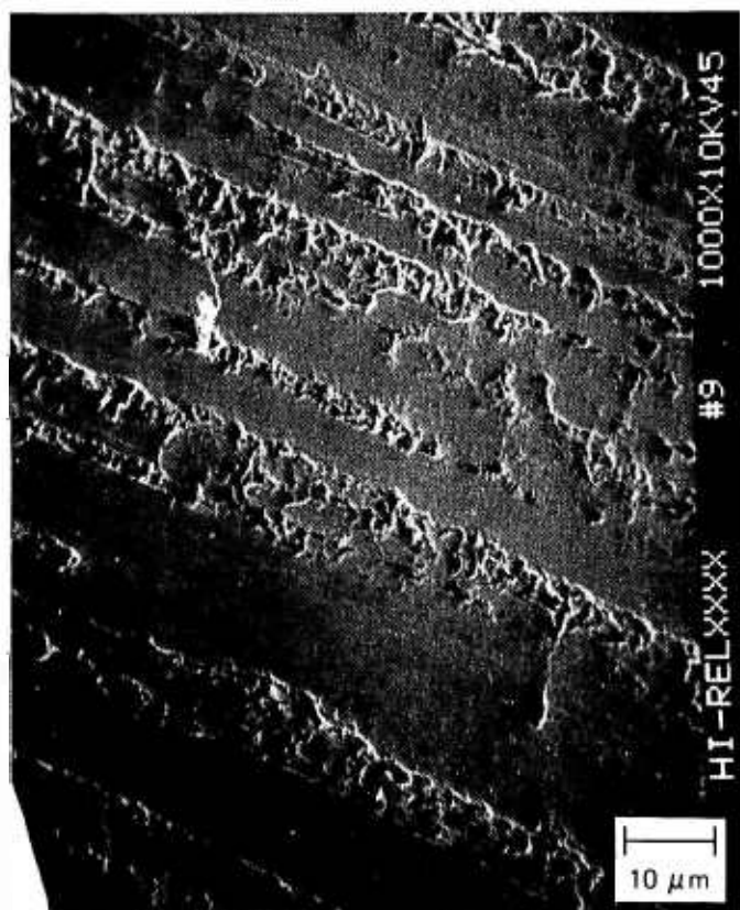
Figure 60. Bearing Surface Damaged by The Machining Process
