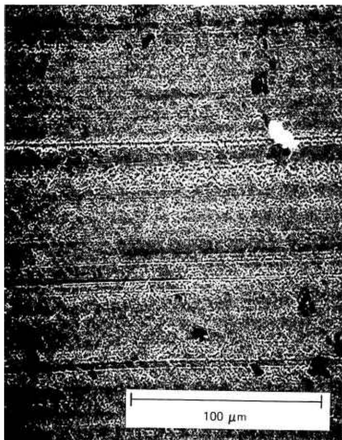
Figure 54a. Specimen 6 One Layer Etch Bearing Surfaces Damaged by The Machining Process 500X
