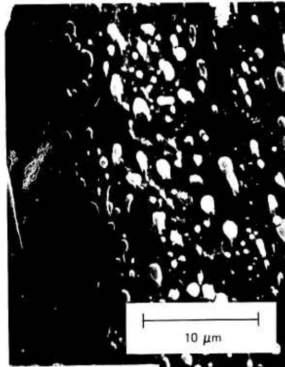
Figure 93. Transition Zone 3000X Near Ball Track
