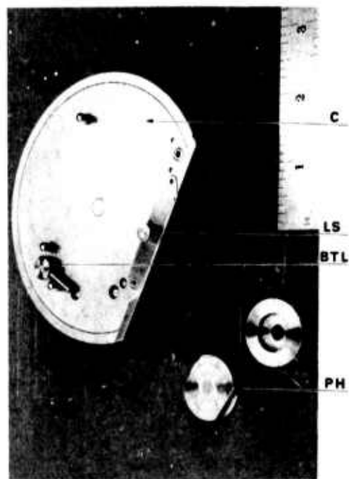
Figure A-4. Precision Guinier camera film holder and powder specimen holders: Guinier camera film holder assembly (C), manually-operated beam trap level (BTL), light shutter (LS), and powder specimen holders (PH).
