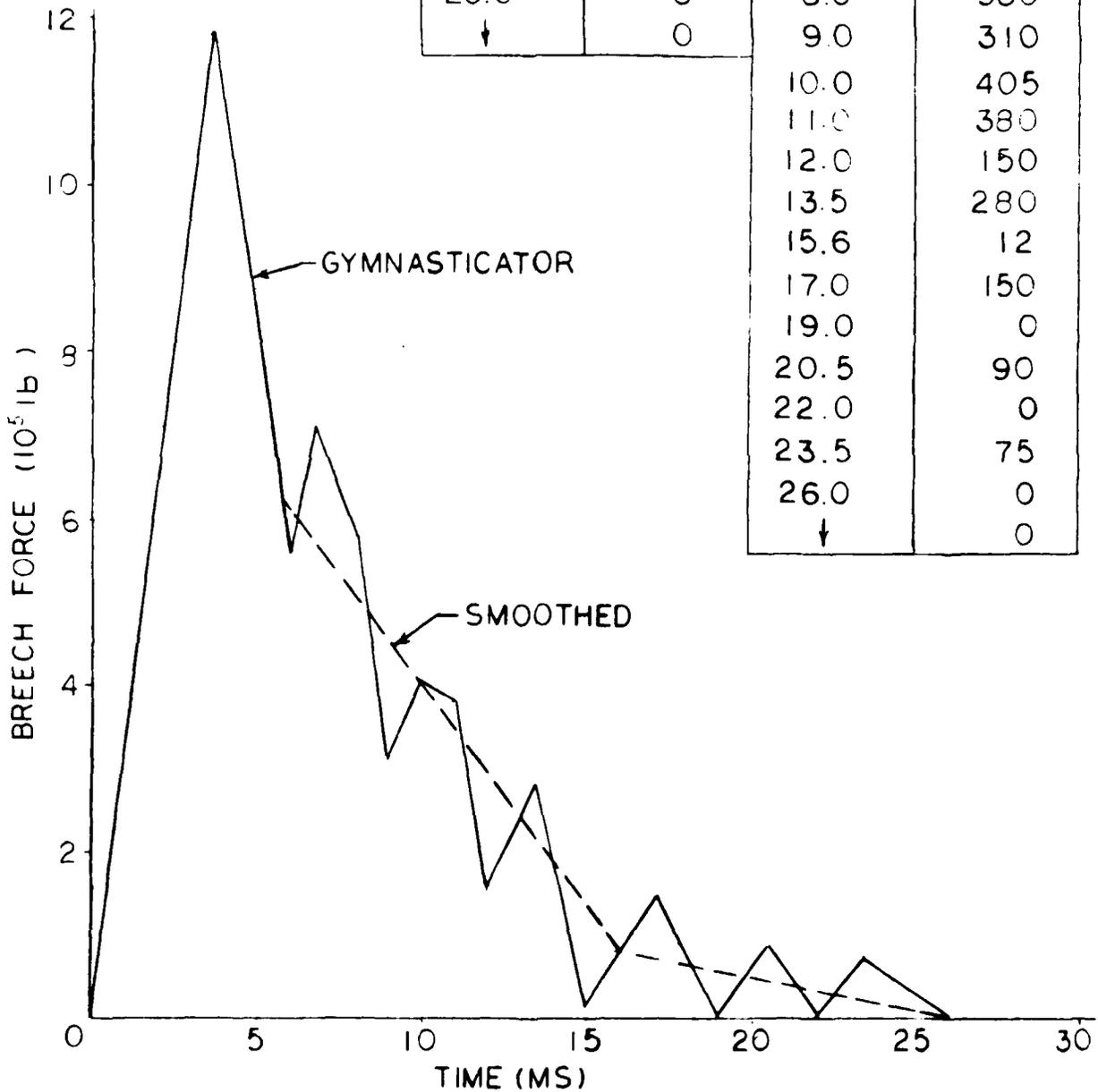
Figure 17. Breach force profile based on recoil response--powder gymnasticator (M203 equivalent)
