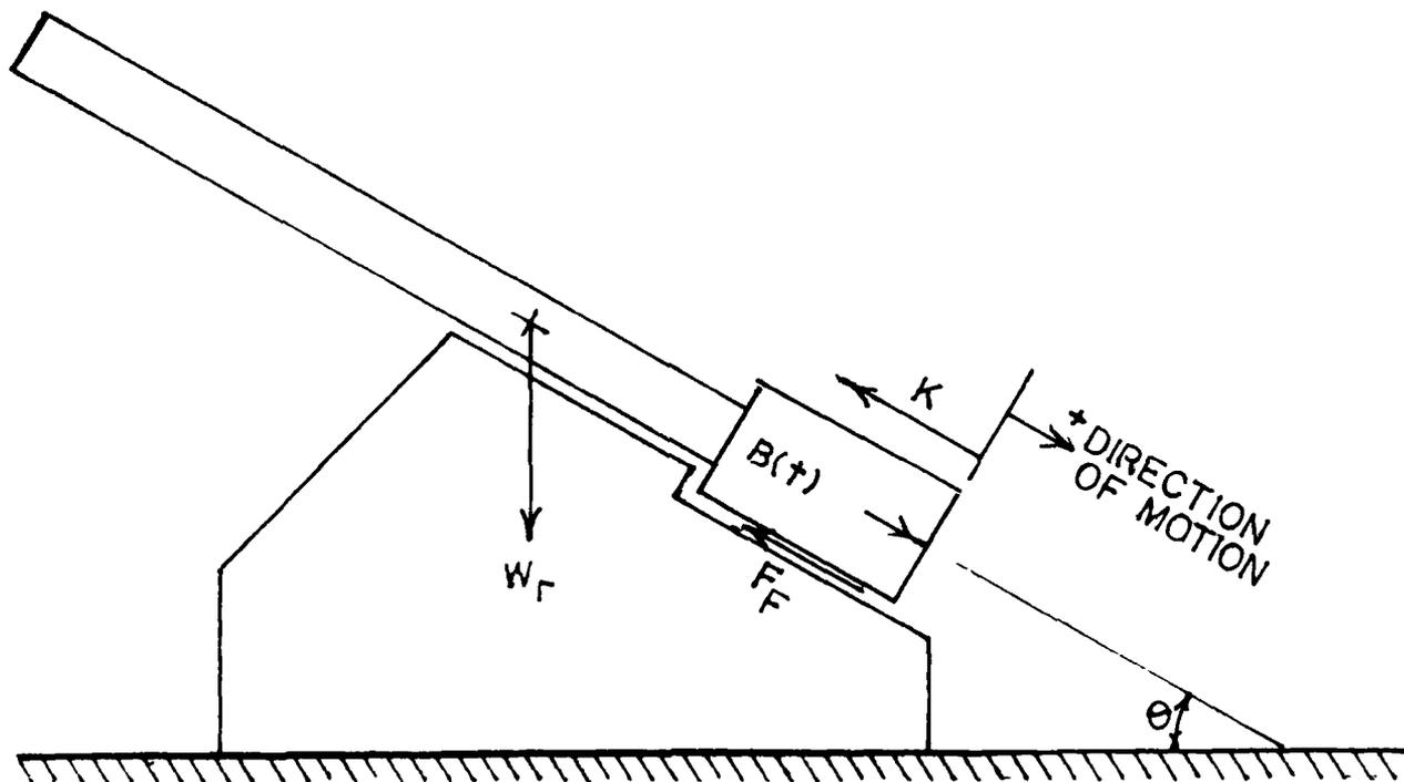
Figure 1. Forces acting on typical artillery recoil mechanism
