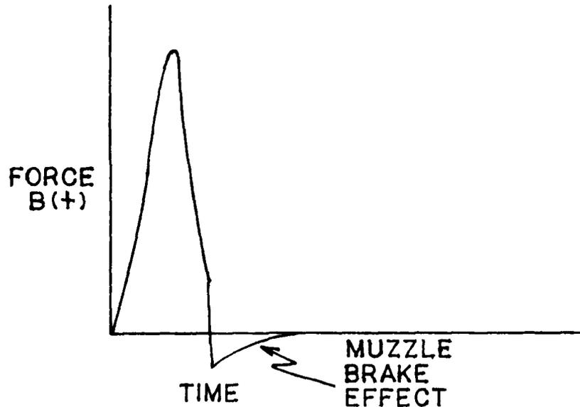
Figure 3. Typical breech force profile with muzzle brake
