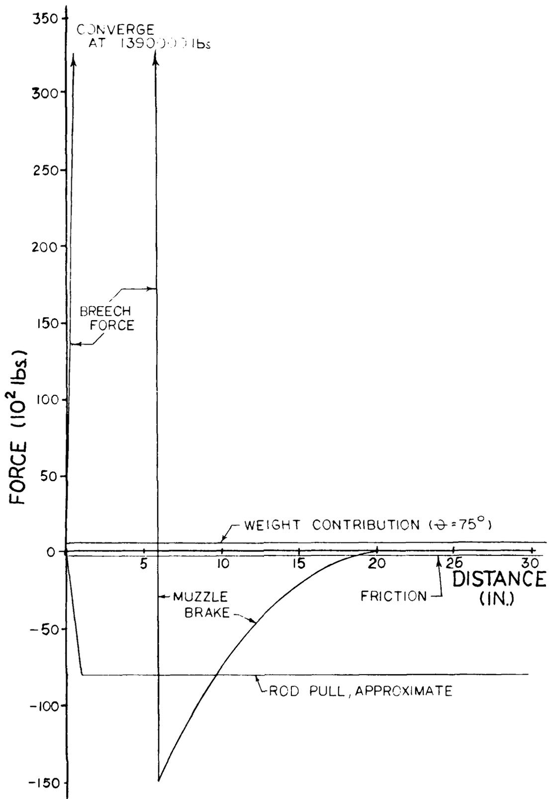
Figure 20. Magnitude of forces in recoil process
