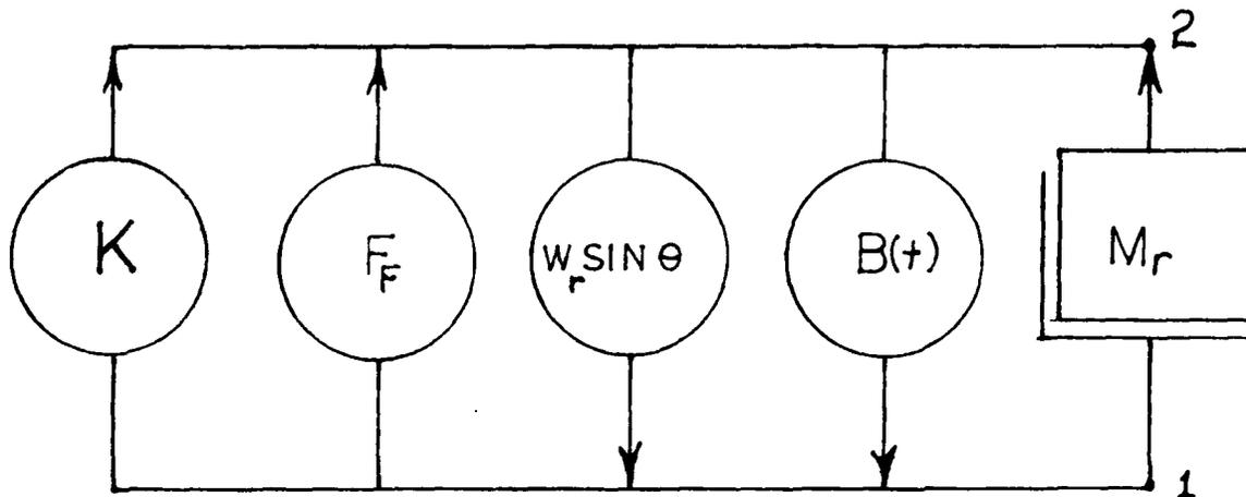
Figure 8. Recoil mechanism network for SUPER\*SCEPTRE model
