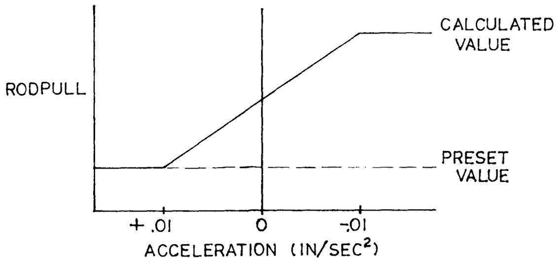
Figure 21. Transition function for calculated rodpull
