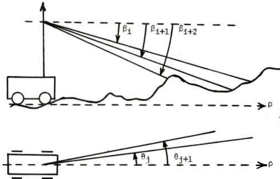
Figure 1. Top and side view of a rangefinder.
