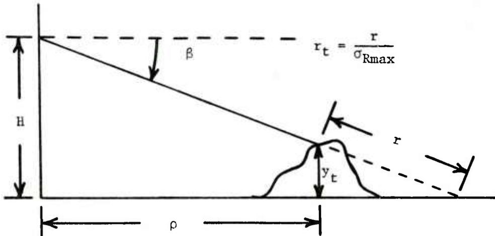
Figure 2. Geometrical relationship of residual  $r$  to model parameters.
