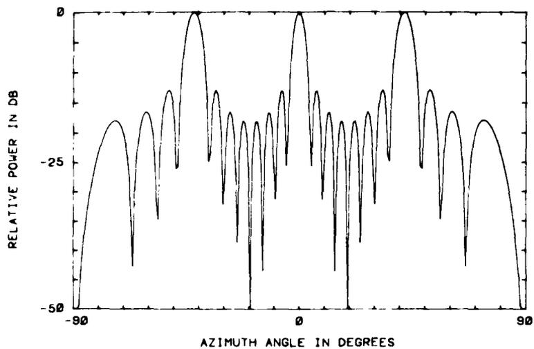
Figure 12. Array Factor for a Three-Element Array With a Spacing of  $1.5\lambda$
