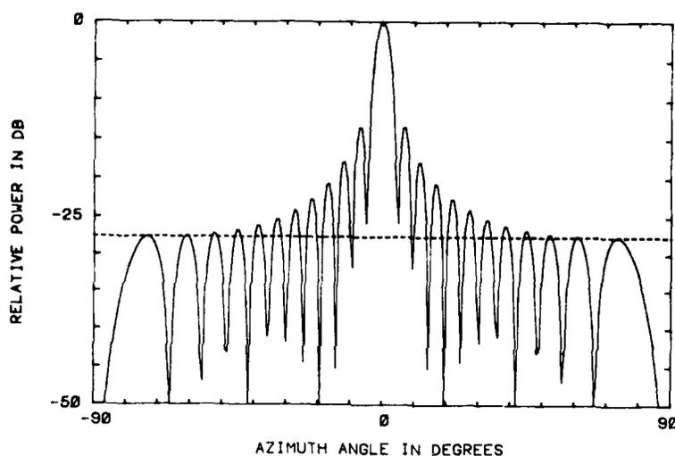
Figure 6. Far-Field Pattern of an Isotropic Element Superimposed on the Quiescent Pattern
