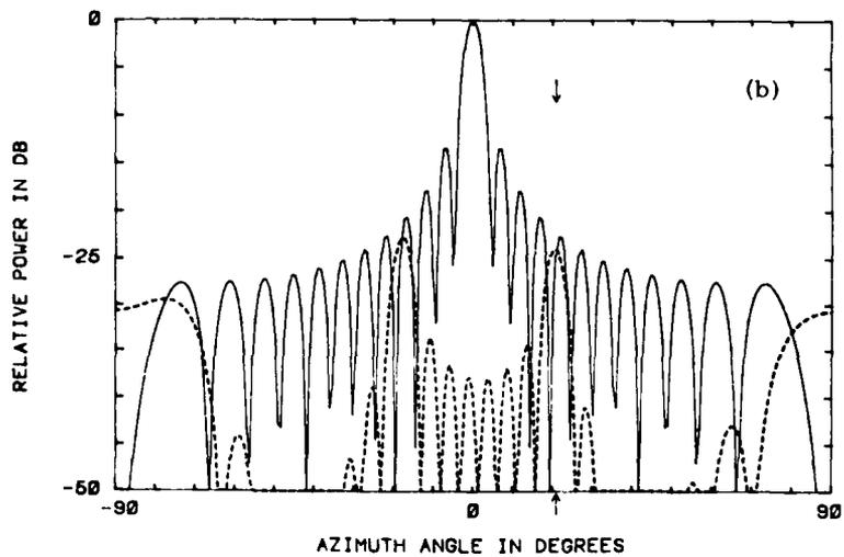
Figure 14. Placing a Null at 21° With Eight Subarrays.
