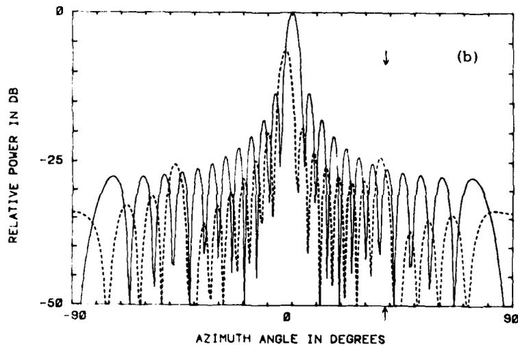
Figure 10. Placing a Null at  $38^\circ$  With Eight Subarrays.
