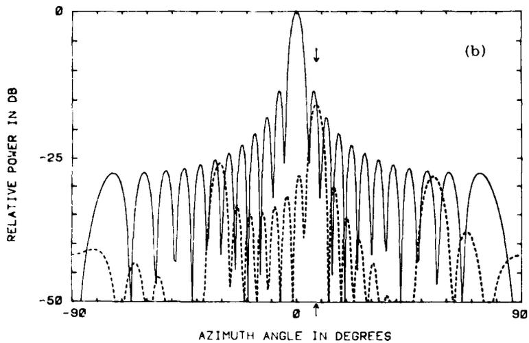
Figure 4. Placing a Null at  $8^\circ$  With Eight Subarrays. (a) Far-Field Pattern, (b) Cancellation Beam Superimposed on Quiescent Pattern
