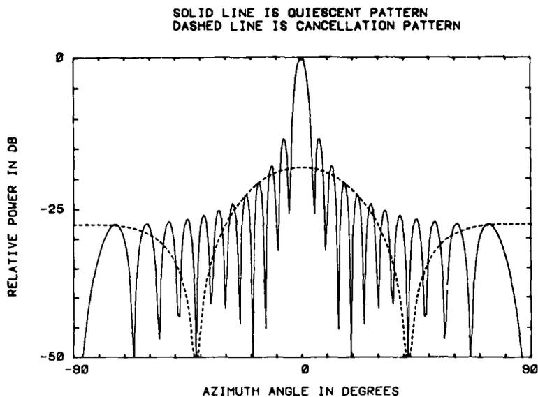
Figure 7. Far-Field Pattern of a Three-Element Subarray Superimposed on the Quiescent Pattern
