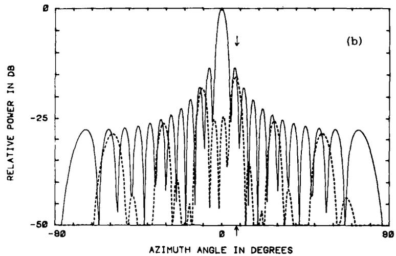
Figure 5. Placing a Null at 8° With Four Subarrays. (a) Far-Field Pattern, (b) Cancellation Beam Superimposed on Quiescent Pattern
