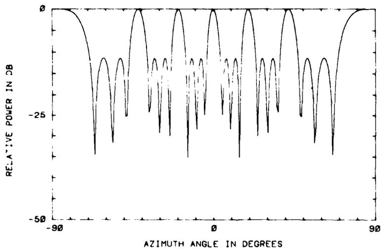
Figure 13. Array Factor for a Six-Element Array With a Spacing of  $3.0\lambda$
