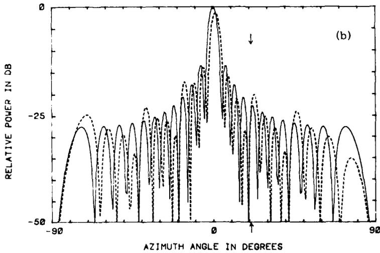
Figure 15. Placing a Null at 21° With Four Subarrays.
