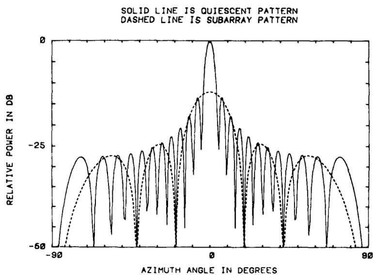
Figure 8. Far-Field Pattern of a Six-Element Subarray Superimposed on the Quiescent Pattern
