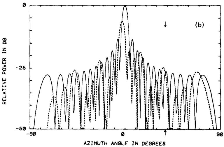
Figure 11. Placing a Null at 38° With Four Subarrays.
