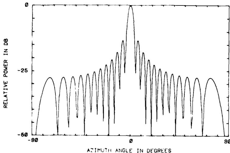
Figure 2. Quiescent Far-Field Pattern of a Twenty-Four Element Uniform Array
