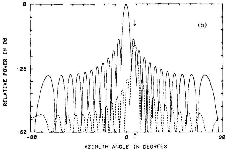
Figure 3. Placing a Null at 8° With Twenty-Four Subarrays.
