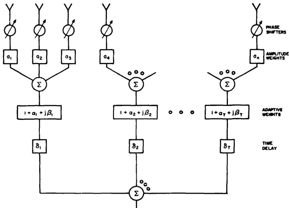
Figure 1. Linear Array Divided Into Subarrays
