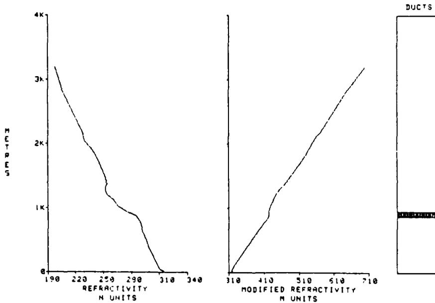
Figure 55. (a) Q and  $\theta$  Plot for Radiosonde Soundings Made 29 July 1983, 1329 GMT. (b) IREPS Output for 29 July 1983, 1329 GMT.
