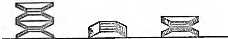
(a) SERIES (b) PARALLEL (c) PARALLEL-SERIES
