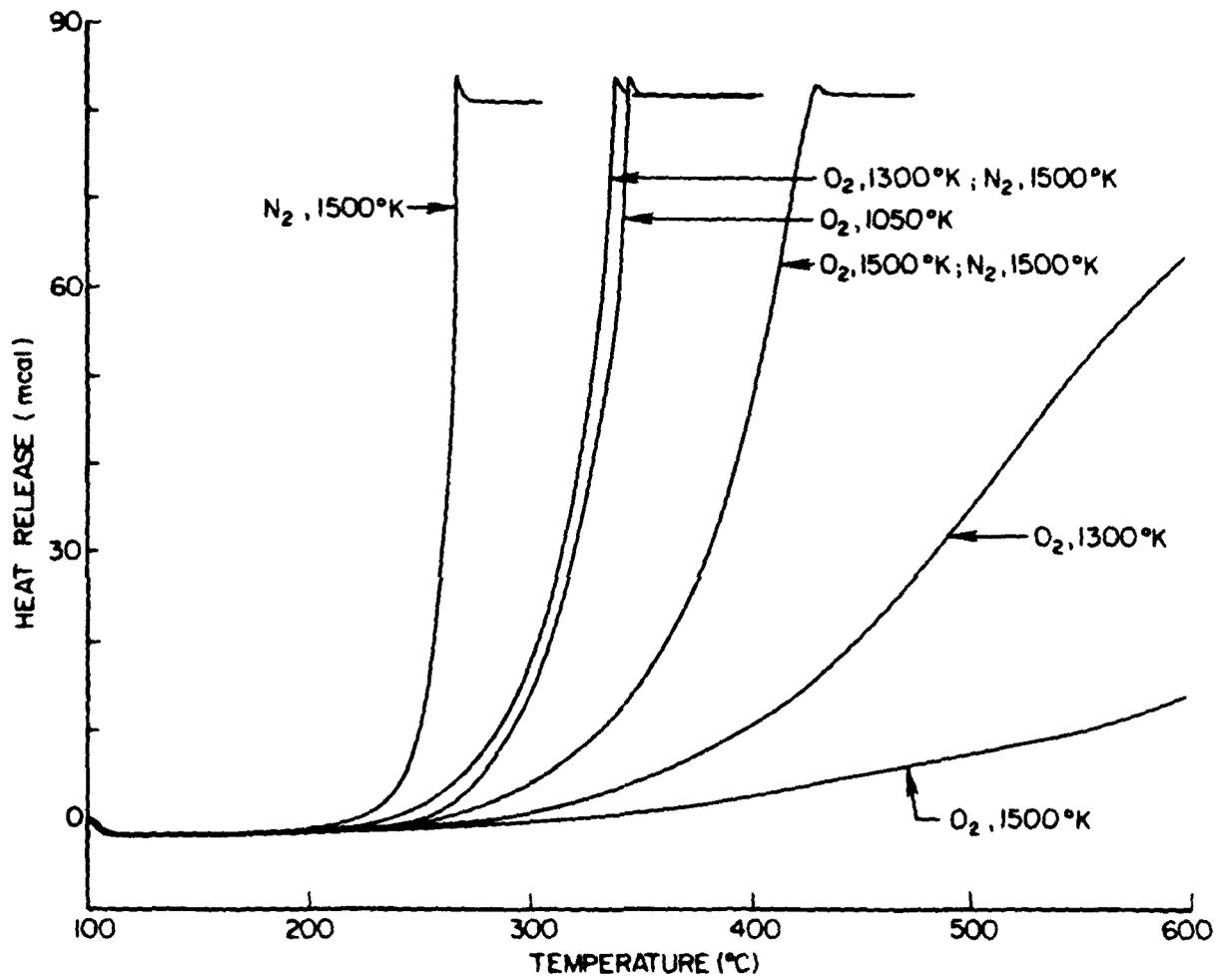
FIGURE 20. DIFFERENTIAL SCANNING CALORIMETER TESTS OF 2% Pt PEROVSKITE POWDER AFTER AGING
