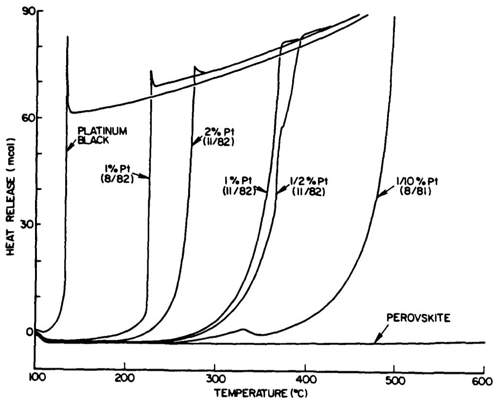
FIGURE 17. DIFFERENTIAL SCANNING CALORIMETRY TESTS OF RELATIVE CATALYTIC ACTIVITY WITH PROPANE IN AIR AT AN EQUIVALENCE RATIO OF 2.8
