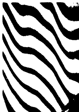
Figure 36. Beam Interferogram after reflection on one poor mirror.
