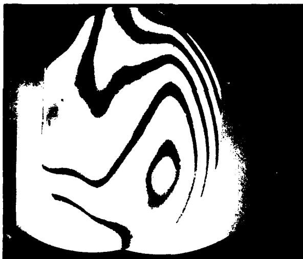
Figure 40. Beam Shearing interferograms after the spherical telescope mounted with two poor quality mirrors.
