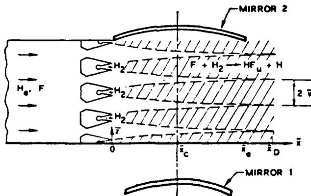
Figure 12. Laser Cavity with Unstable Resonator.
