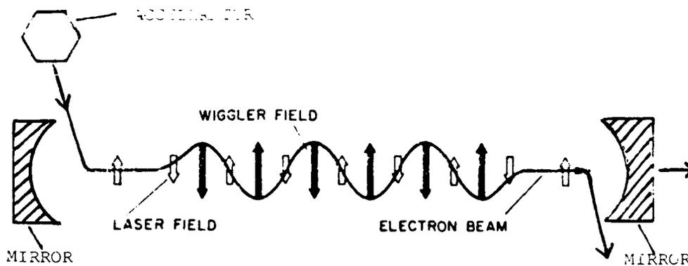
Figure 14. Basic Principle of a Free Electron Laser.
