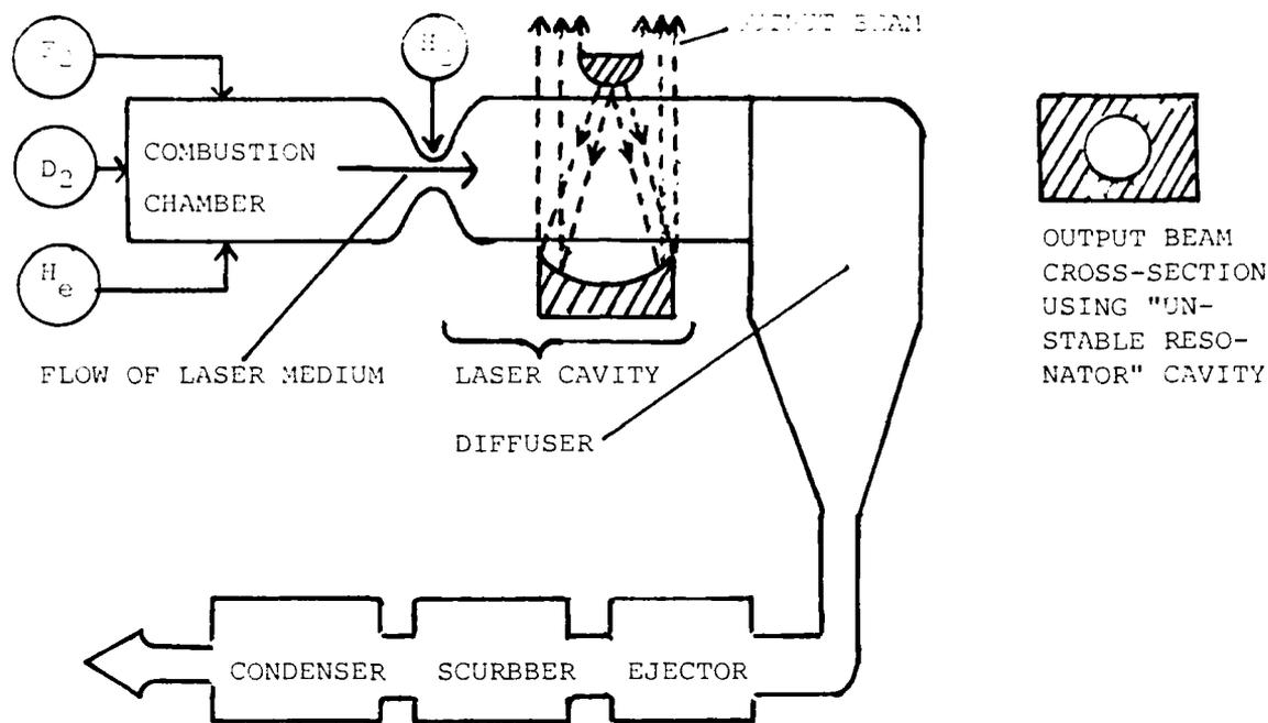
Figure 8. Combustion-Driven, Supersonic-Diffusion HF Chemical Laser System [Ref. 18].
