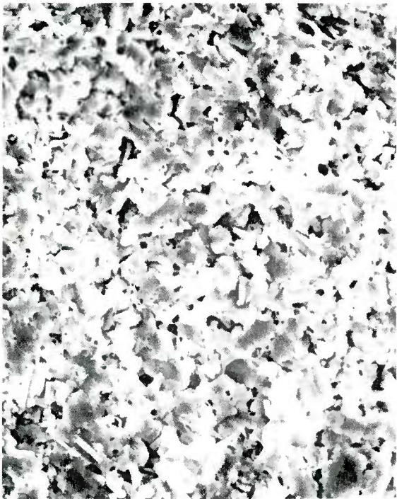
Figure 2. Interior of Black Powder Grain Produced by Jet-Mill Process
