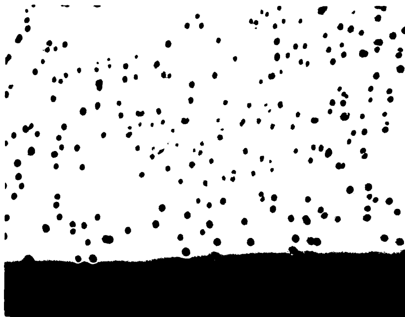
Figure 3. Spheroidal Regions in the RHA Microstructure Removed During Polishing. Unetched, 55X.
