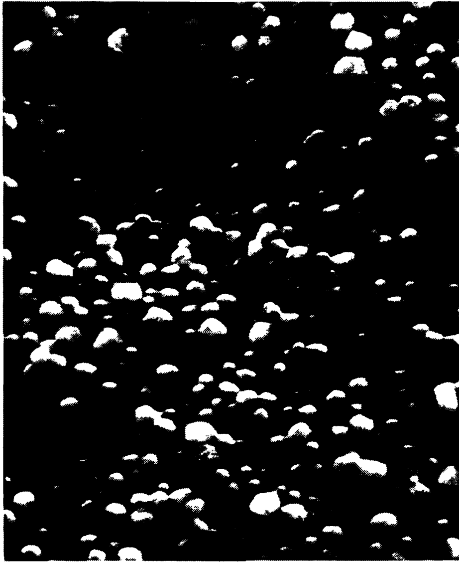
Figure 2. Scanning electron microscope photograph of the Kodak 101-07 film showing nearly spherical AgBr grains of about one micron average diameter.
