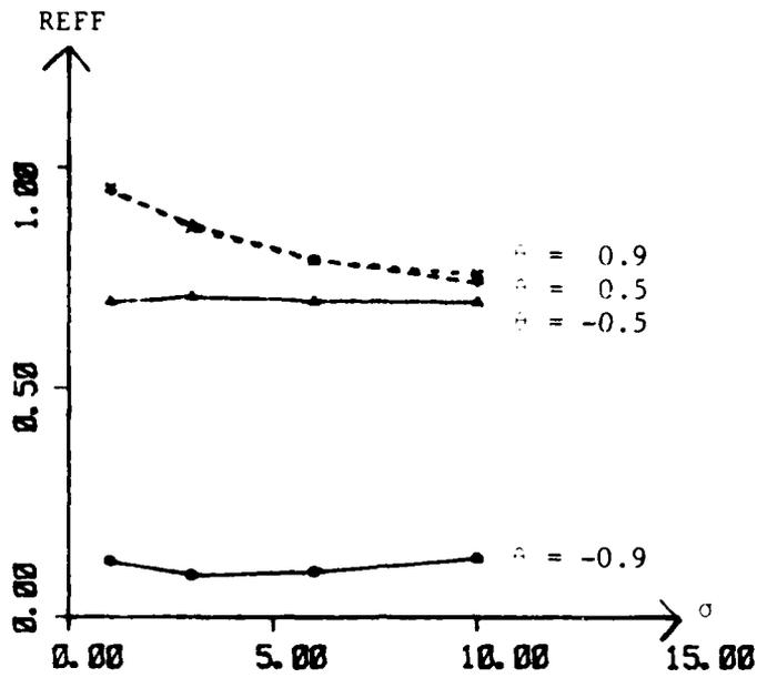
Figure 3a. REFF versus  $\sigma$  for MA(1) model using  $\psi_{\theta}$ .
