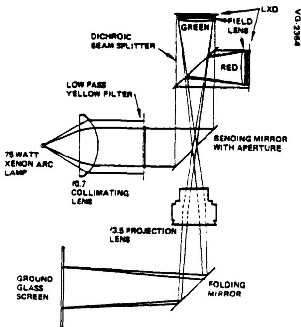
Figure 4. Optical Schematic of Color Display Demonstration Unit
