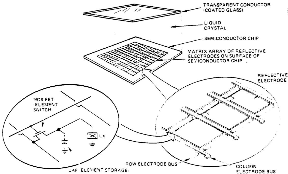
Figure 2. Liquid Crystal Display Module Construction.
