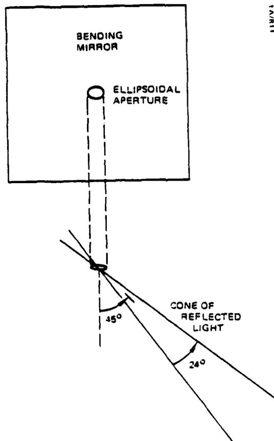
Figure 11. Aperture Geometry.
