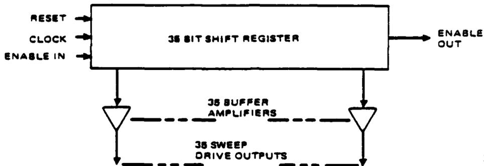
Figure 7. Sweep Driver LSI Circuit Block Diagram.
