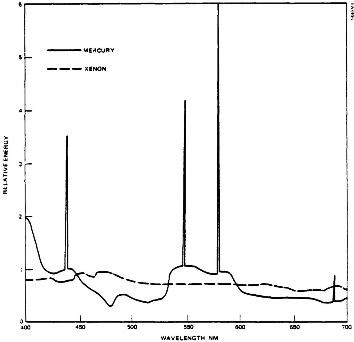
Figure 9. Spectrum of Xenon and Mercury Arc Lamps.
