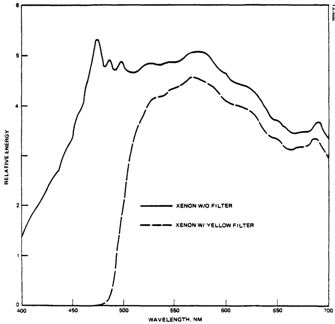
Figure 10. Spectral Distribution of Xenon Lamp after Filtration.
