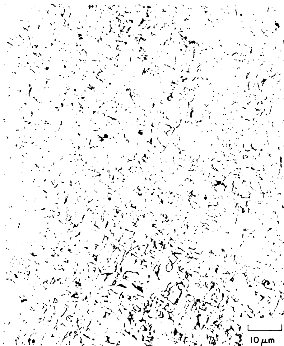
Figure 5. Example of weld metal acicular ferrite (AF) found in microalloyed HSLA steels. (2% nital etch) 1500x.
