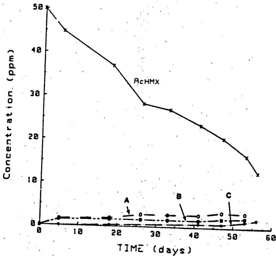
Figure 11. Kinetics of disappearance of AcHMx and production of intermediates during anaerobic incubation.
