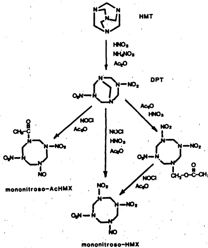
Figure 4. Preparation of mononitroso-HMX and mononitroso-AcHMX.
