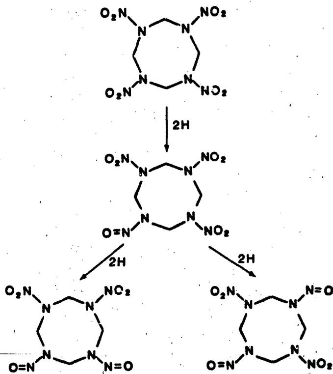
Figure 10. Stepwise reduction of nitro groups on HMX.
