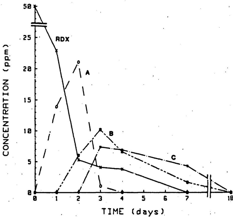
Figure 5. Kinetics of disappearance of RDX and production of intermediates during anaerobic incubation. A = mononitroso-RDX; B = dinitroso-RDX; C = trinitroso-RDX.
