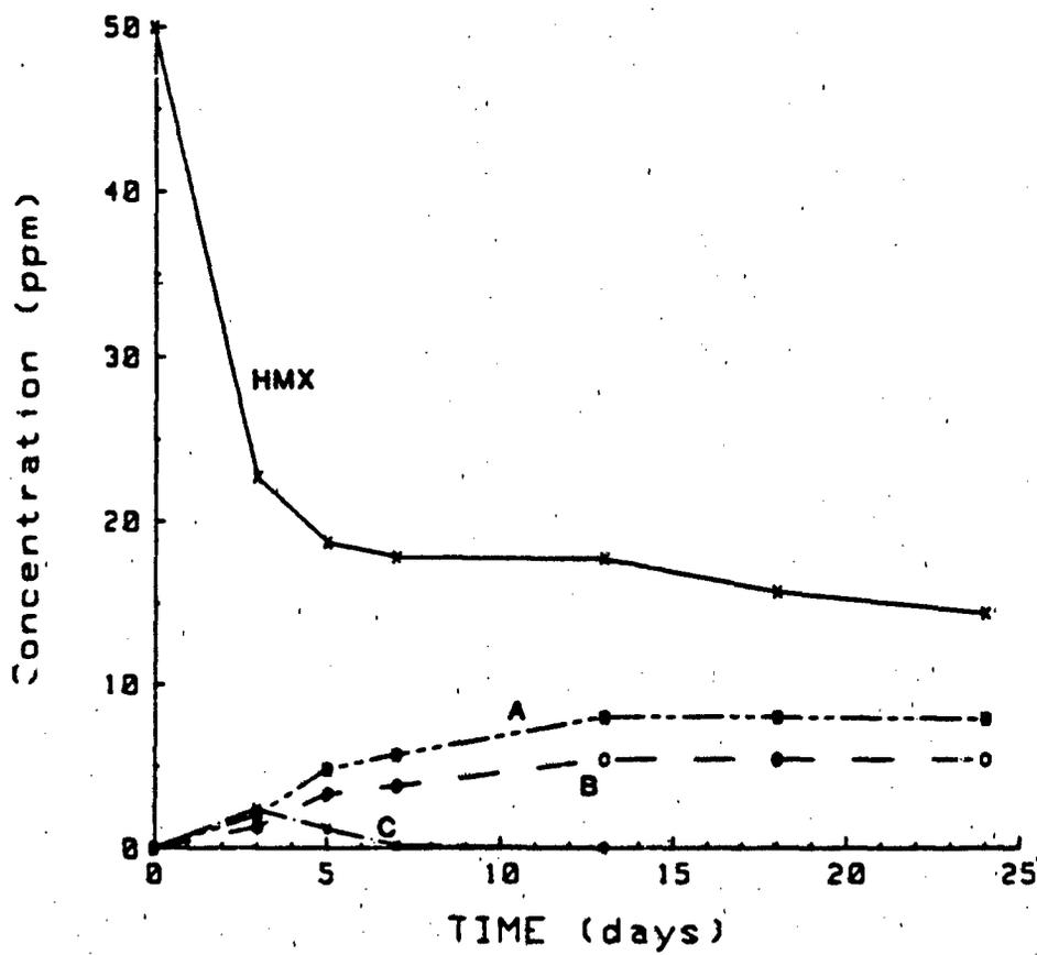
Figure 7. Kinetics of disappearance of HMX and production of intermediates during anaerobic incubation.
