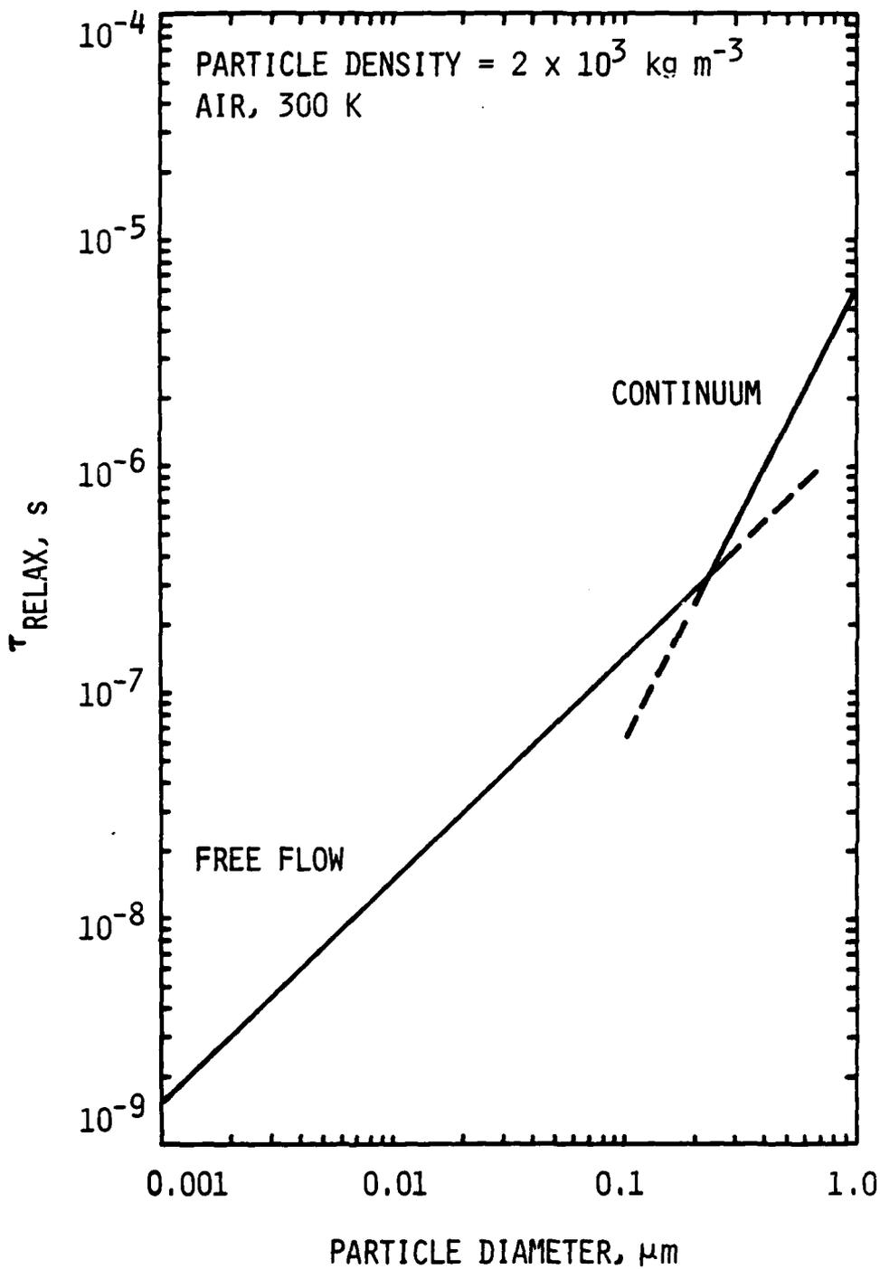
Figure A-1. Characteristic Relaxation Time for Particles in Brownian Motion.
