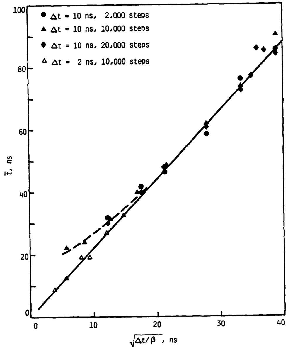
Figure A-10. Correlation Between the Mean Time Between Signal Extrema and the Particle Relaxation Time,  $\beta^{-1}$ .
