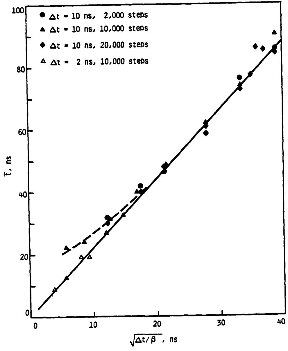
Figure 4. Correlation Between the Mean Time Between Signal Extrema and the Particle Relaxation Time,  $\beta^{-1}$ .
