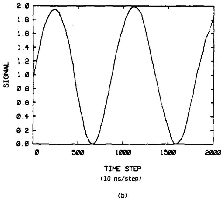
Figure A-7. Simulated Brownian Motion Signals for a 0.1 μm Diameter Particle with Fluid Velocity Component  $\bar{v}_z$  Superimposed
