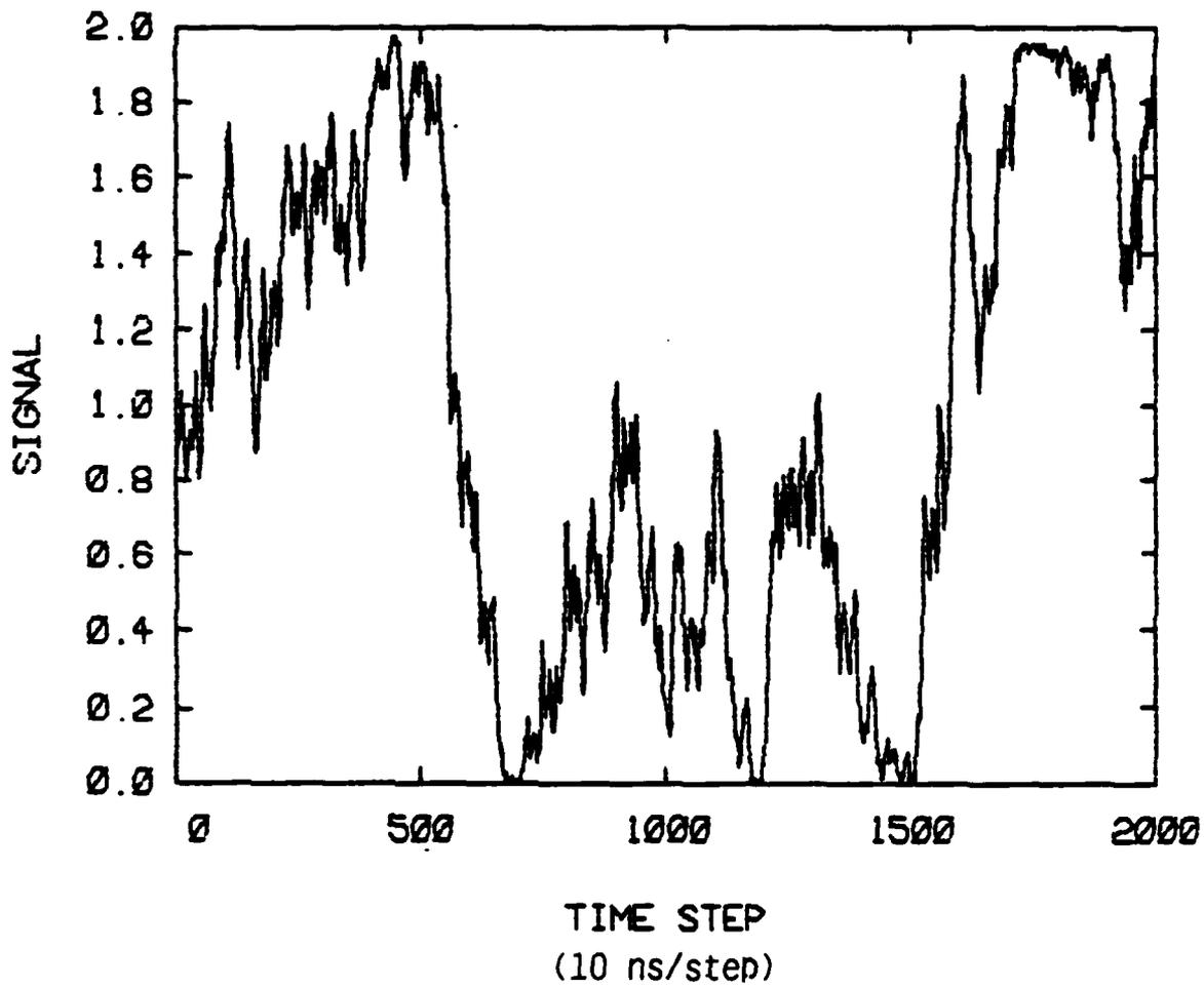
Figure A-8. Simulated Brownian Motion Signal for a  $0.01 \mu\text{m}$  Diameter Particle with  $\bar{v}_z = 0.3 \text{ m.s}^{-1}$  Superimposed.
